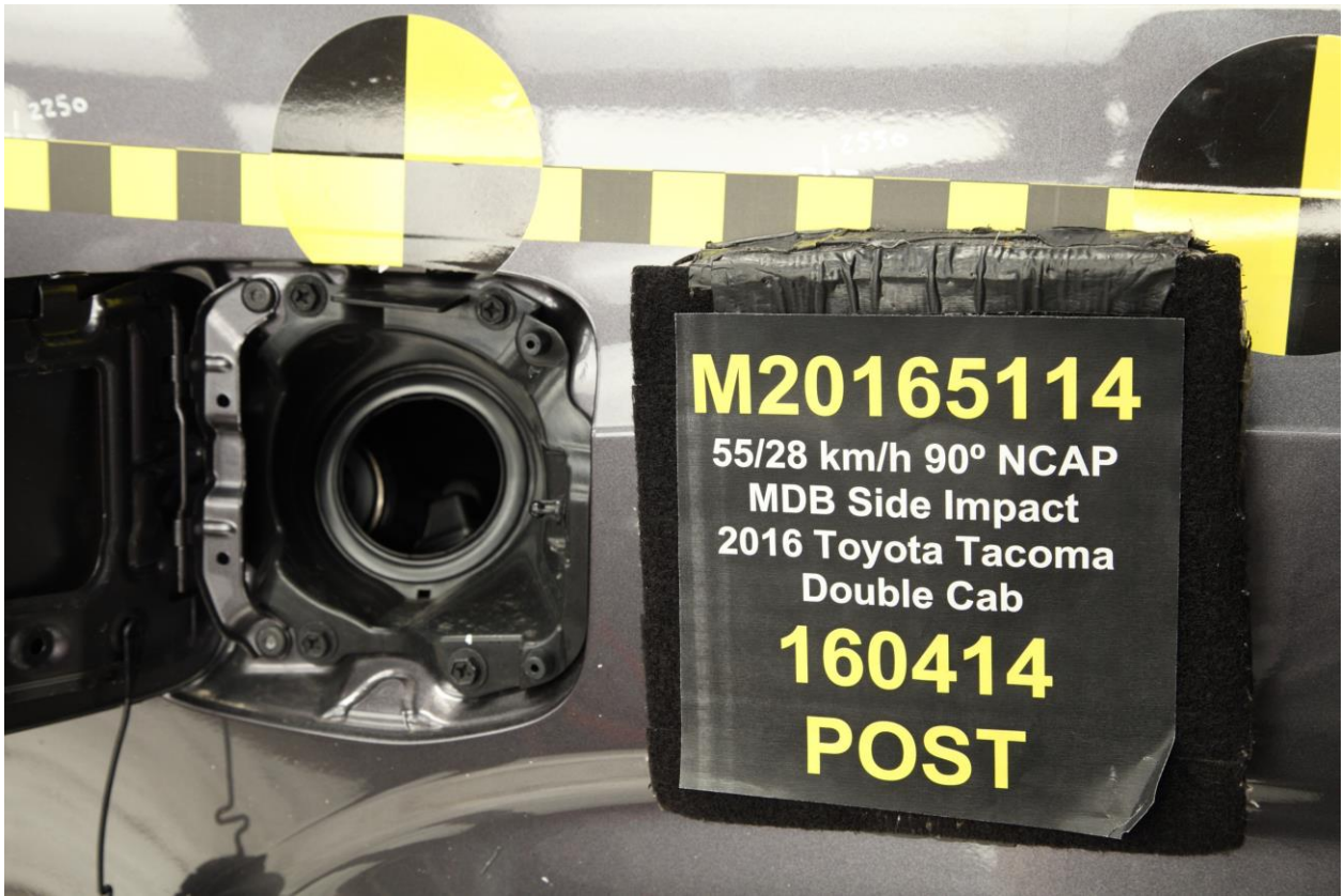
083a Post-Test View of Fuel Filler Cap or Fuel Filler Neck
