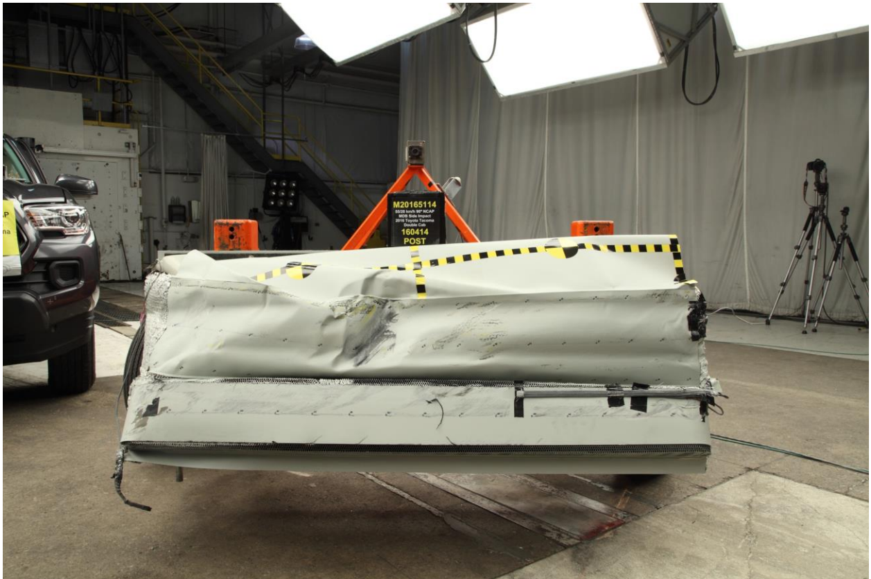
085 Post-Test Front View of MDB Impactor Face
