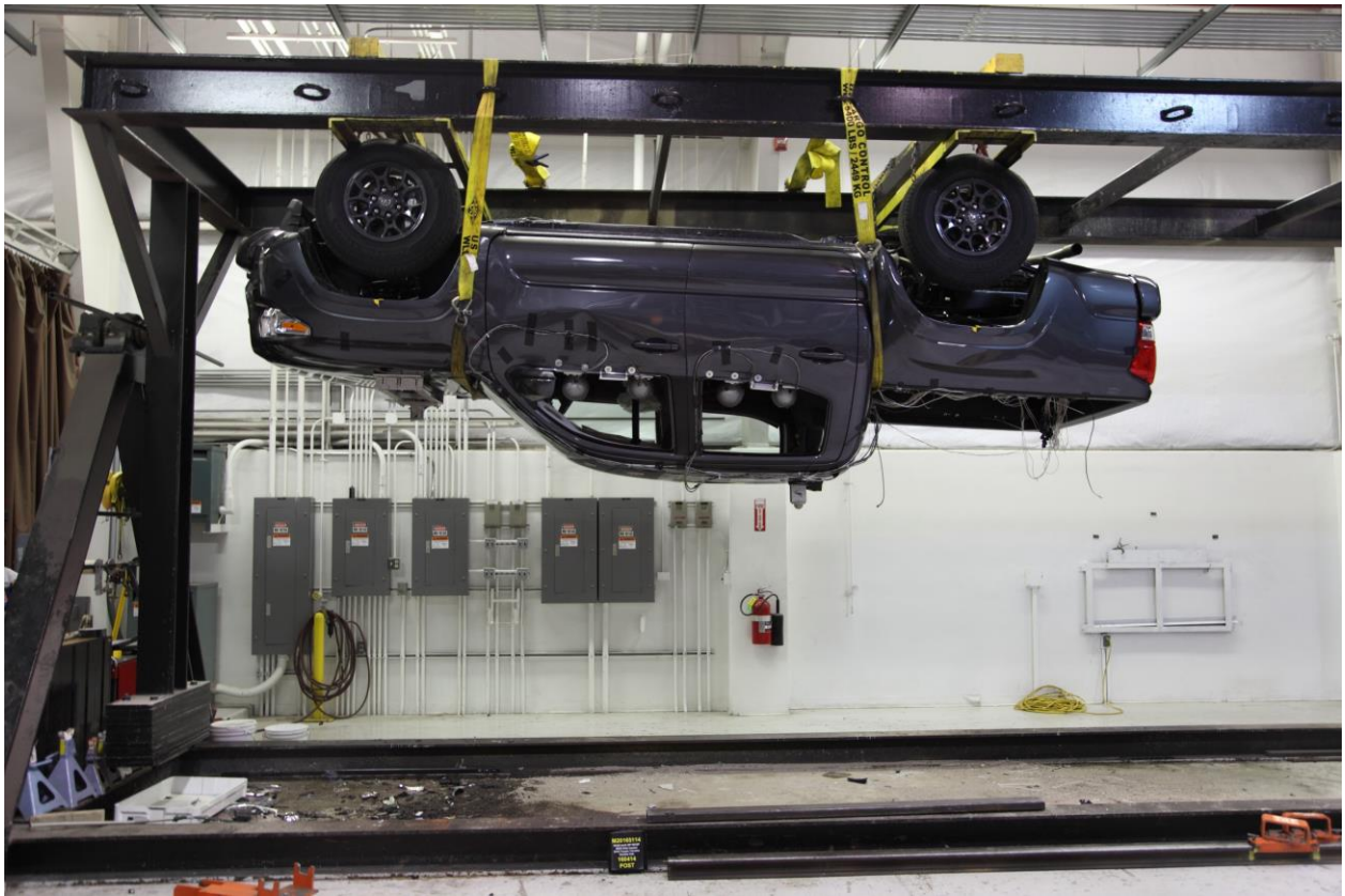
098 FMVSS No. 301 Static Rollover 180 Degrees
