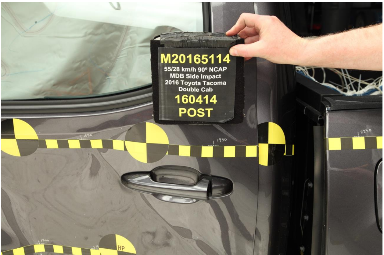
024 Post-Test Left Rear Door Latch Close-Up
