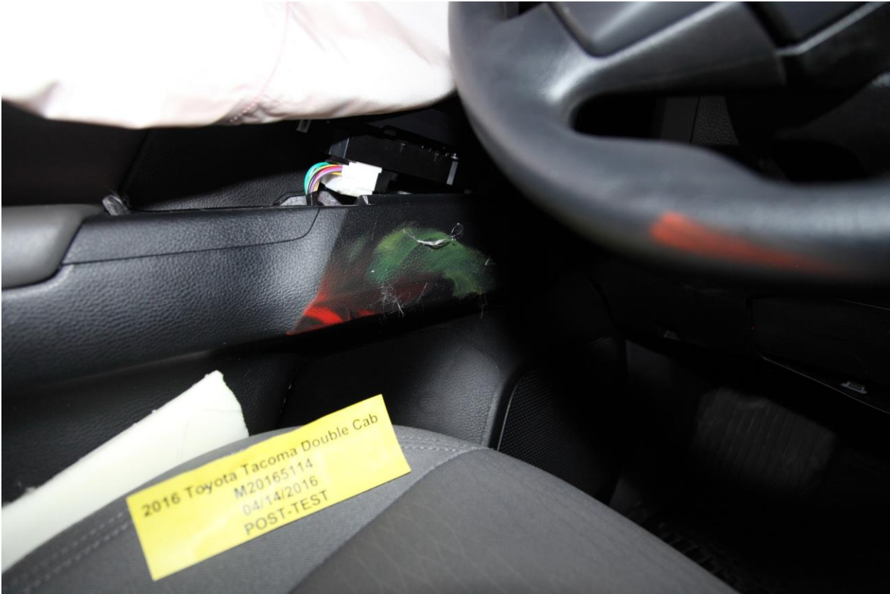
054 Post-Test Driver Dummy Close-Up Knee Contact View
