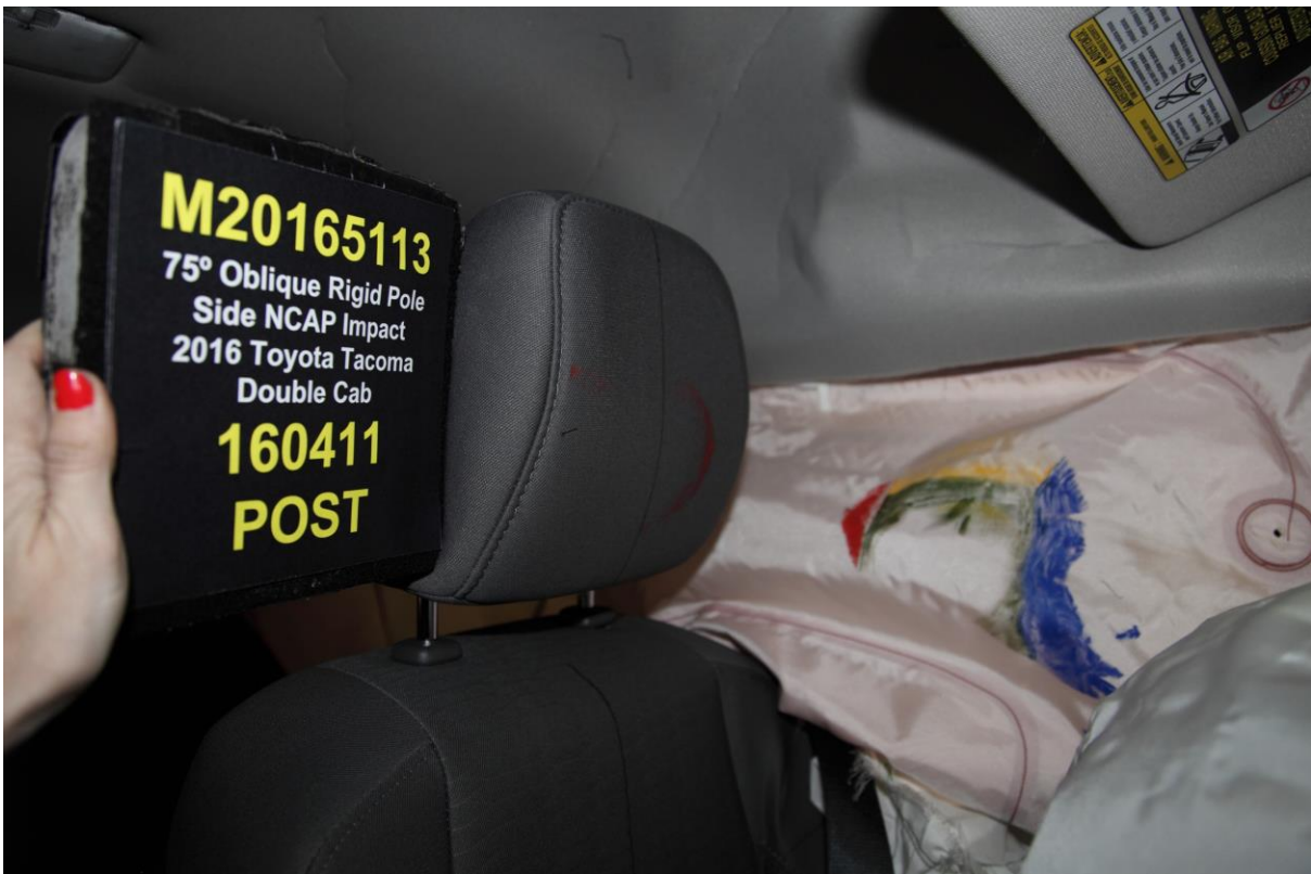
046 Post-Test Dummy Close-Up Head Contact with Vehicle Interior View
