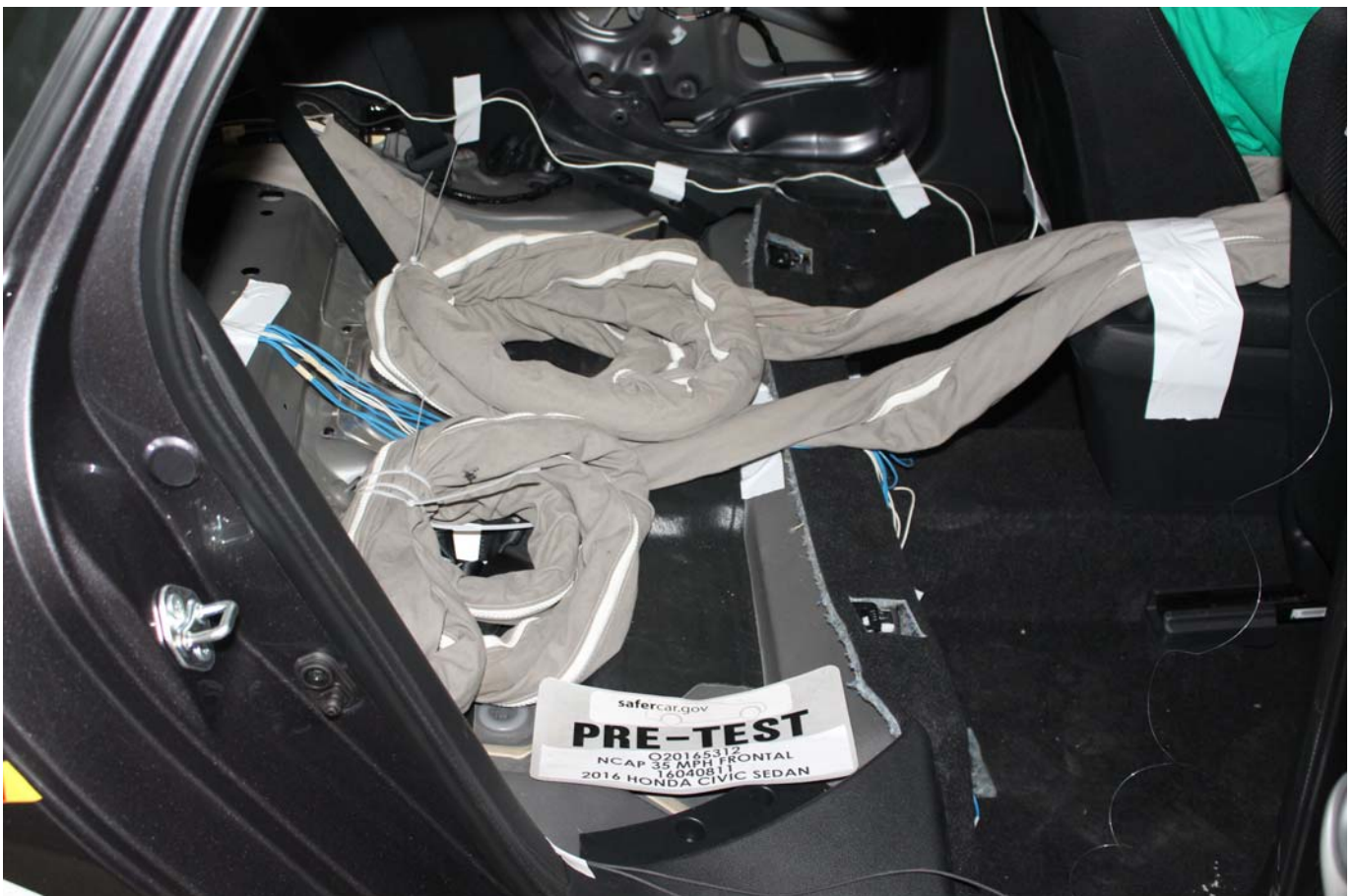
Photo No. 028 - Pre-Test Dummy Cable Routing
