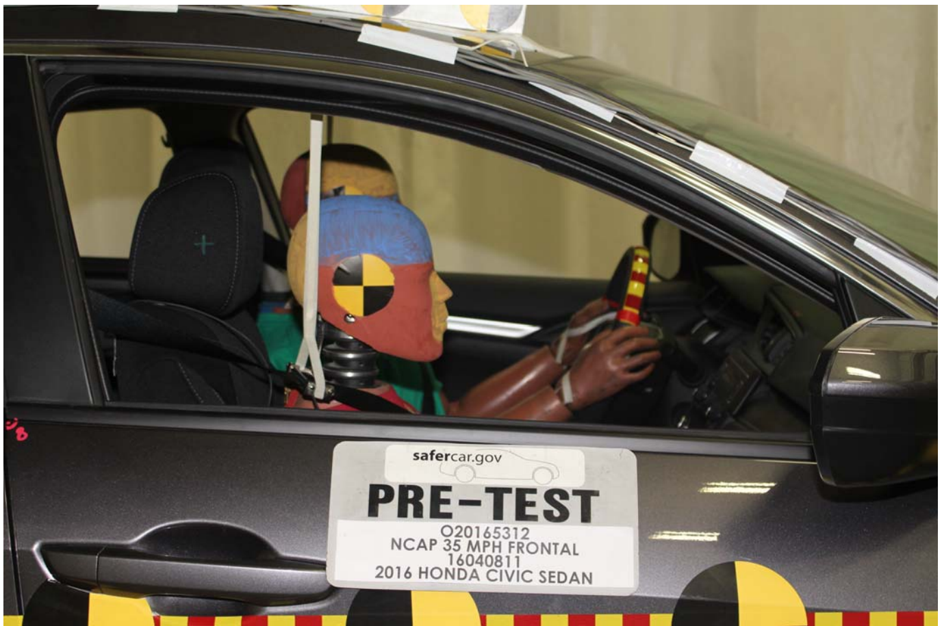
Photo No. 053 - Pre-Test Passenger Dummy Window View
