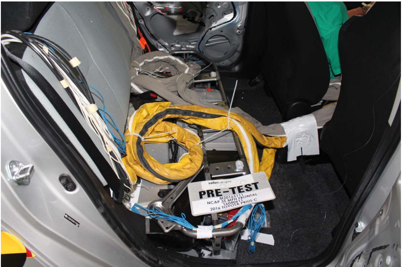
Photo No. 028 - Pre-Test Dummy Cable Routing
