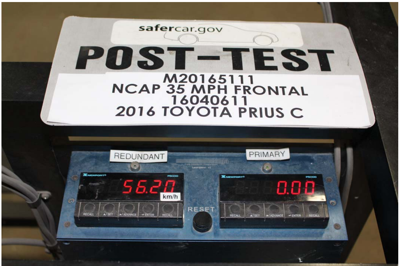
Photo No. 072 - Post-Test Speed Trap Read-Out
