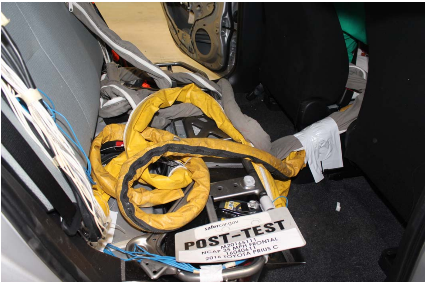
Photo No. 029 - Post-Test Dummy Cable Routing
