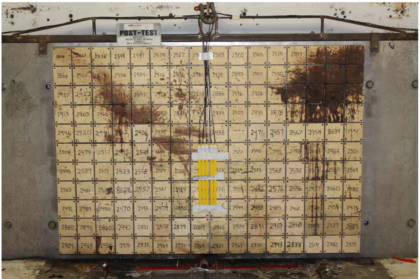
Photo No. 003 - Post-Test Load Cell Wall
