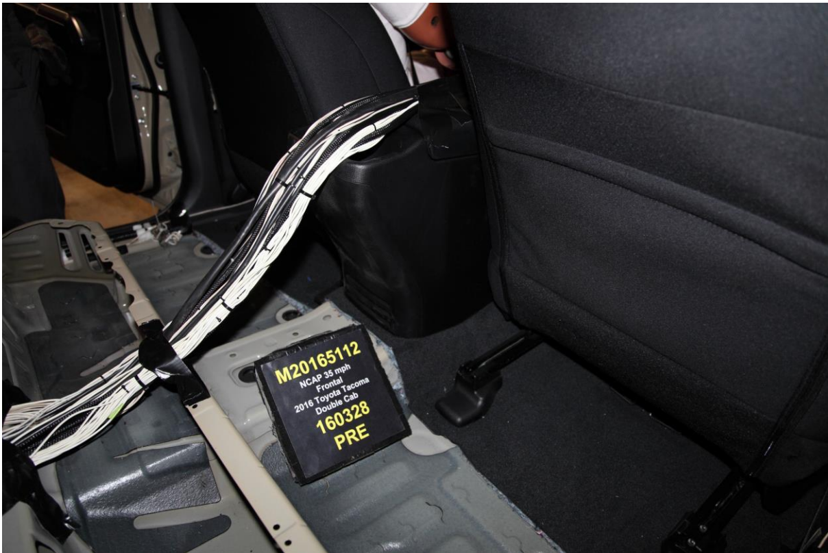
028 Pre-Test Dummy Cable Routing
