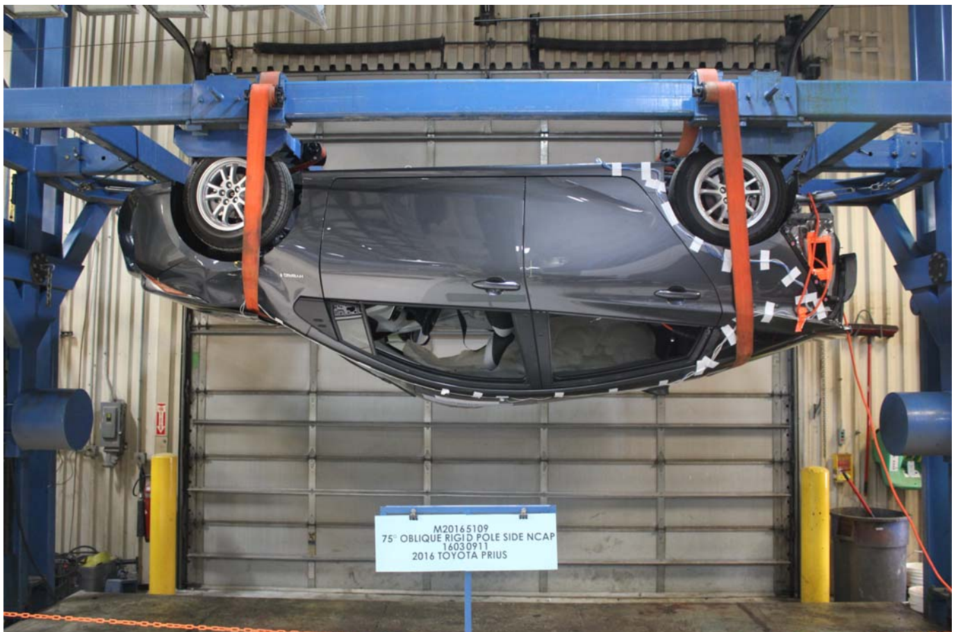
Photo No. 065 - FMVSS No. 301 Static Rollover 180 Degrees
