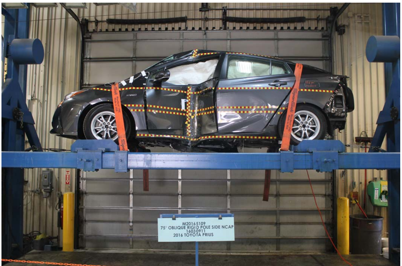
Photo No. 067 - FMVSS No. 301 Static Rollover 360 Degrees
