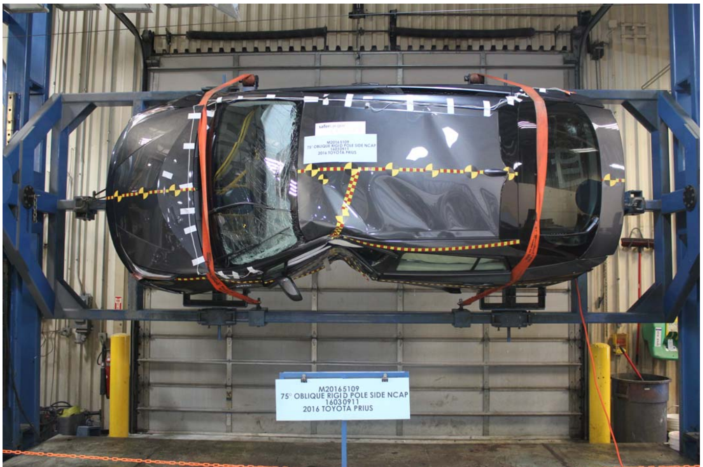
Photo No. 064 - FMVSS No. 301 Static Rollover 90 Degrees
