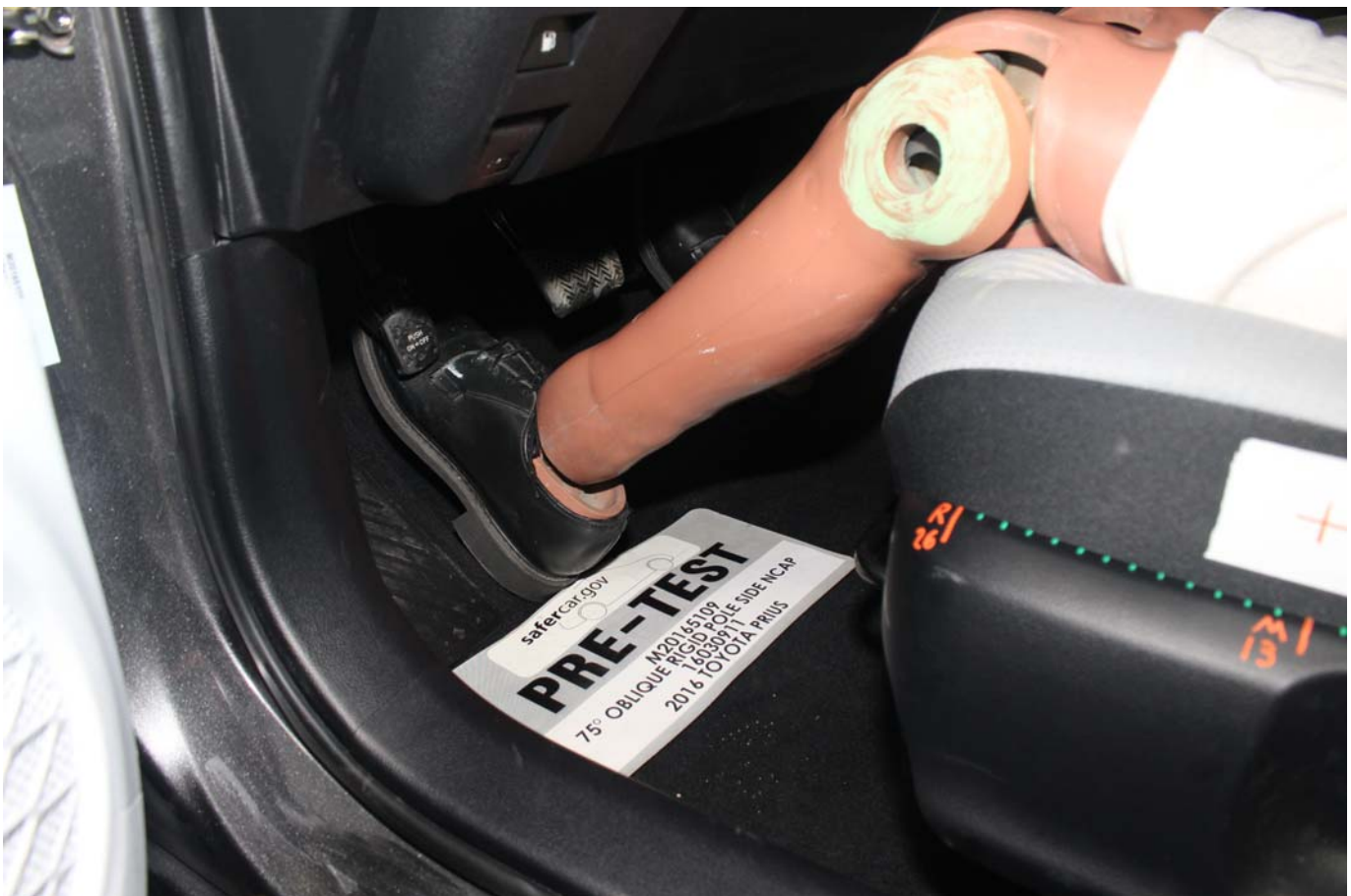
Photo No. 032 - Pre-Test Placement of Dummy's Feet
