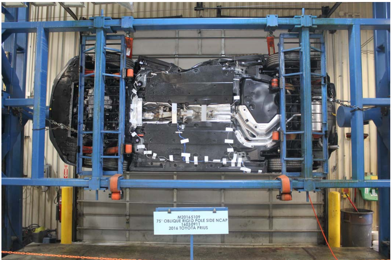
Photo No. 066 - FMVSS No. 301 Static Rollover 270 Degrees
