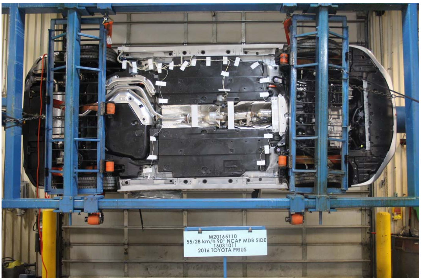
Photo No. 097 - FMVSS No. 301 Static Rollover 90 Degrees
