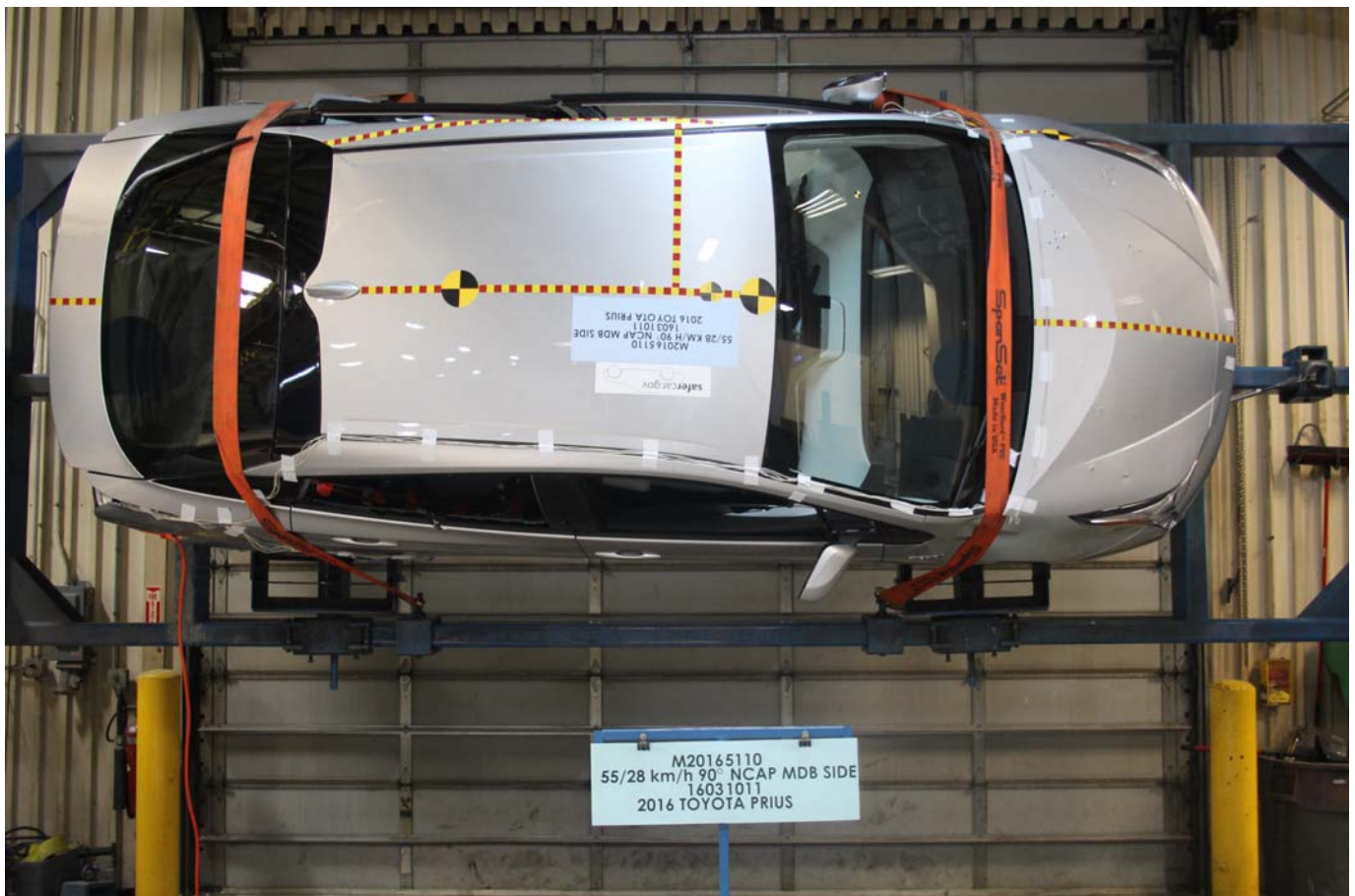
Photo No. 099 - FMVSS No. 301 Static Rollover 270 Degrees
