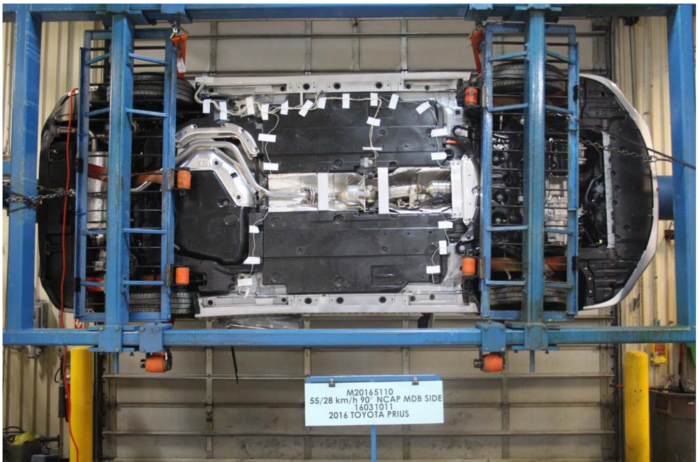
Photo No. 027 - FMVSS No. 305 Static Rollover at 90°
