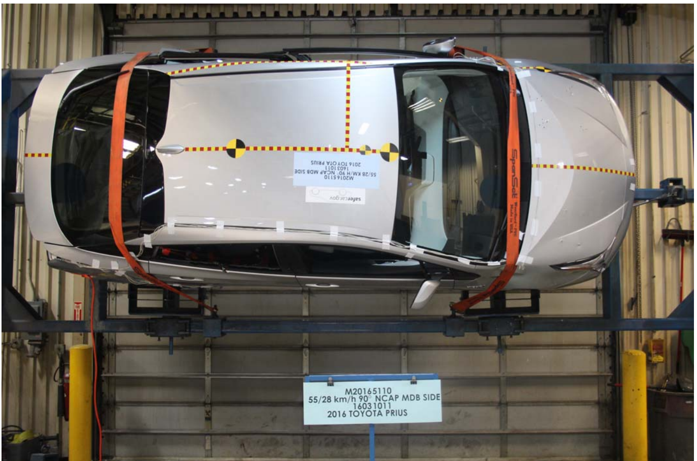
Photo No. 029 - FMVSS No. 305 Static Rollover at 270°
