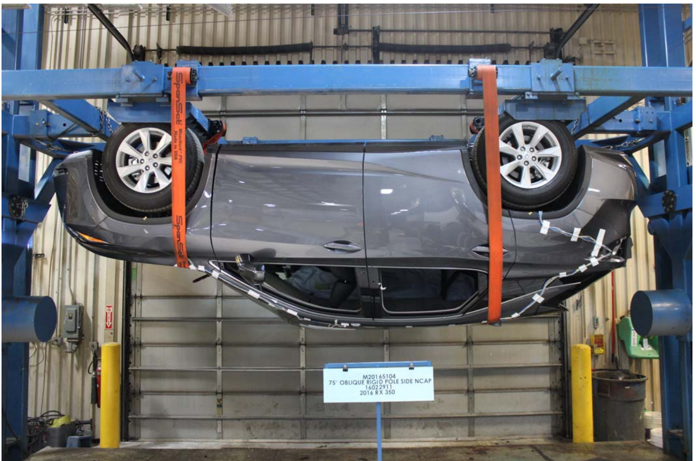
Photo No. 065 - FMVSS No. 301 Static Rollover 180 Degrees
