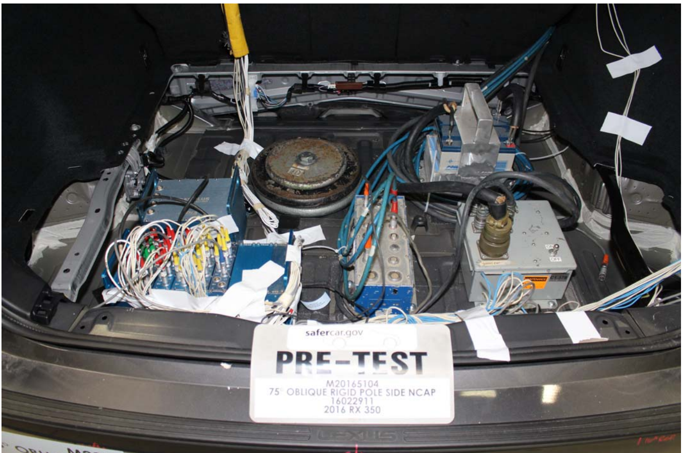
Photo No. 061 - Pre-Test Ballast View
