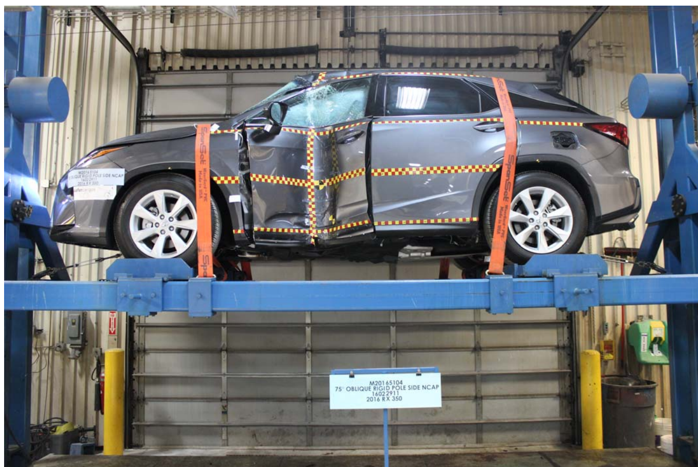
Photo No. 063 - FMVSS No. 301 Static Rollover 0 Degrees
