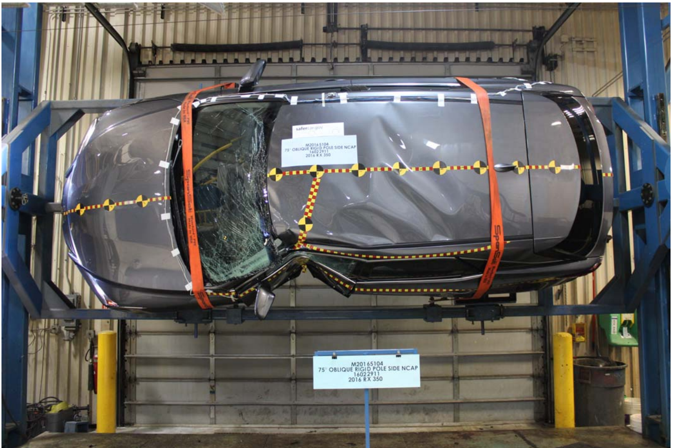
Photo No. 064 - FMVSS No. 301 Static Rollover 90 Degrees
