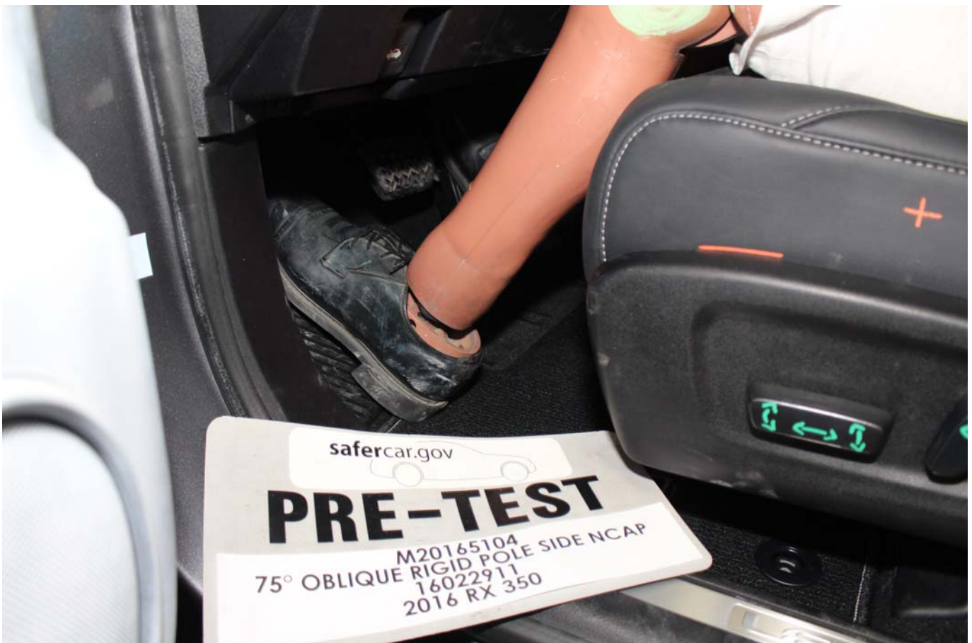
Photo No. 032 - Pre-Test Placement of Dummy's Feet
