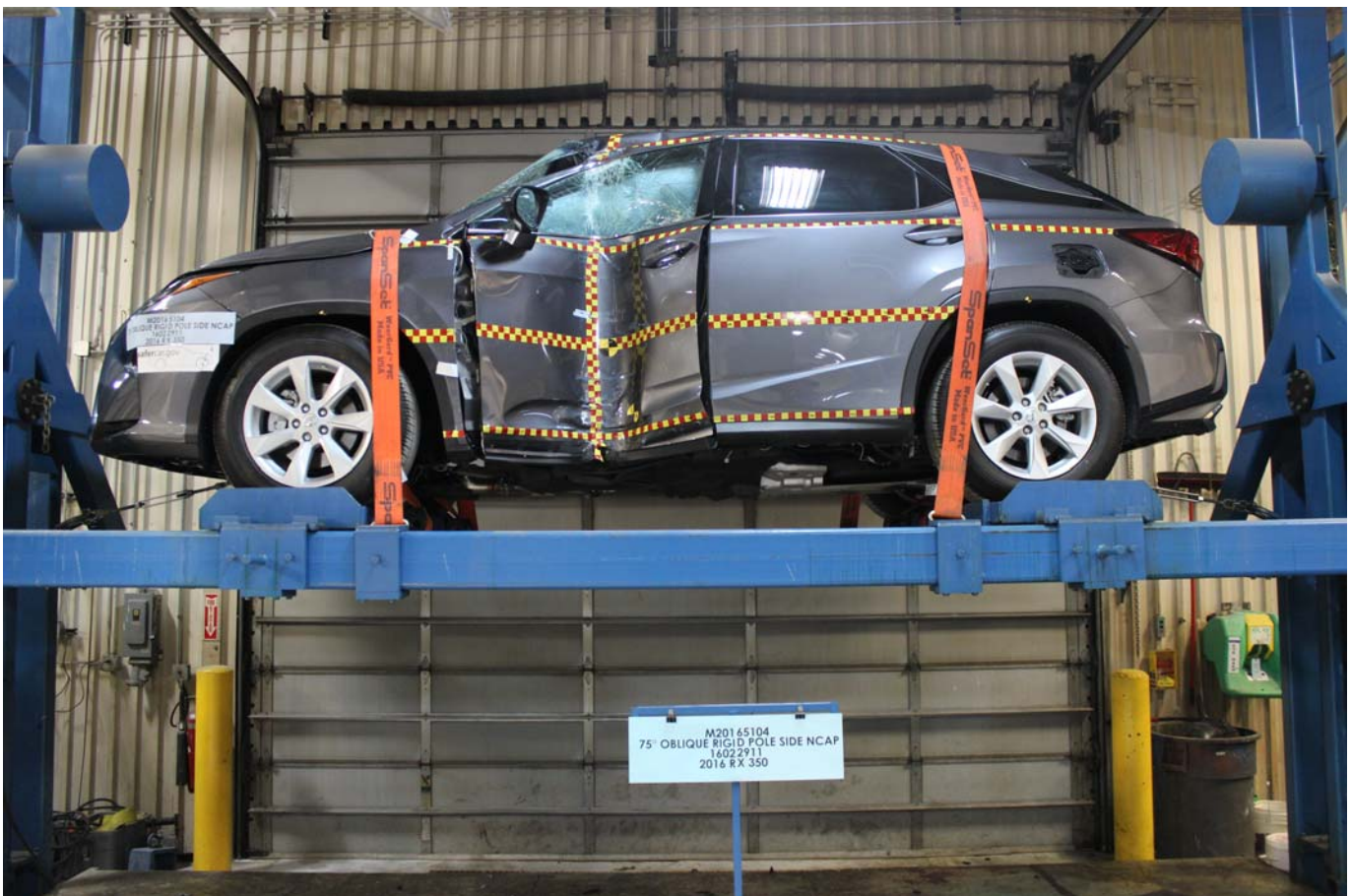
Photo No. 067 - FMVSS No. 301 Static Rollover 360 Degrees
