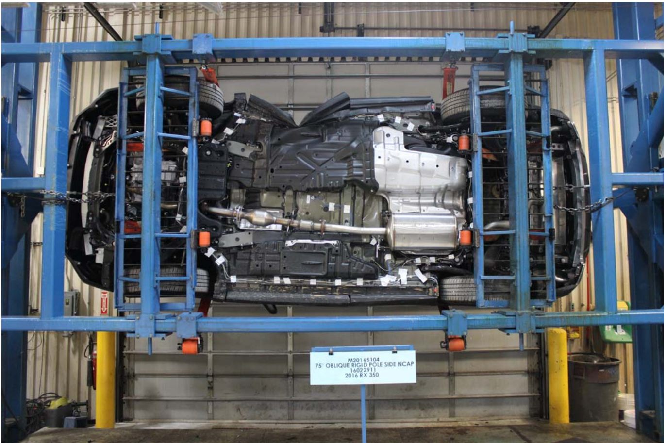
Photo No. 066 - FMVSS No. 301 Static Rollover 270 Degrees
