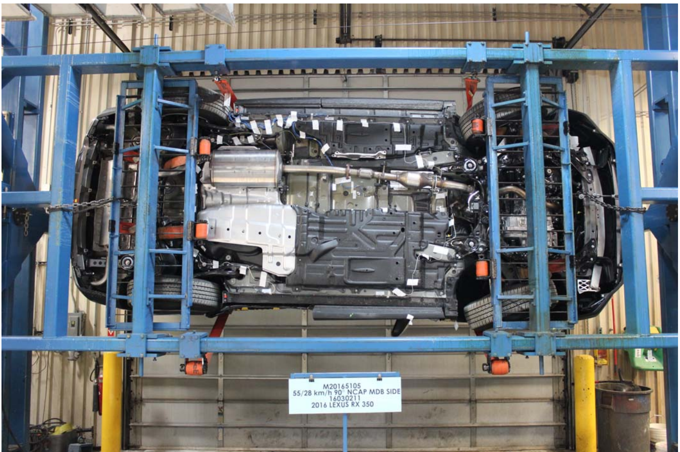
Photo No. 097 - FMVSS No. 301 Static Rollover 90 Degrees
