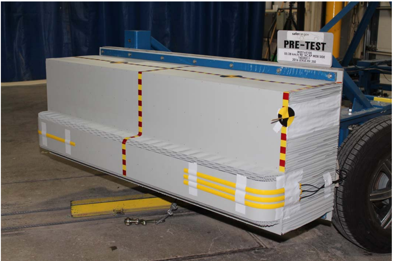
Photo No. 088 - Pre-Test Left Side View of MDB Impactor Face
