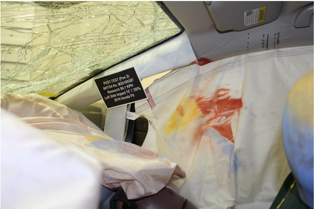
No. 119: Post-Test View of Passenger Head contact with Airbag - Curtain Note: Curtain Airbag did not fire during Impact Event
