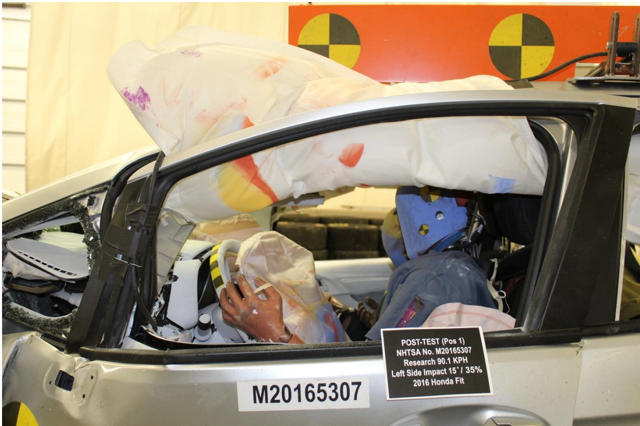
No. 078 Post-Test View of Driver Head Contact with Curtain Airbag
