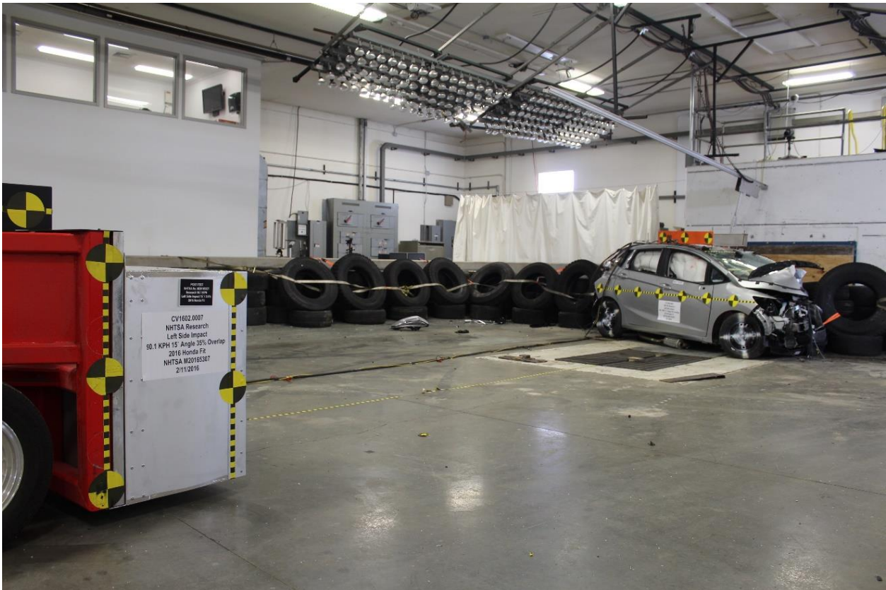
No. 184: Post-Test OMDB & Vehicle, Right Side
