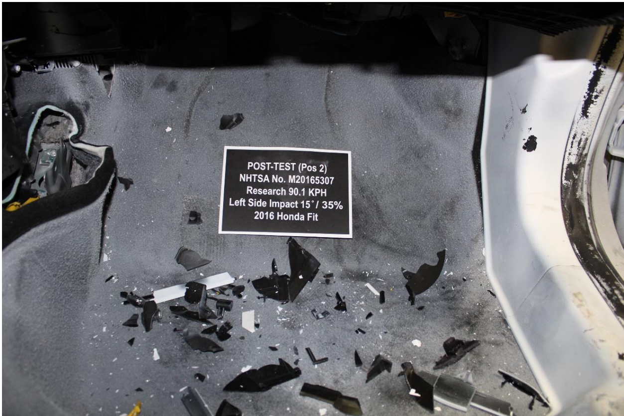
No. 091: Post-Test view of Passenger Floor pan at Mid seat level, w/carpet
