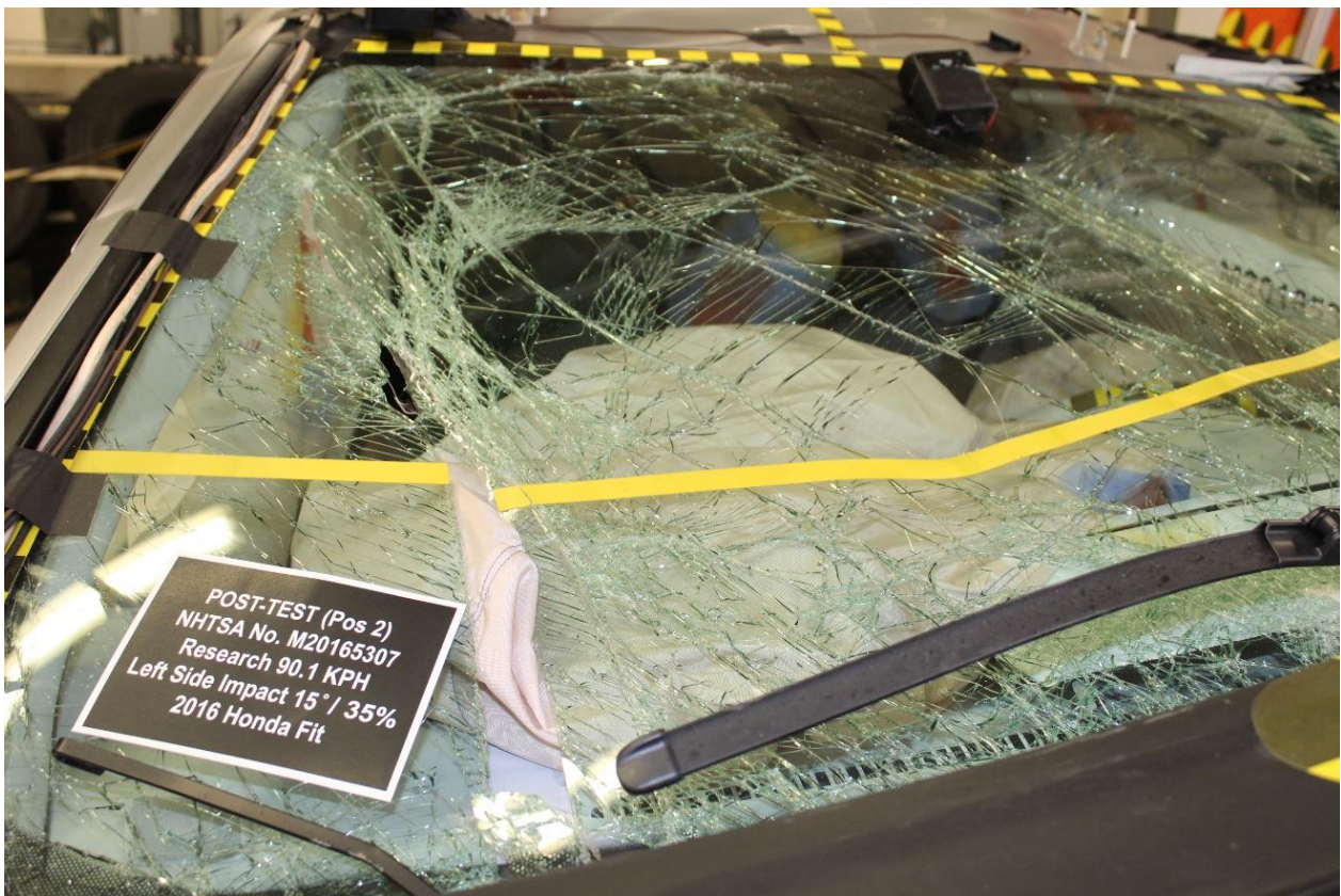
No. 166: Post-Test View of Windshield Separation
