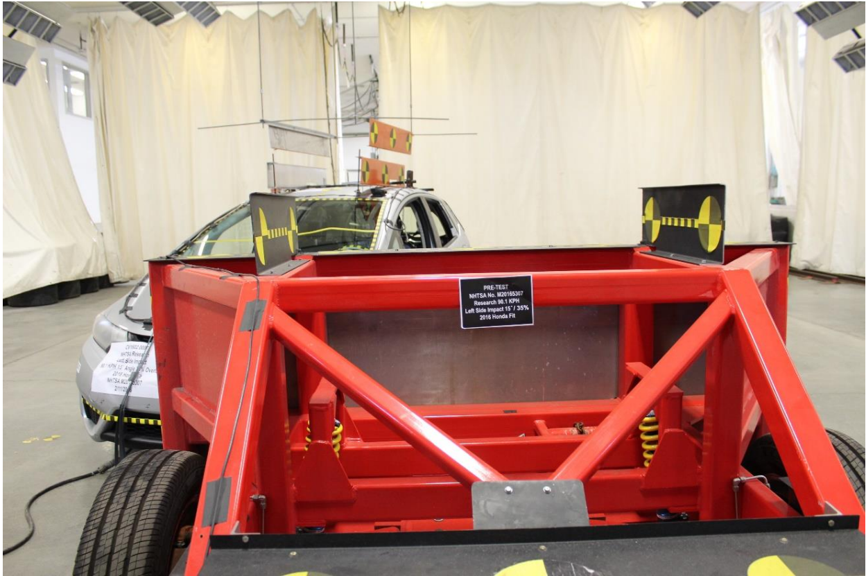
No. 189: Pre-Test OMDB & Vehicle, Rear View
