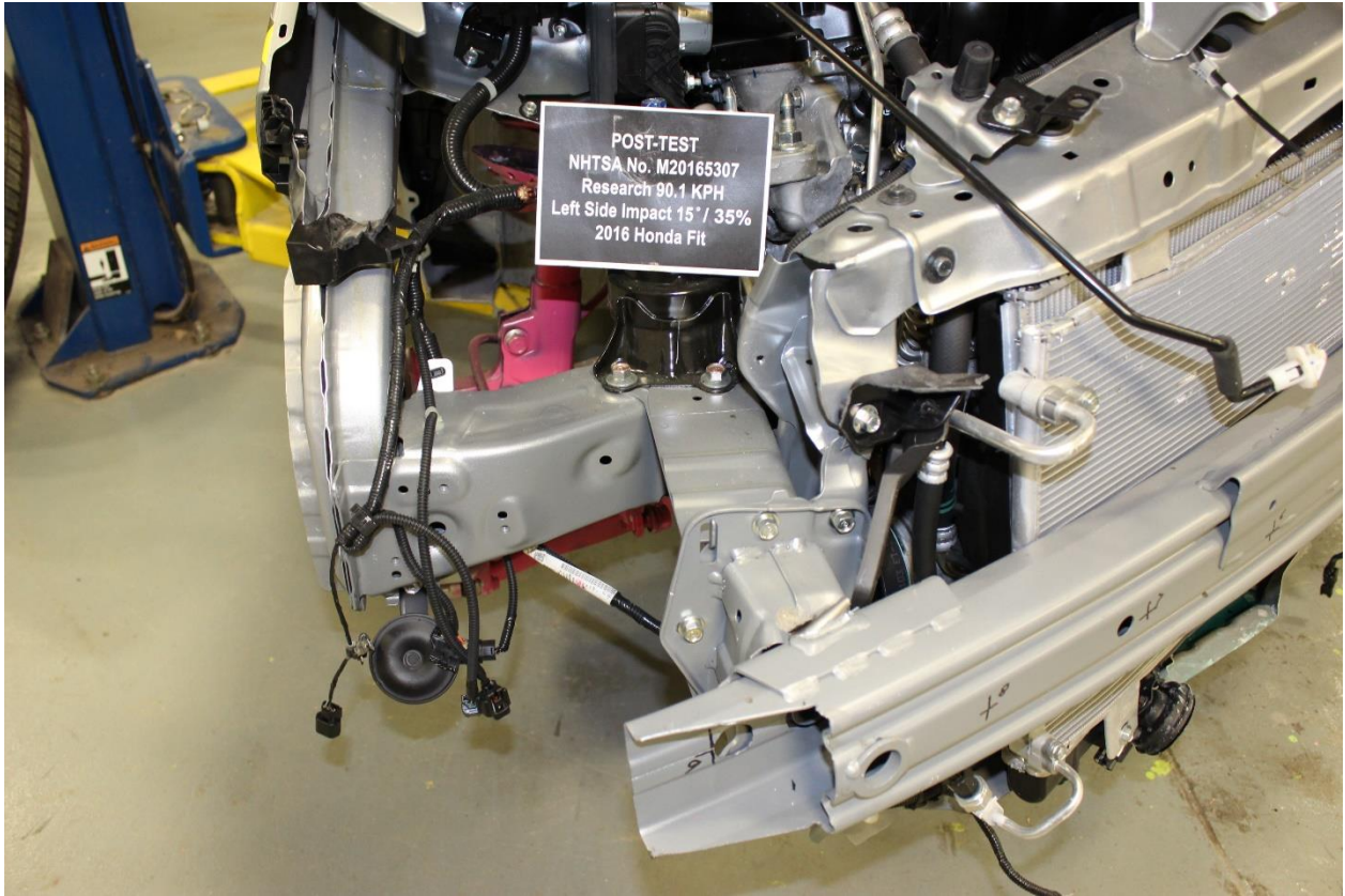
No. 157: Post-Test Looking Down at the Front Passenger Shotgun
