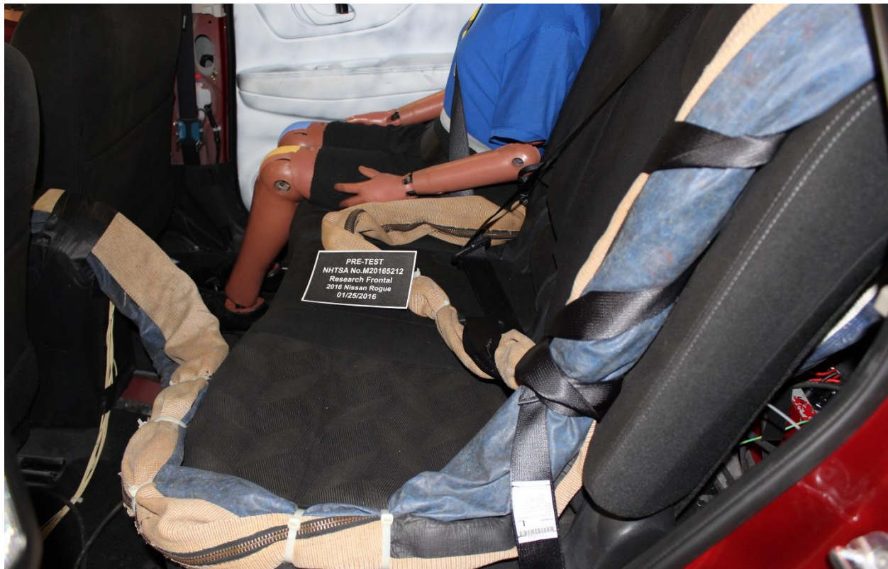
Figure A-27: Pre-Test Dummy Cable Routing
