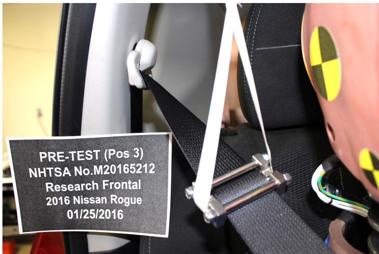
Figure A-87: Pre-Test View of Belt Anchorage for Rear Passenger Dummy
