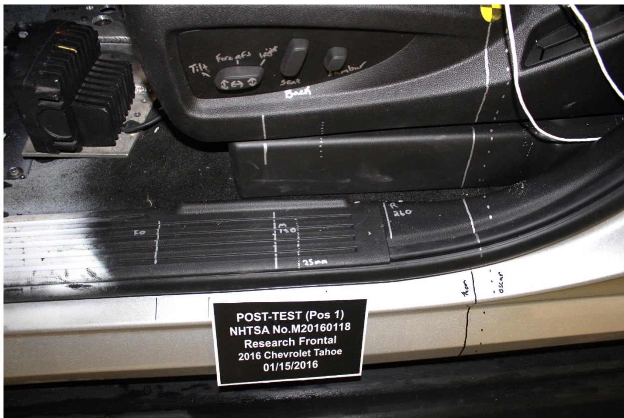
Figure A-36: Post-Test Driver's Seat Fore-Aft Markings
