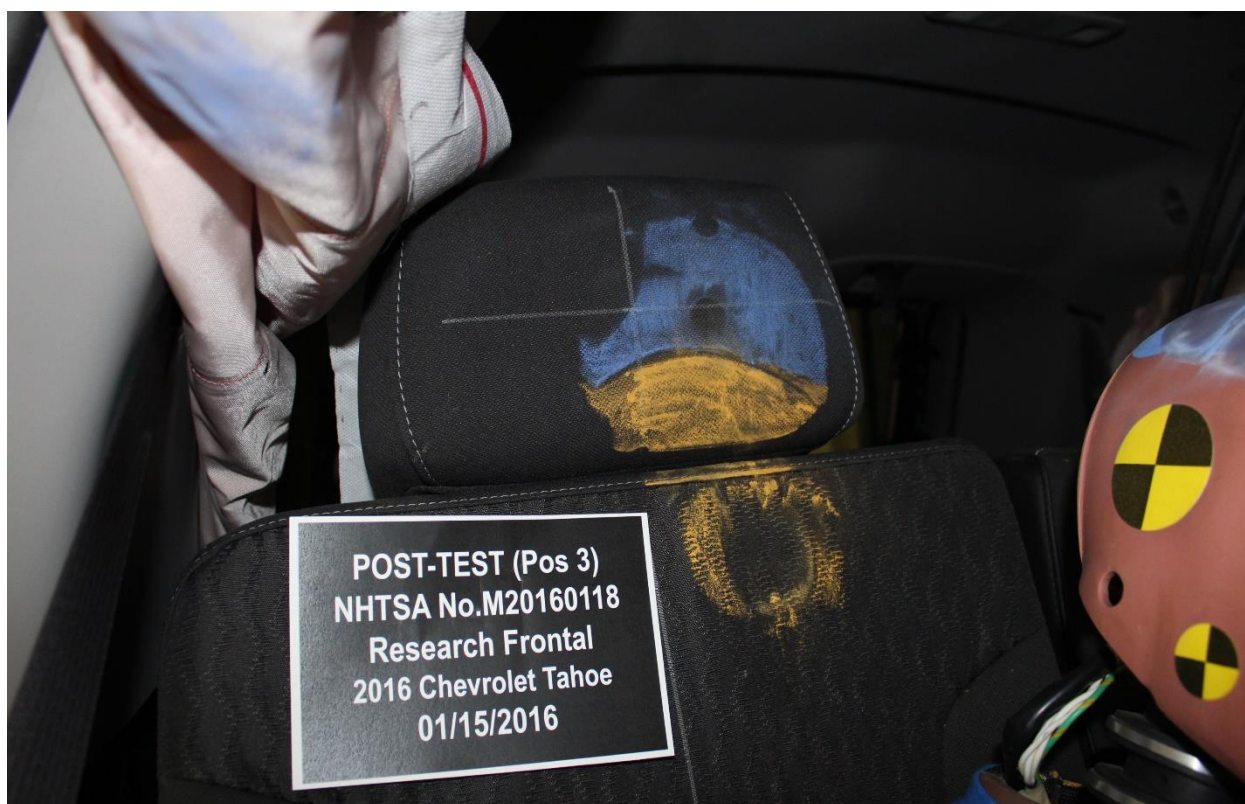
Figure A-97: Post-Test Rear Passenger dummy Contact with Headrest
