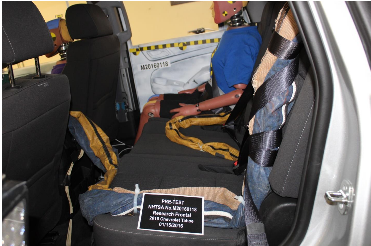
Figure A-27: Pre-Test Dummy Cable Routing
