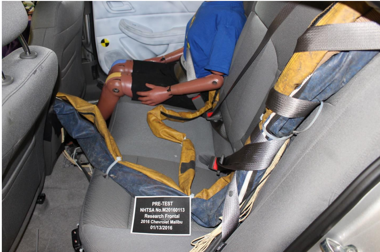
Figure A-27: Pre-Test Dummy Cable Routing
