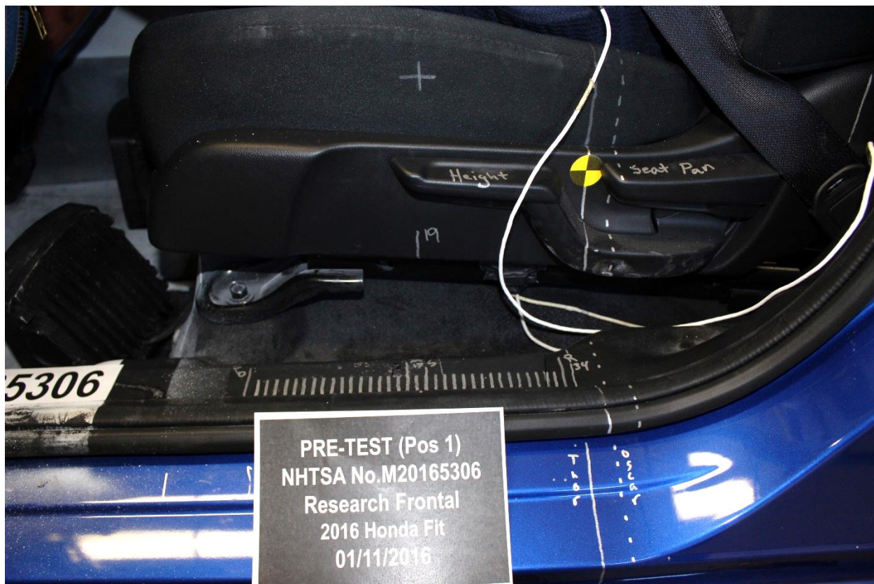
Figure A-35: Pre-Test Driver's Seat Fore-Aft Markings
