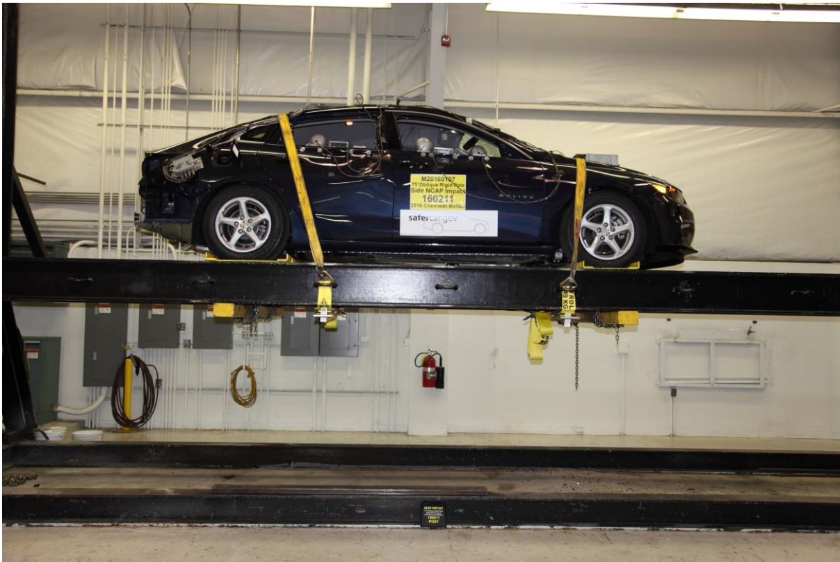
063 FMVSS No. 301 Static Rollover 0 Degrees
