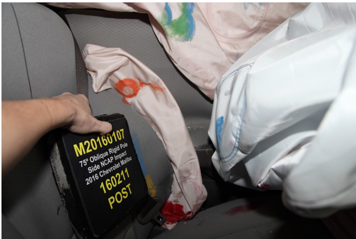
049 Post-Test Dummy Close-Up Torso Contact with Side Airbag View
