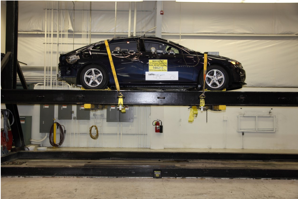
067 FMVSS No. 301 Static Rollover 360 Degrees
