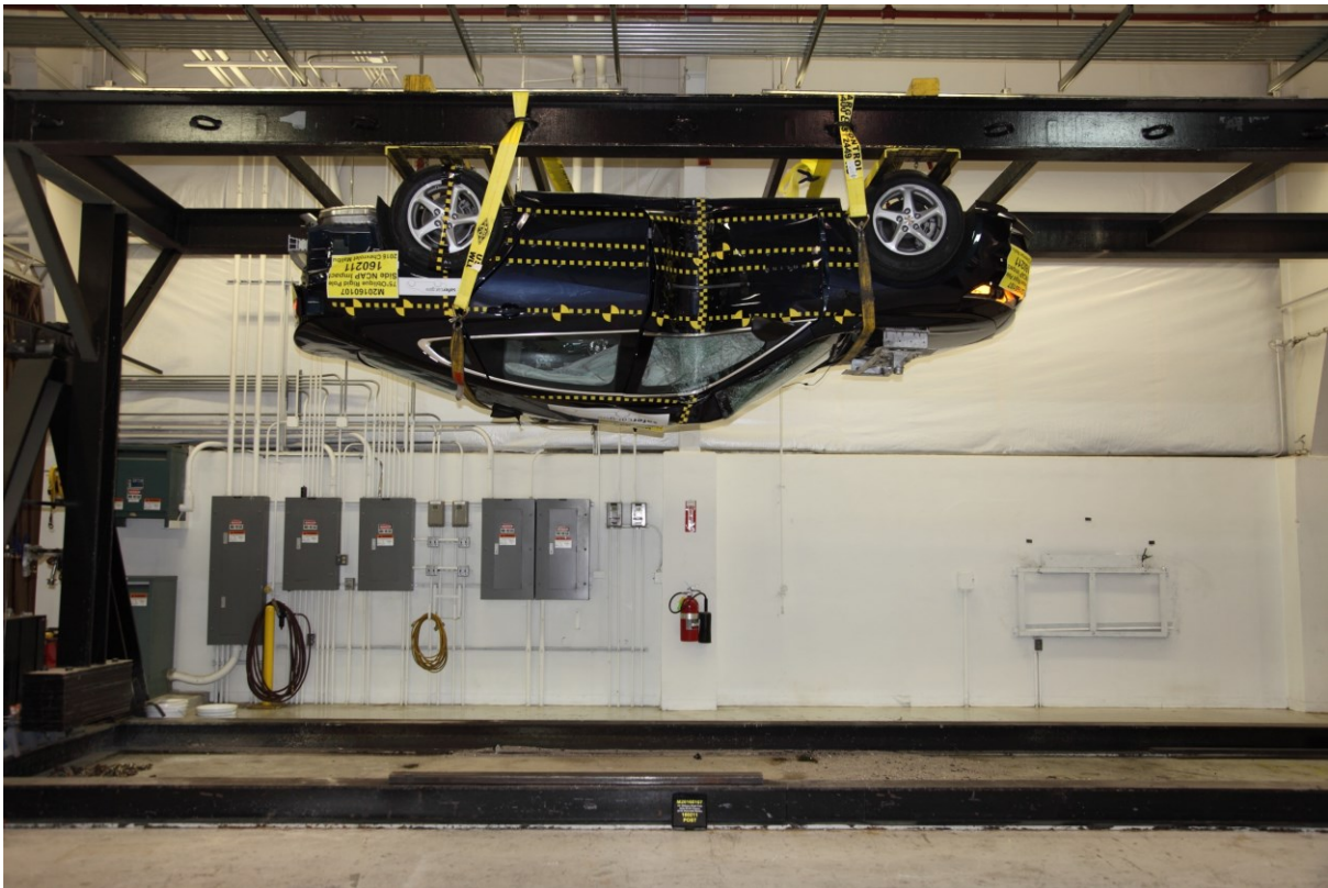
065 FMVSS No. 301 Static Rollover 180 Degrees
