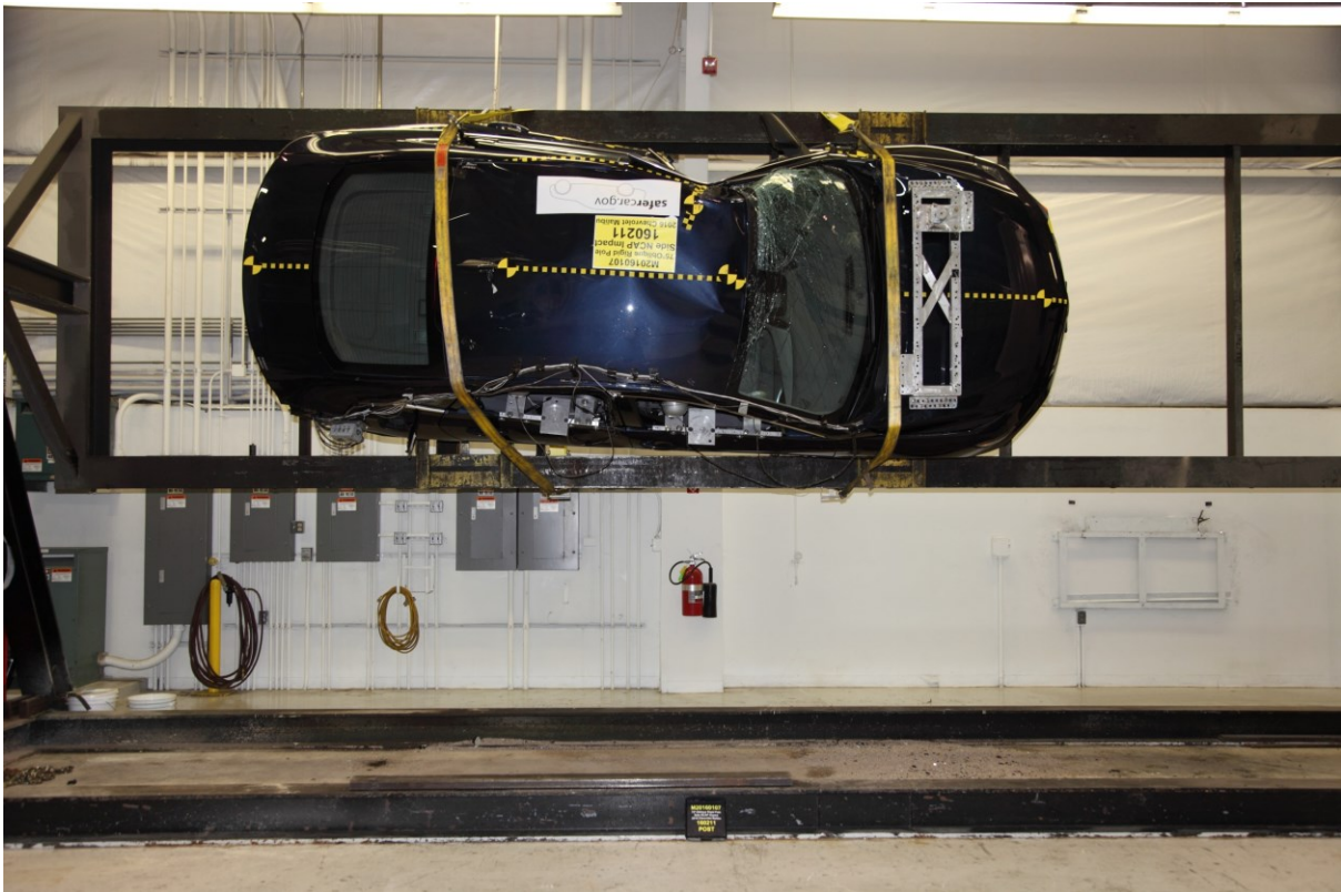
064 FMVSS No. 301 Static Rollover 90 Degrees
