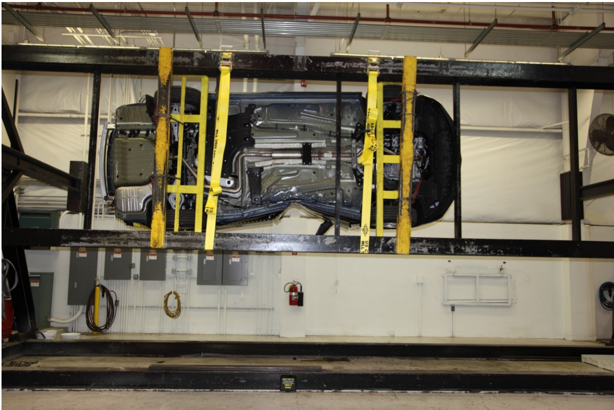
066 FMVSS No. 301 Static Rollover 270 Degrees
