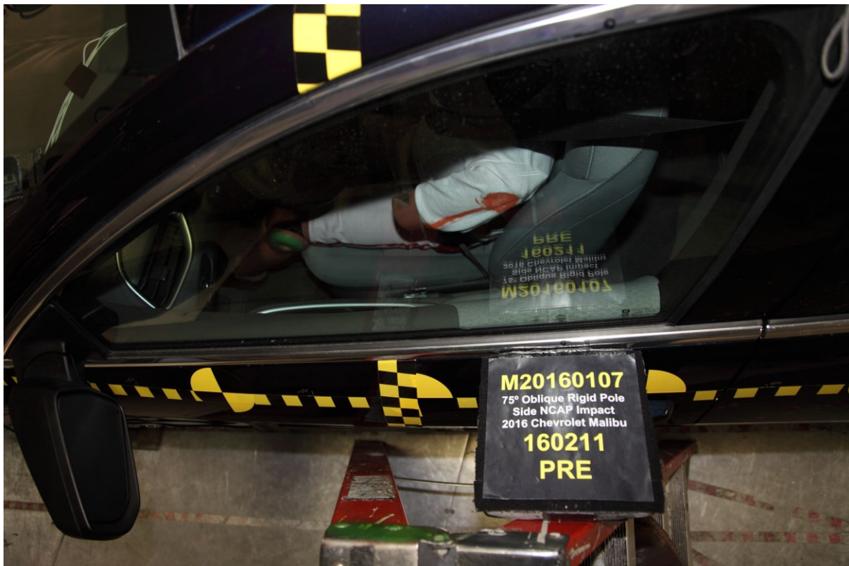
040 Pre-Test Dummy and Door Clearance View
