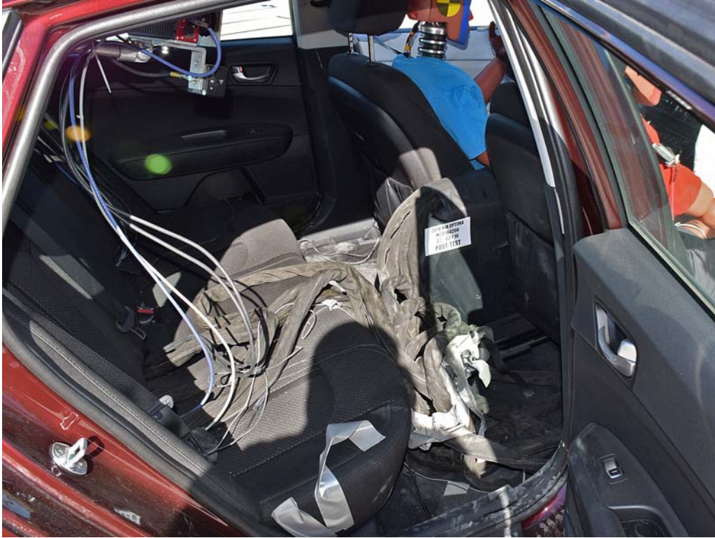
FIGURE 29. Post-Test Dummy Cable Routing
