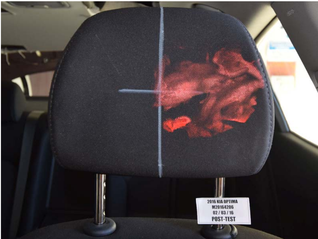
FIGURE 48. Post-Test Driver Dummy Contact with Headrest
