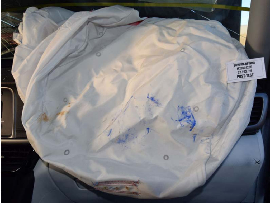
FIGURE 69a. Post-Test Passenger Dummy Contact with Airbag
