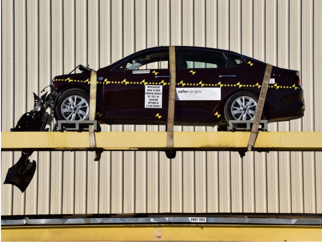
FIGURE 77. Vehicle at 360° on Static Rollover Device
