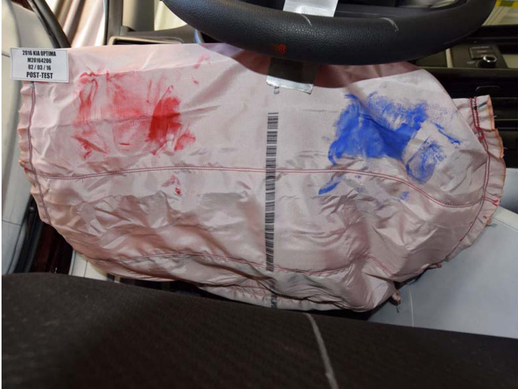
FIGURE 48a. Post-Test Driver Dummy Contact with Knee Airbag
