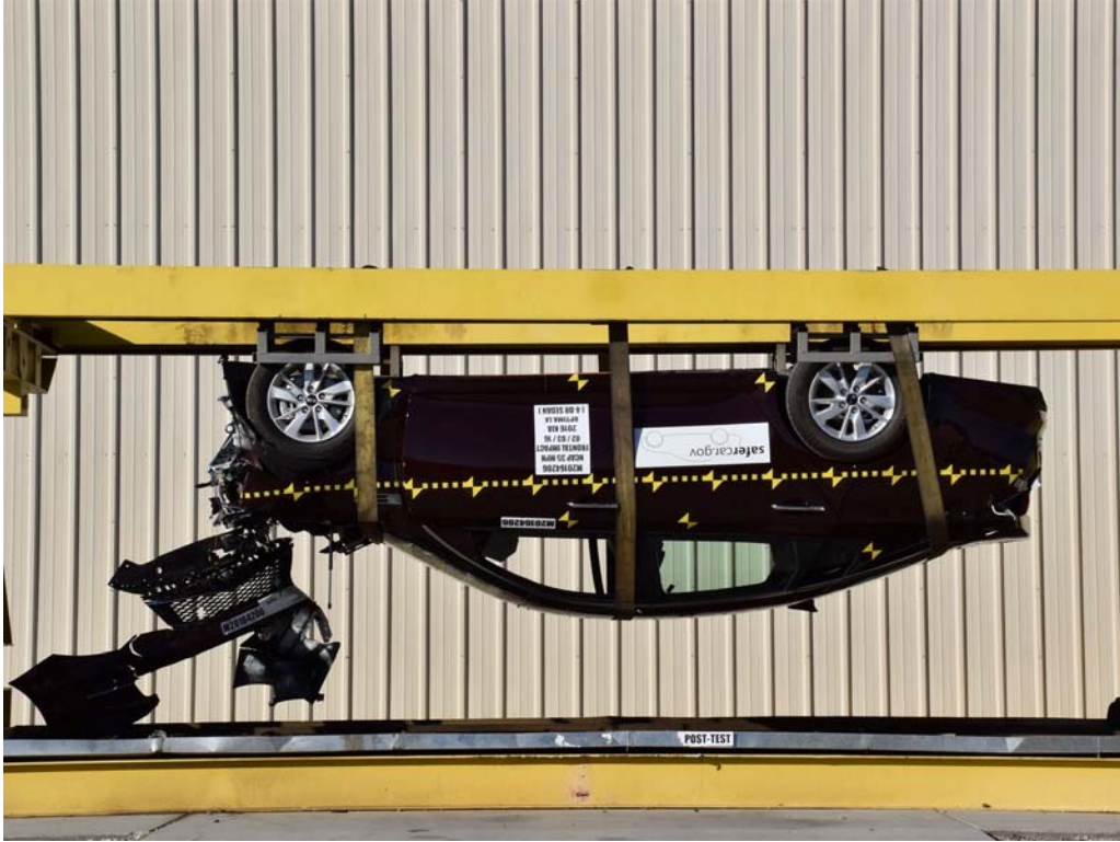
FIGURE 75. Vehicle at 180° on Static Rollover Device
