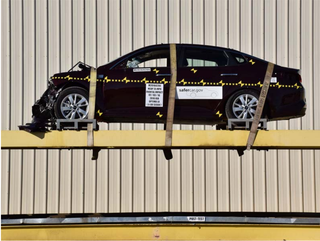
FIGURE 73. Vehicle at 0° on Static Rollover Device
