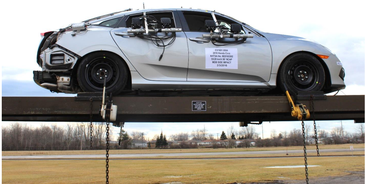
Figure A-100: FMVSS No. 301 Static Rollover 360 Degrees
