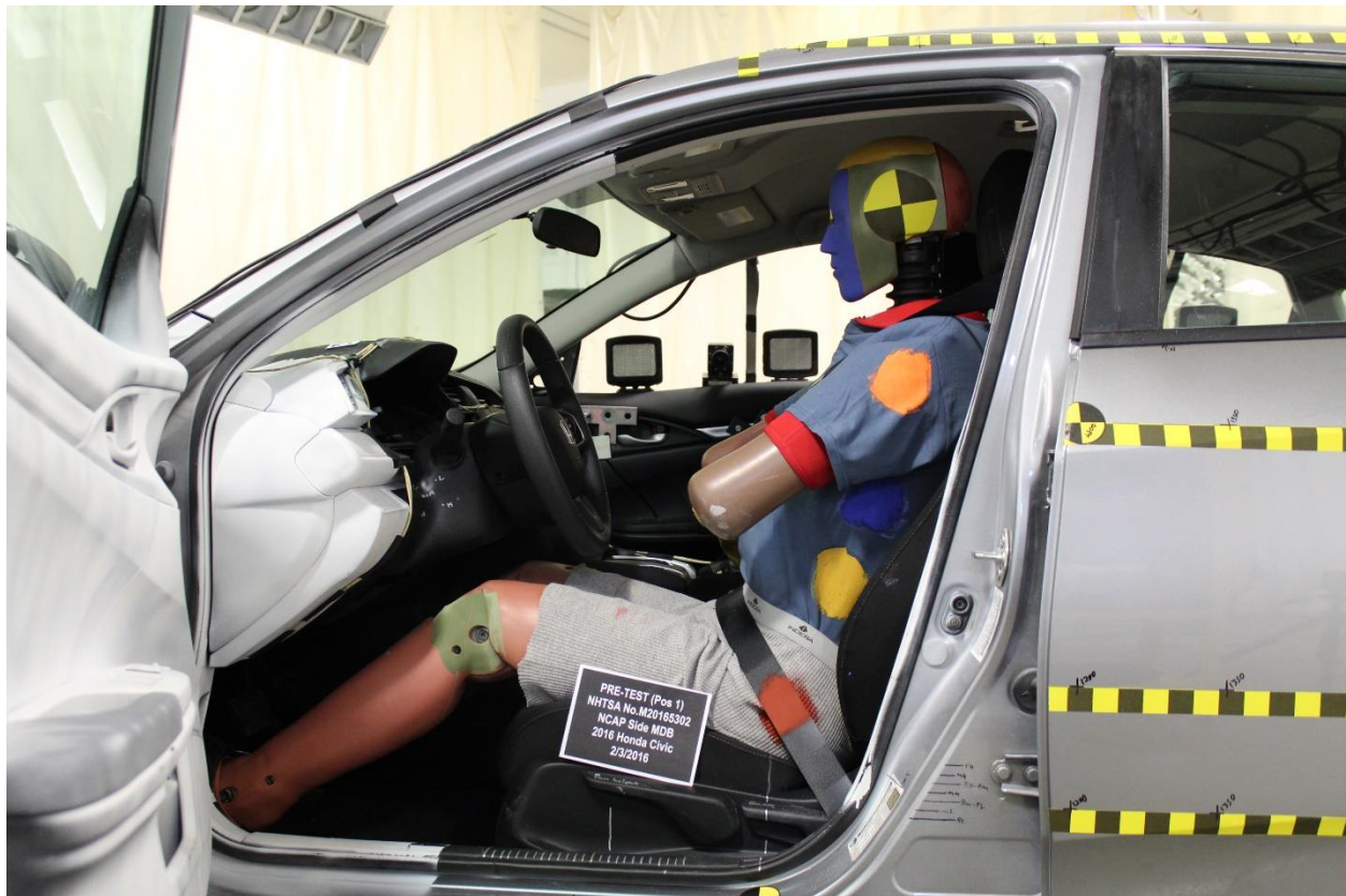
Figure A-27: Pre-Test Left Side View of Driver Dummy Showing Belt and Chalking
