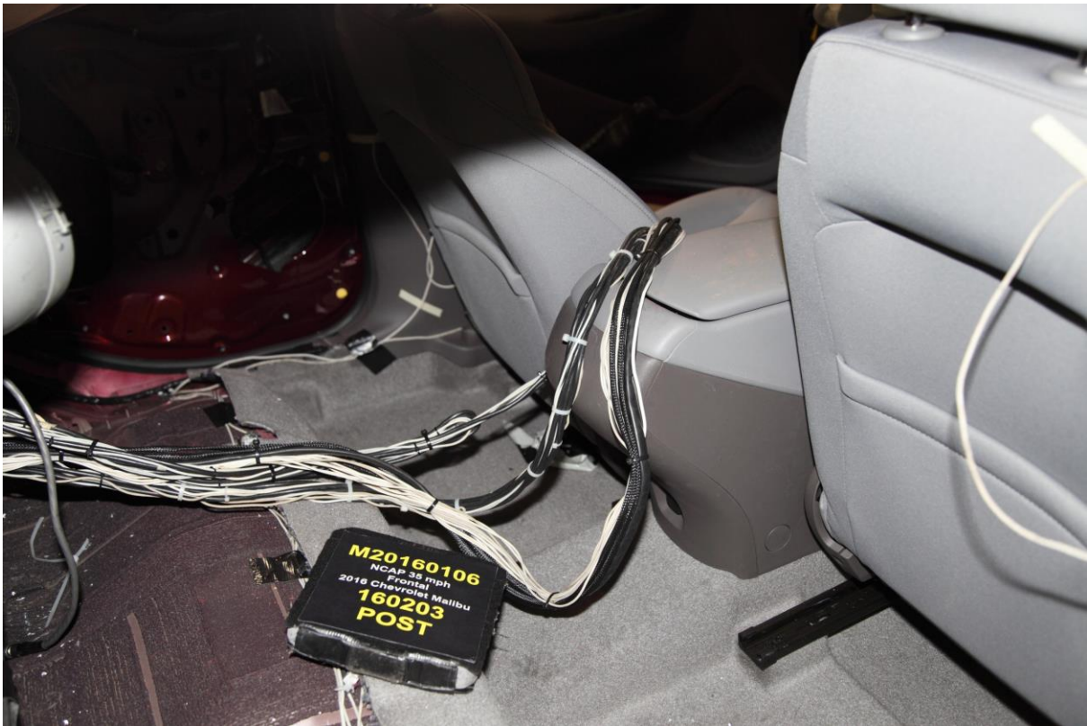
029 Post-Test Dummy Cable Routing
