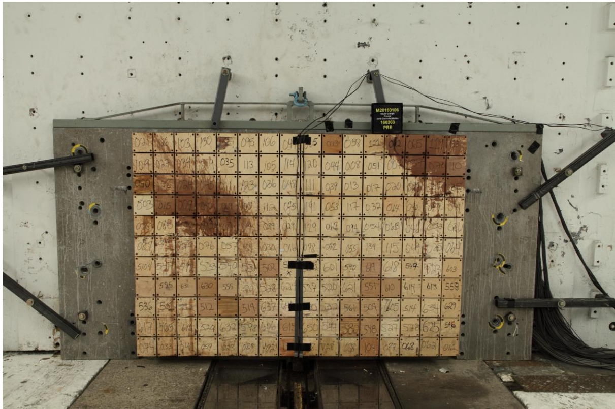
002 Pre-Test Load Cell Wall
