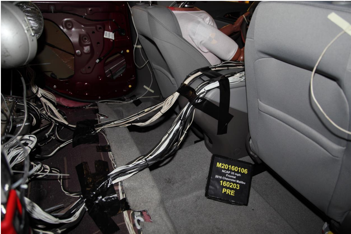
028 Pre-Test Dummy Cable Routing
