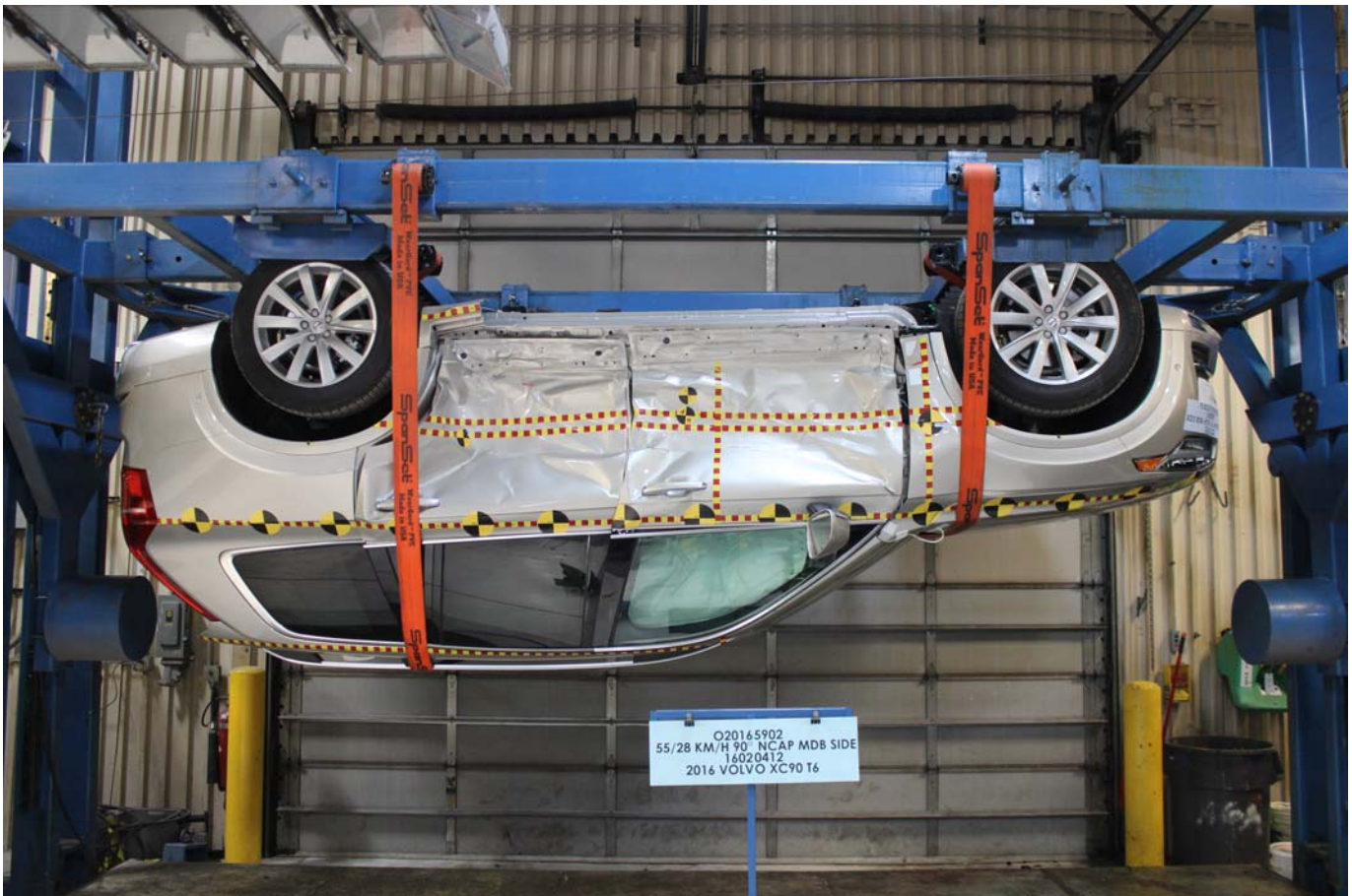
Photo No. 098 - FMVSS No. 301 Static Rollover 180 Degrees
