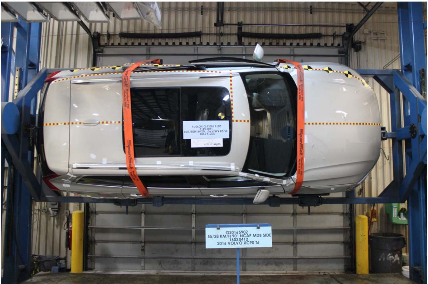
Photo No. 097 - FMVSS No. 301 Static Rollover 90 Degrees
