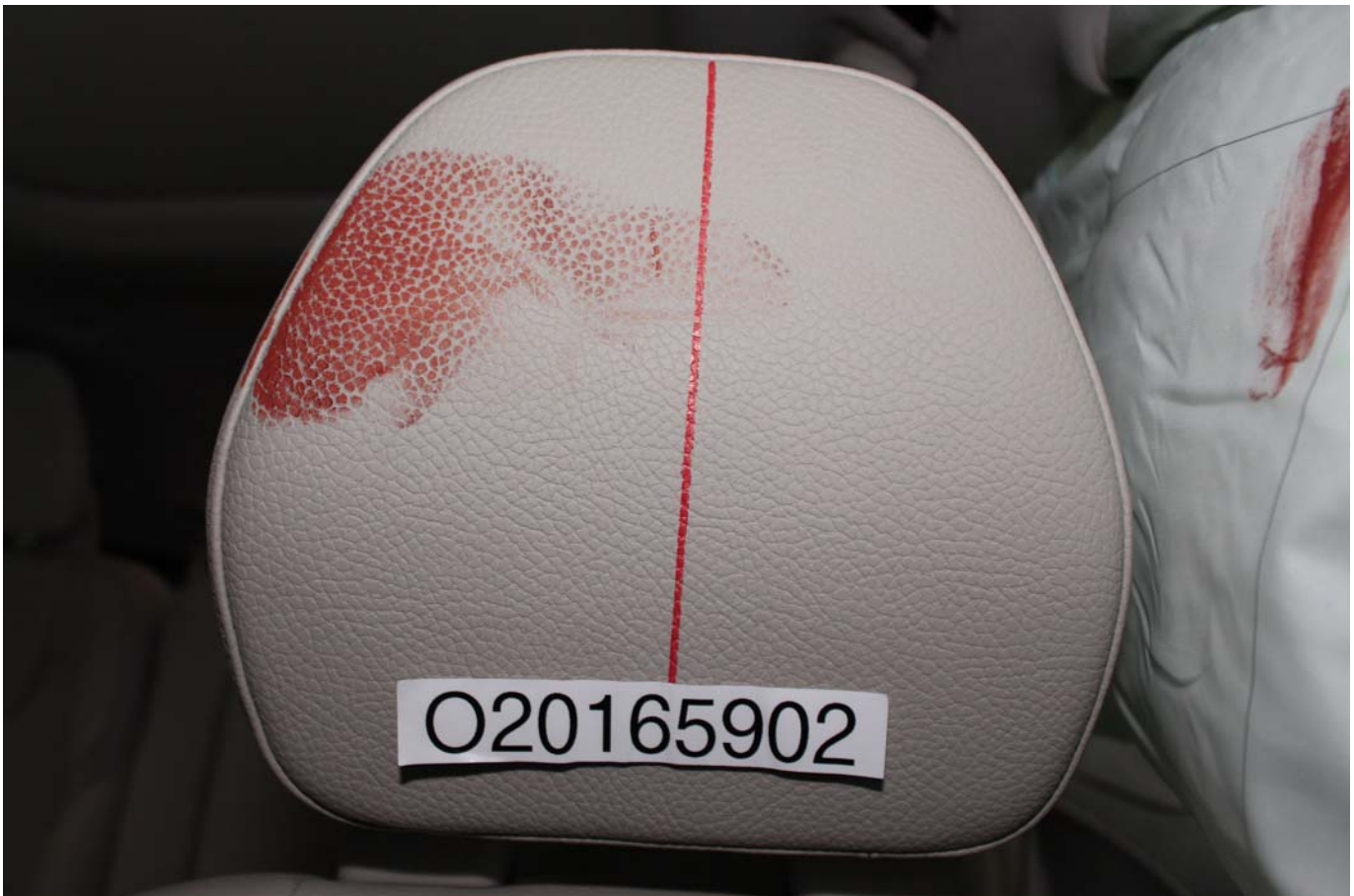
Photo No. 048 - Post-Test Driver Dummy Close-up Head Contact with Vehicle Interior View
