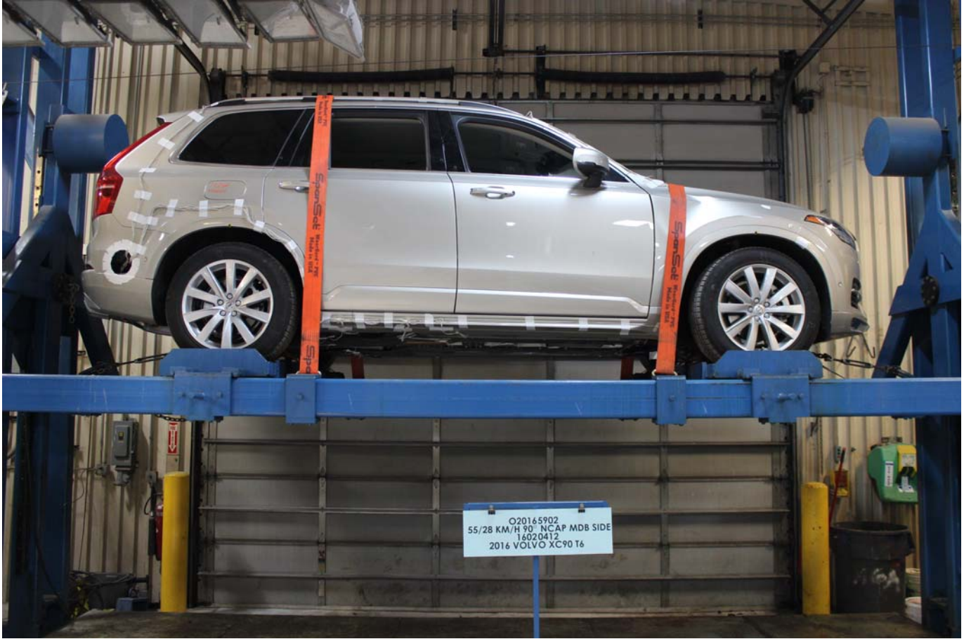
Photo No. 096 - FMVSS No. 301 Static Rollover 0 Degrees
