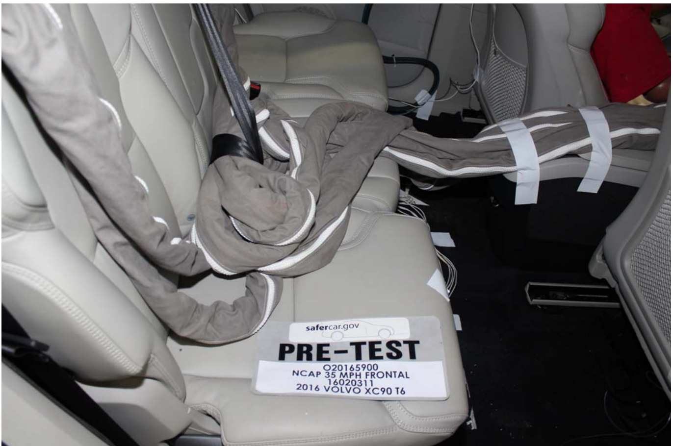
Photo No. 028 - Pre-Test Dummy Cable Routing
