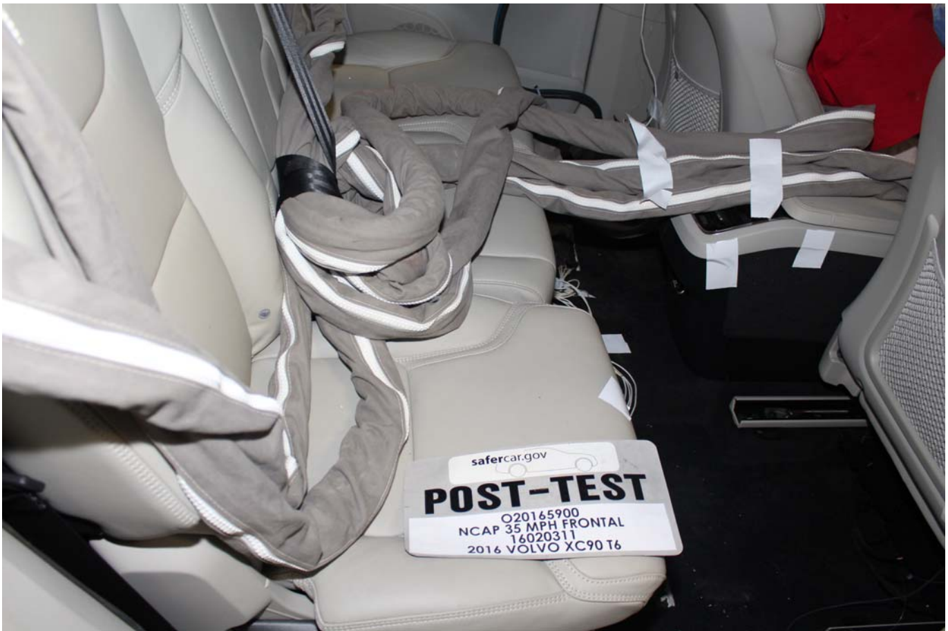
Photo No. 029 - Post-Test Dummy Cable Routing
