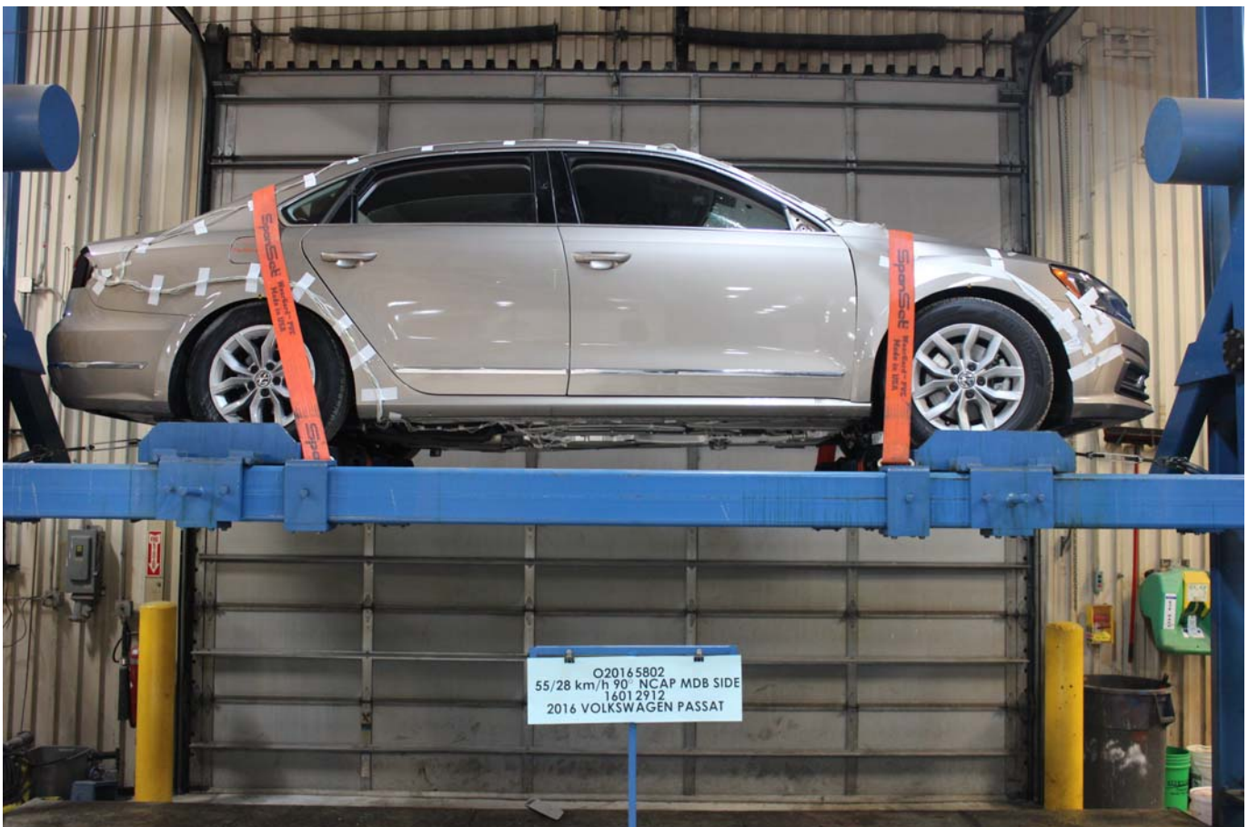
Photo No. 100 - FMVSS No. 301 Static Rollover 360 Degrees
