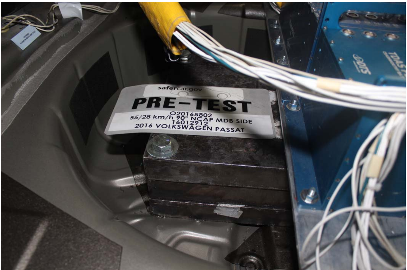
Photo No. 094 - Pre-Test Ballast View
