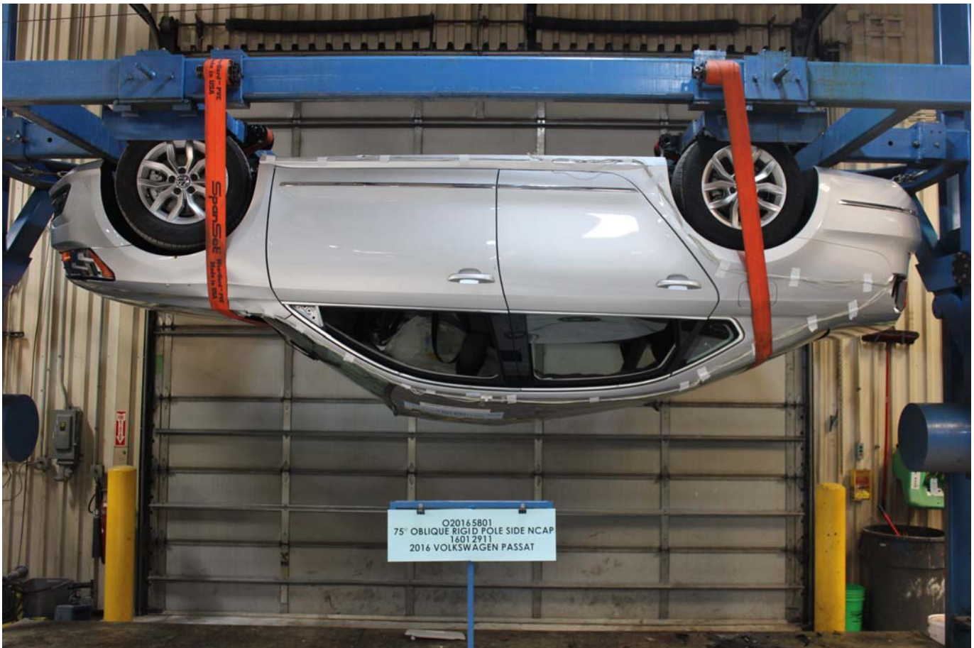
Photo No. 065 - FMVSS No. 301 Static Rollover 180 Degrees
