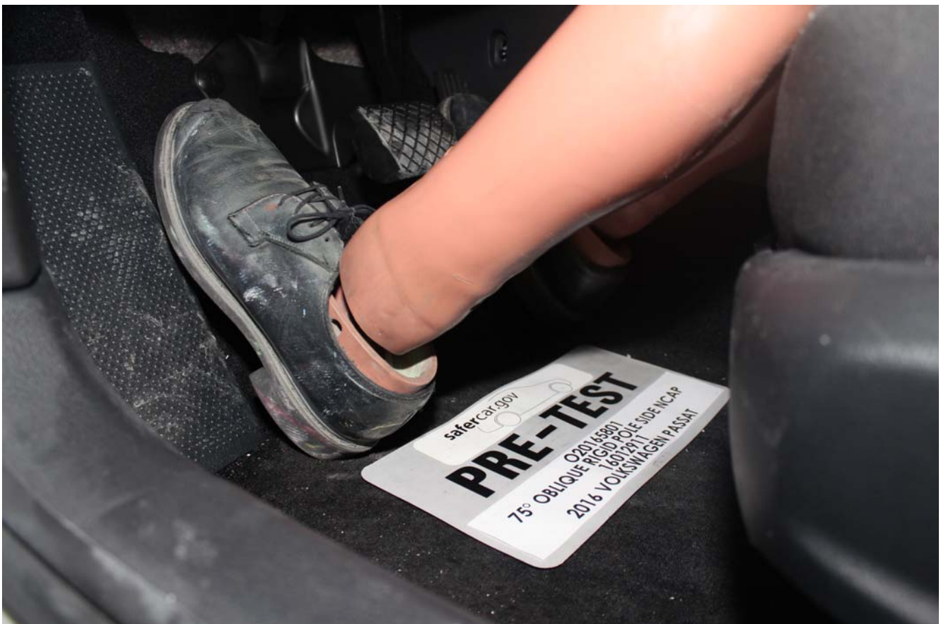
Photo No. 032 - Pre-Test Placement of Dummy's Feet
