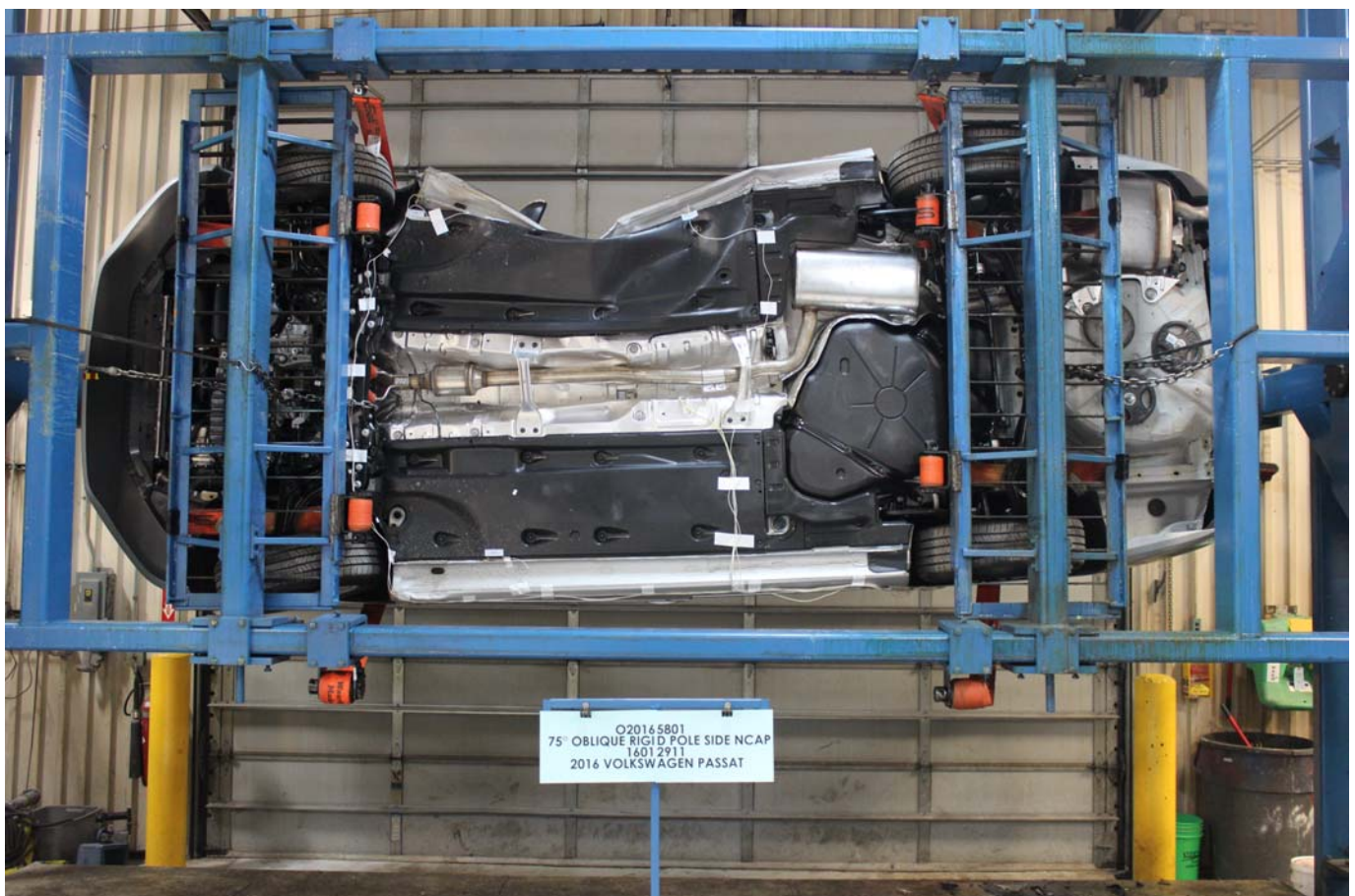
Photo No. 064 - FMVSS No. 301 Static Rollover 90 Degrees
