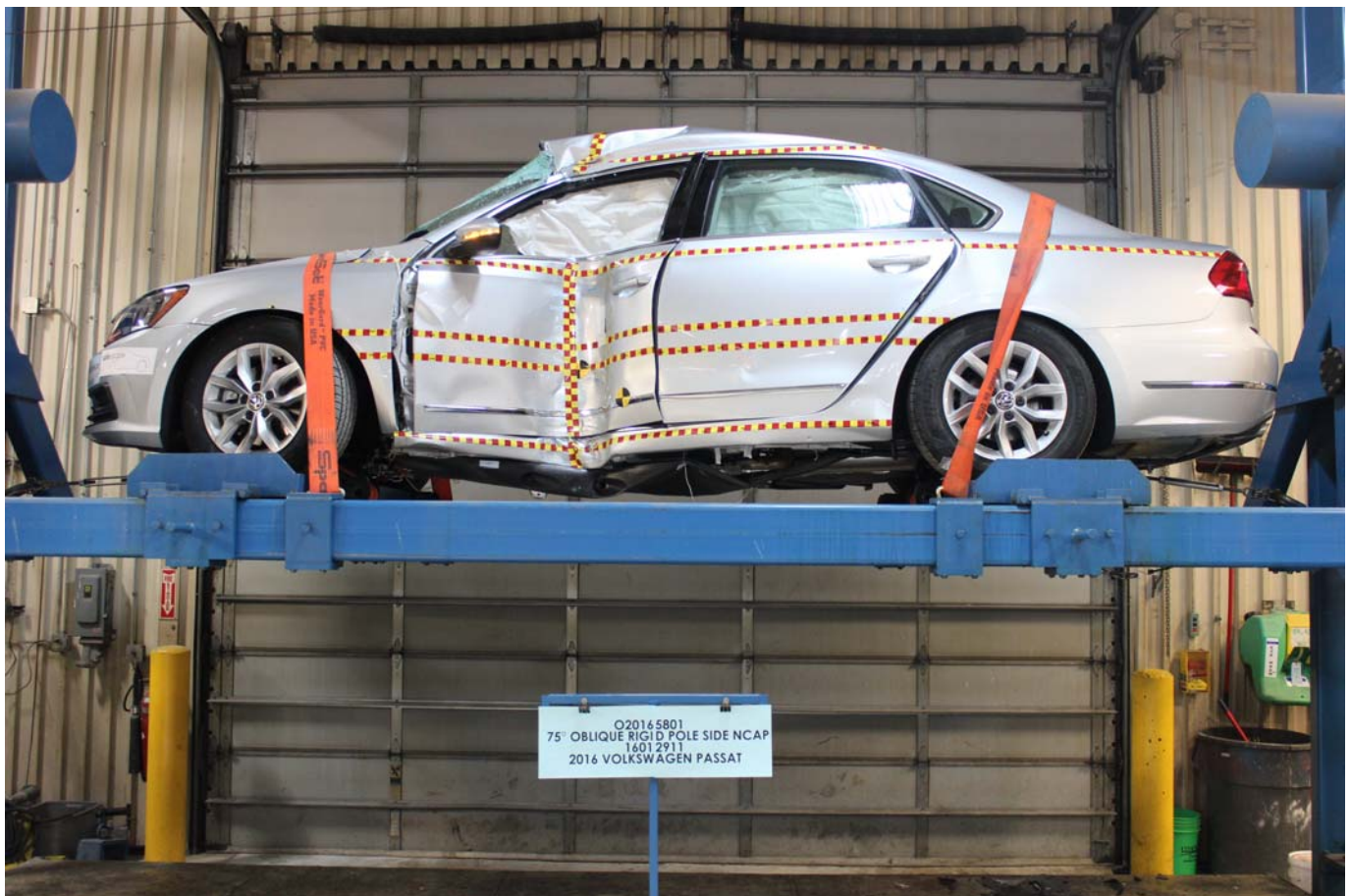
Photo No. 063 - FMVSS No. 301 Static Rollover 0 Degrees
