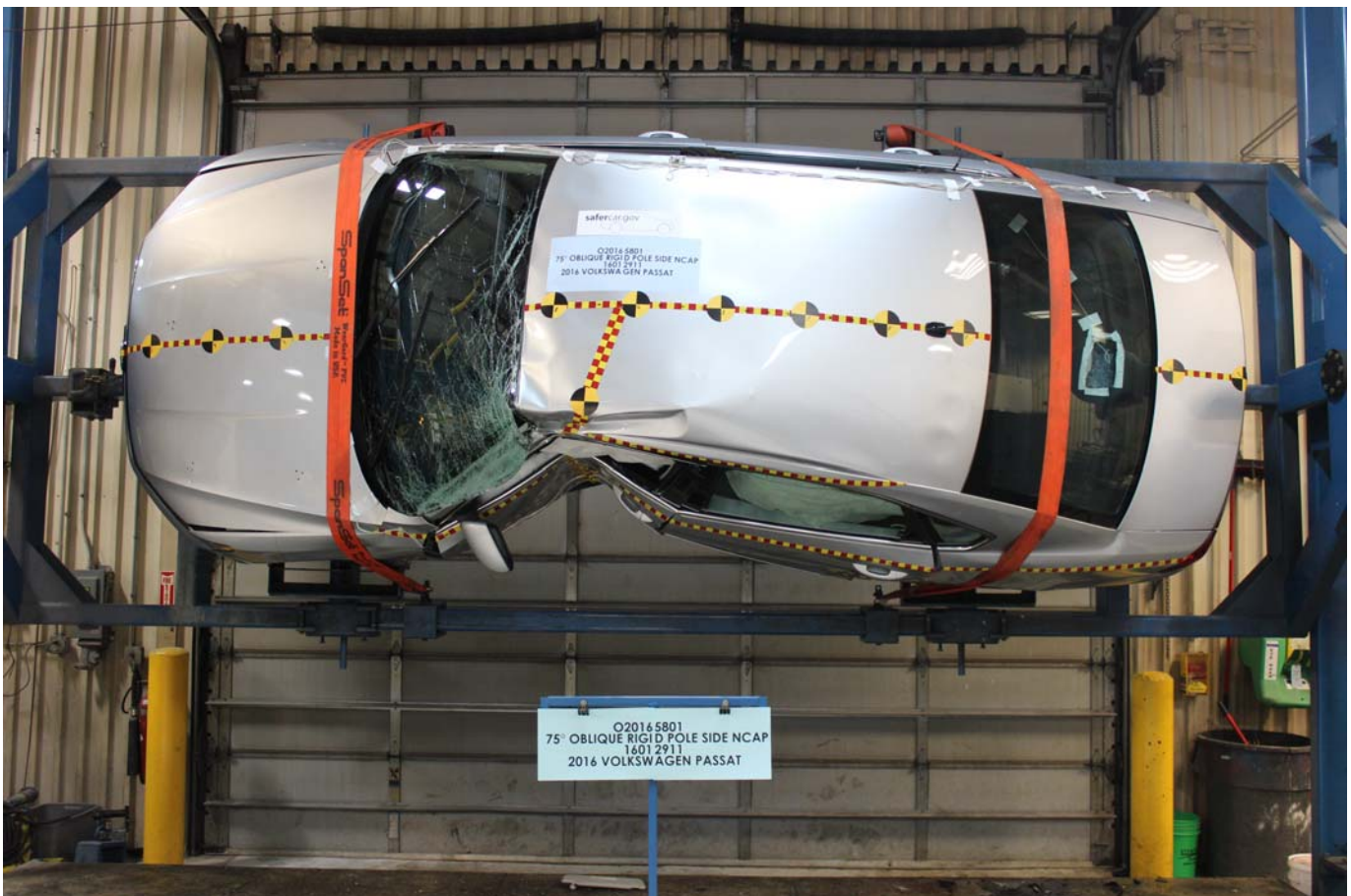
Photo No. 066 - FMVSS No. 301 Static Rollover 270 Degrees
