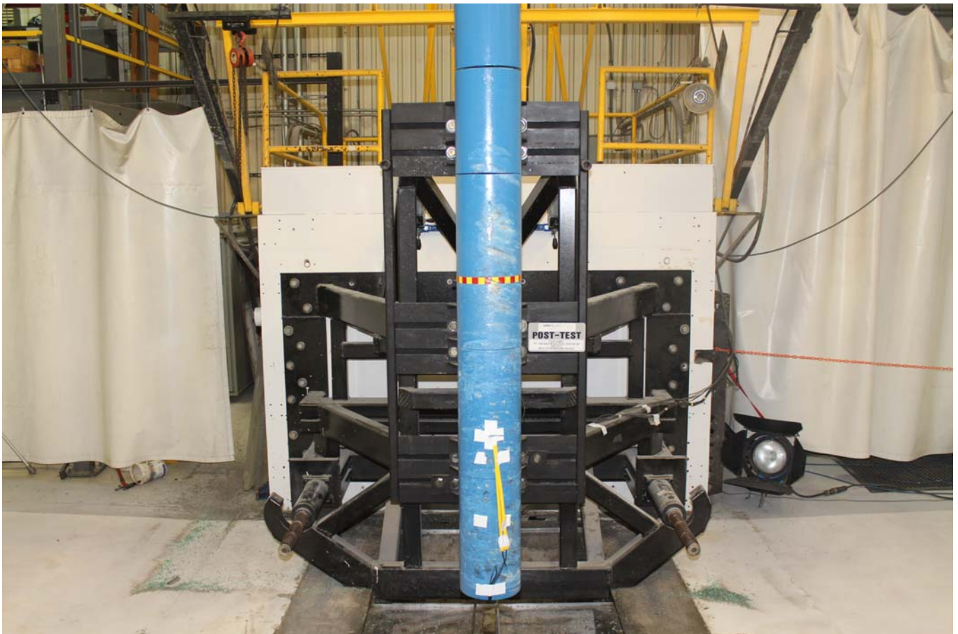
Photo No. 058 - Post-Test Pole Barrier Front View
