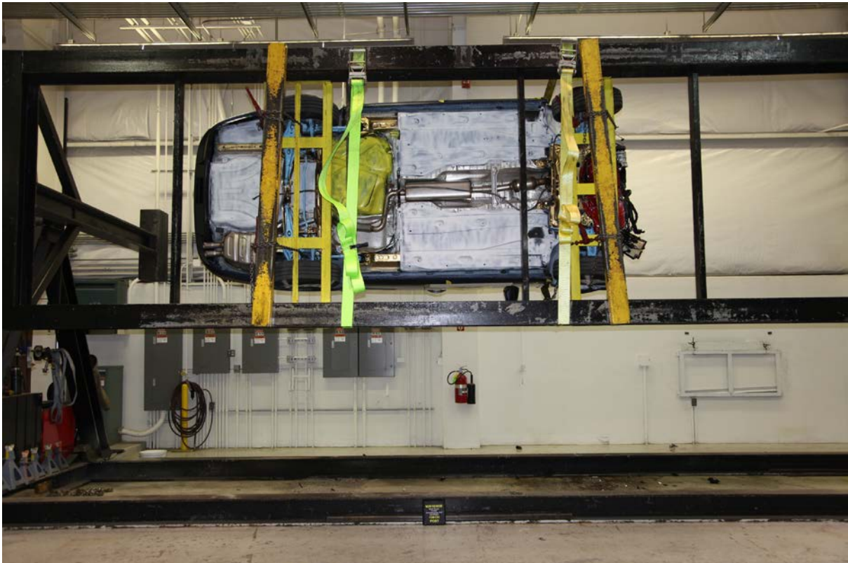
076 Vehicle at 270° on Static Rollover Device
