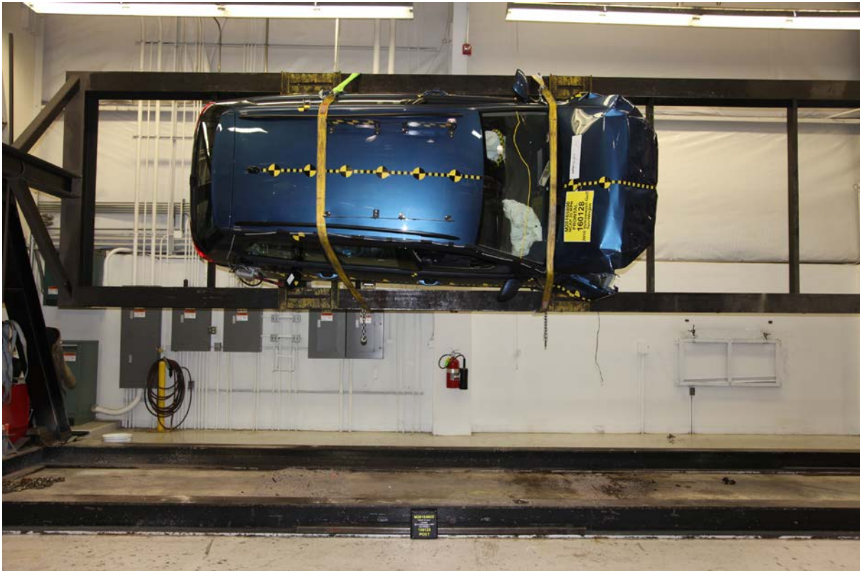
074 Vehicle at 90° on Static Rollover Device
