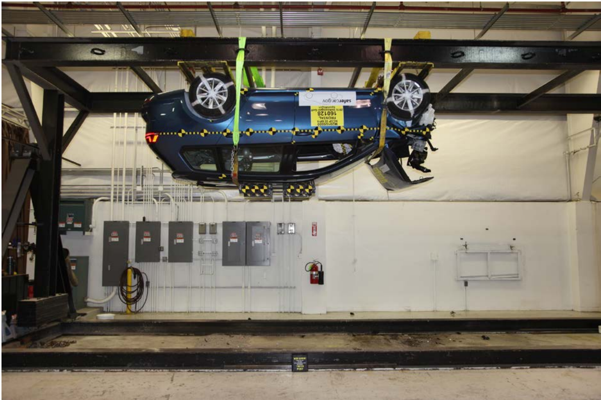
075 Vehicle at 180° on Static Rollover Device
