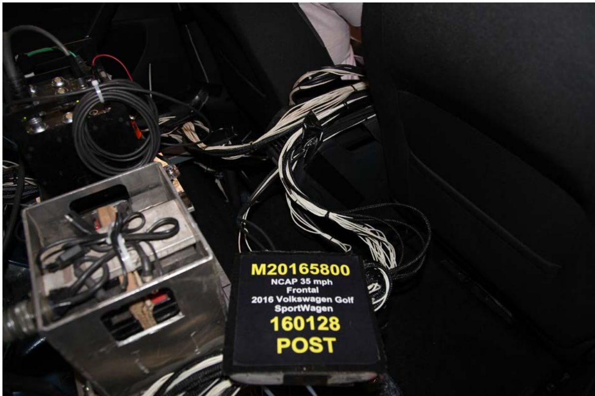
029 Post-Test Dummy Cable Routing
