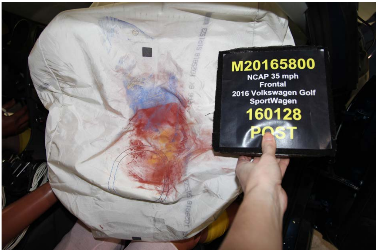
068 Post-Test Passenger Dummy Contact With Airbag
