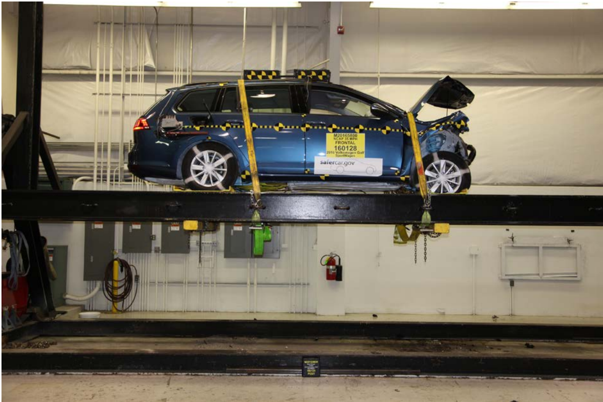
077 Vehicle at 360° on Static Rollover Device
