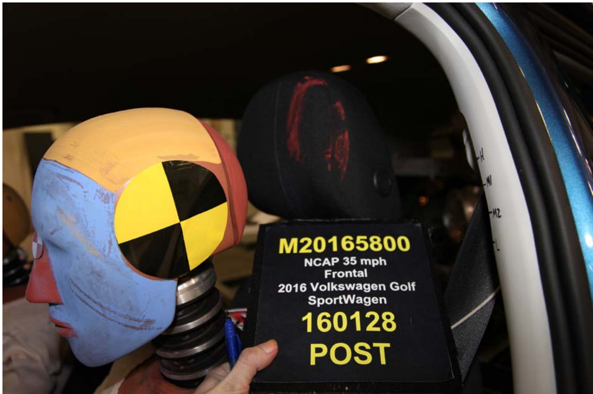
048 Post-Test Driver Dummy Contact With Headrest
