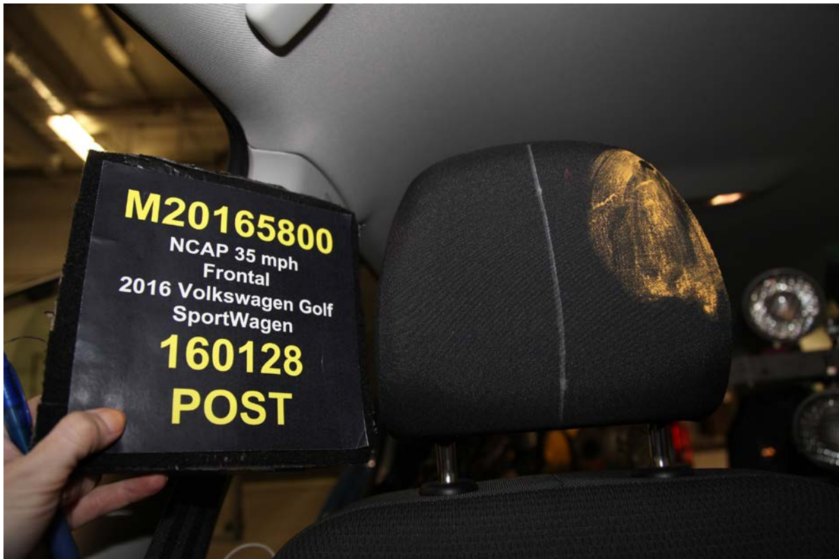
069 Post Test Passenger Dummy Contact With Headrest
