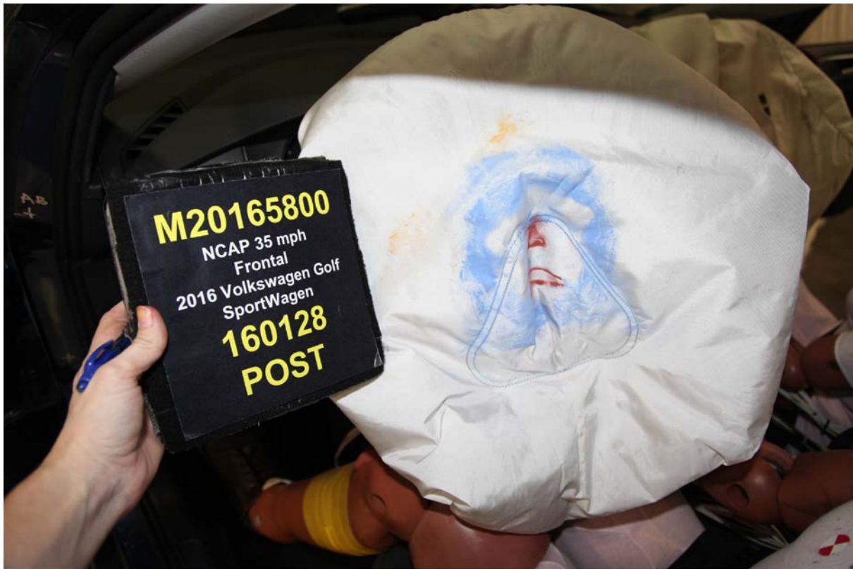
047 Post-Test Driver Dummy Contact With Airbag
