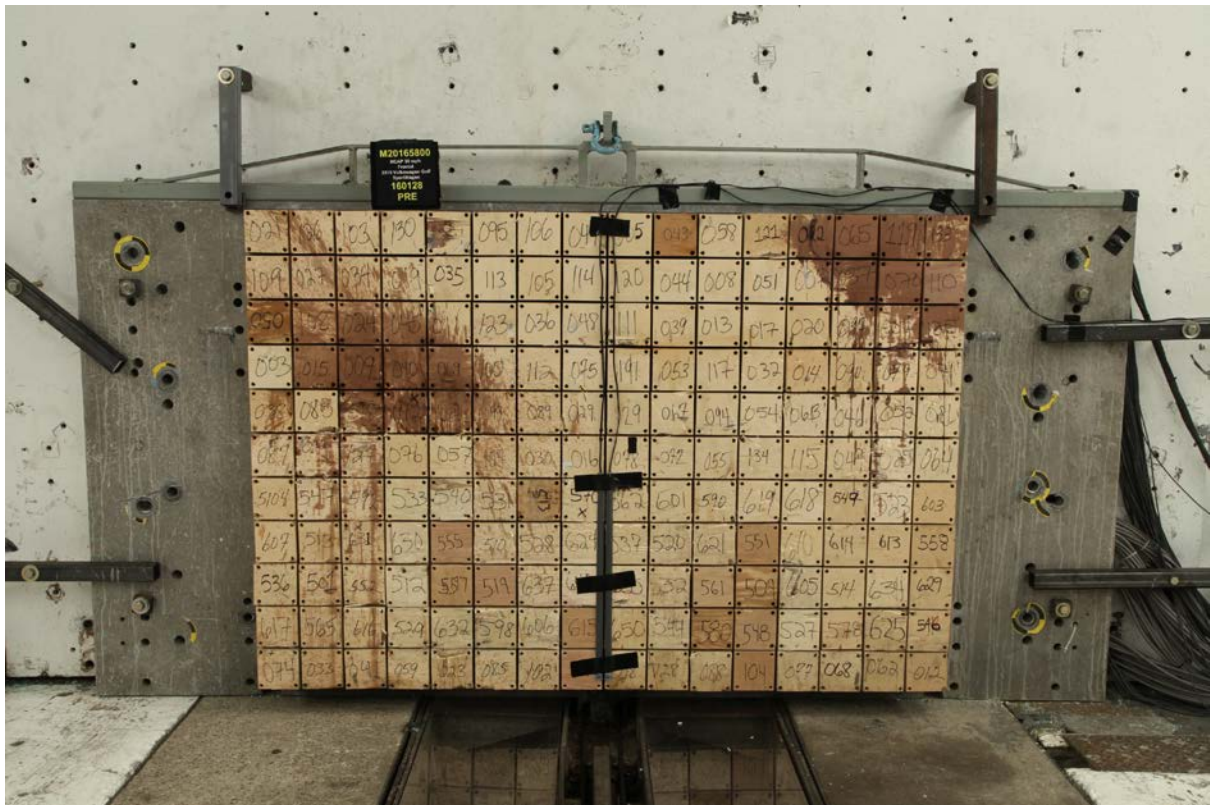
002 Pre-Test Load Cell Wall
