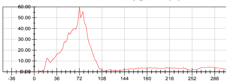
Driver Chest Resultant Acceleration vs. Time Primary (g) vs. Time [ms]
