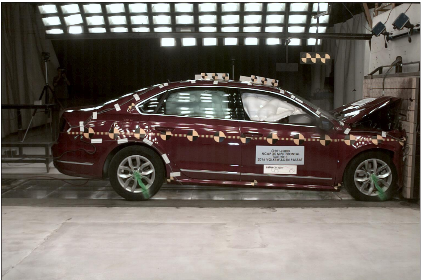
Photo No. 078 - 2016 Volkswagen Passat 1.8T S Frontal Impact Event
