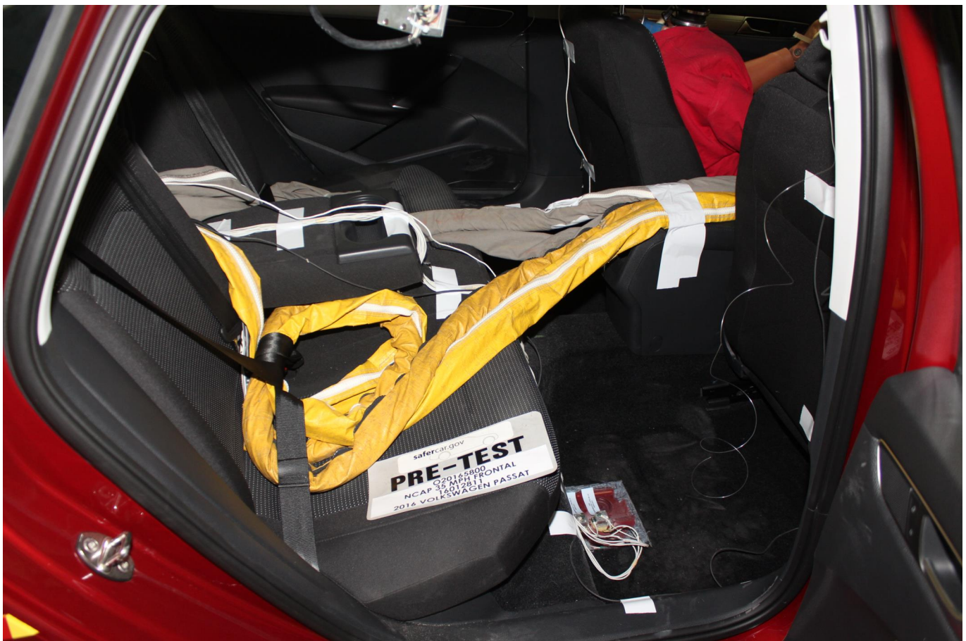
Photo No. 028 - Pre-Test Dummy Cable Routing
