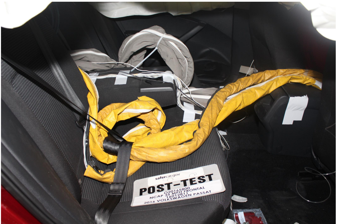
Photo No. 029 - Post-Test Dummy Cable Routing
