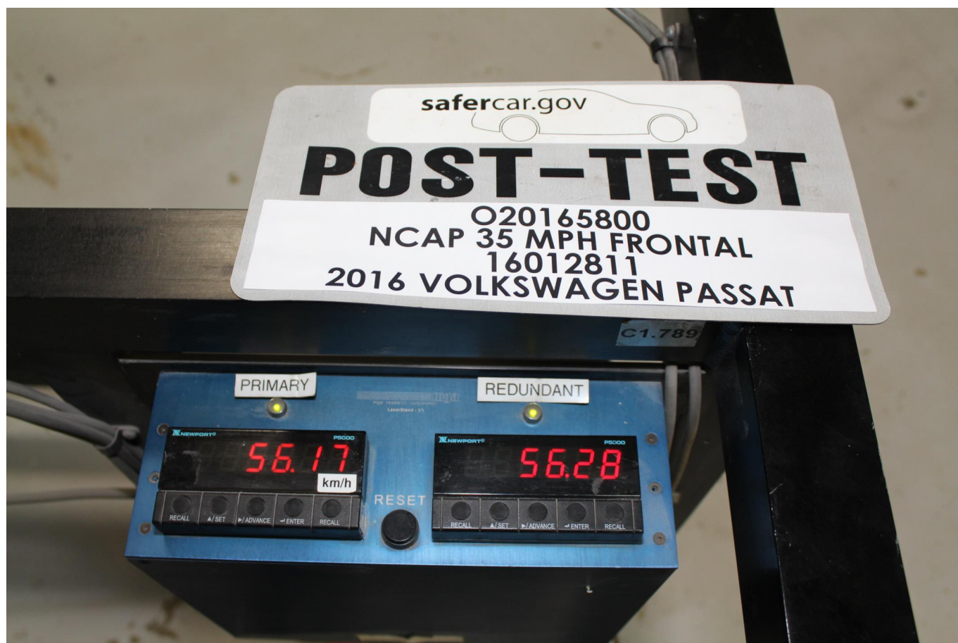
Photo No. 072 - Post-Test Speed Trap Read-Out
