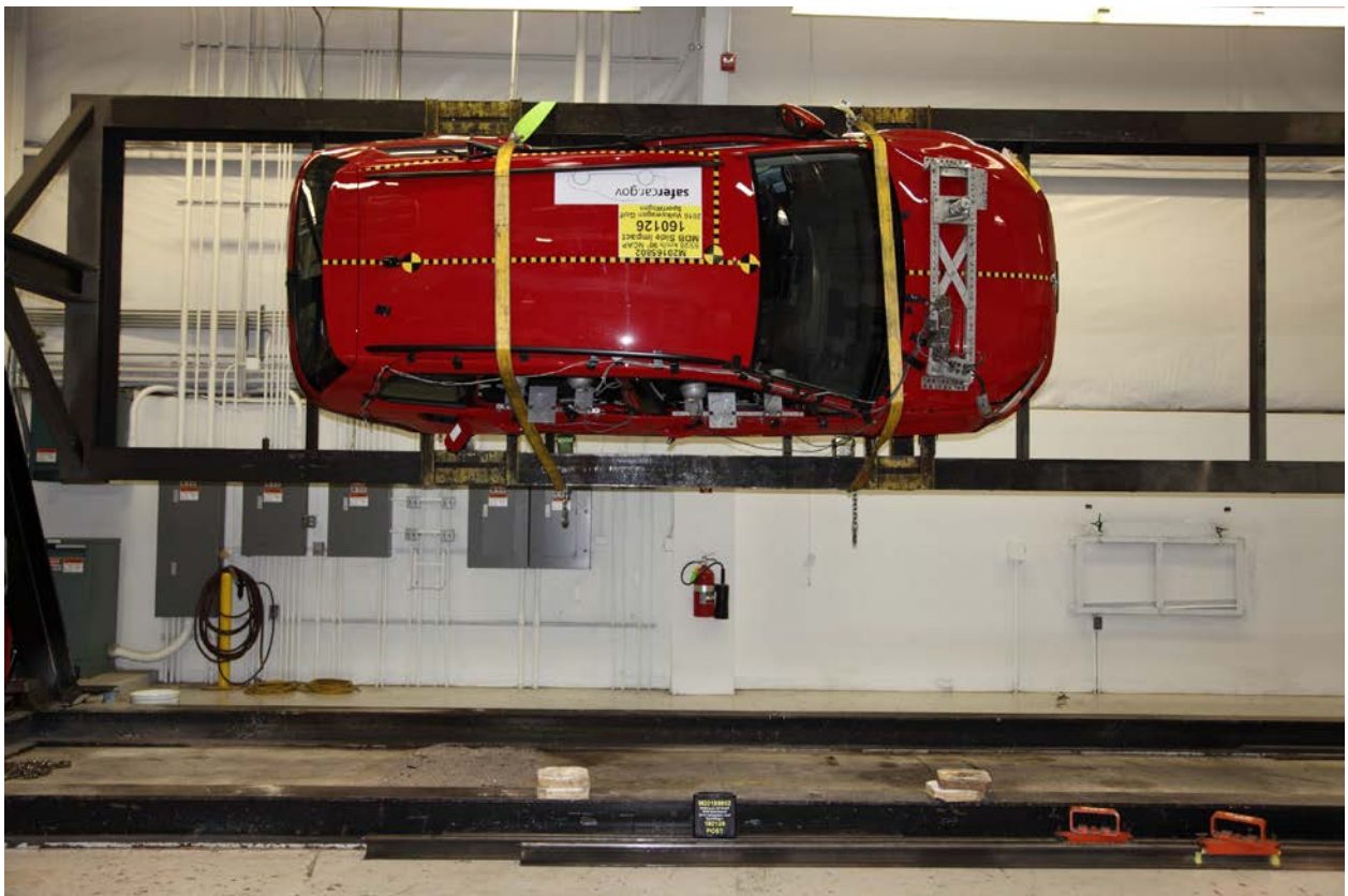
097 FMVSS No. 301 Static Rollover 90 Degrees
