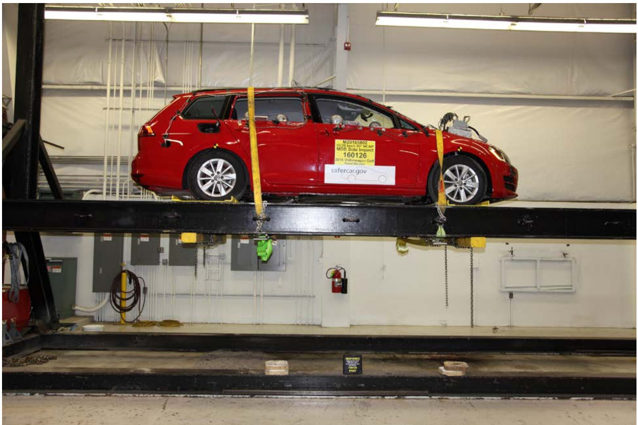
100 FMVSS No. 301 Static Rollover 360 Degrees
