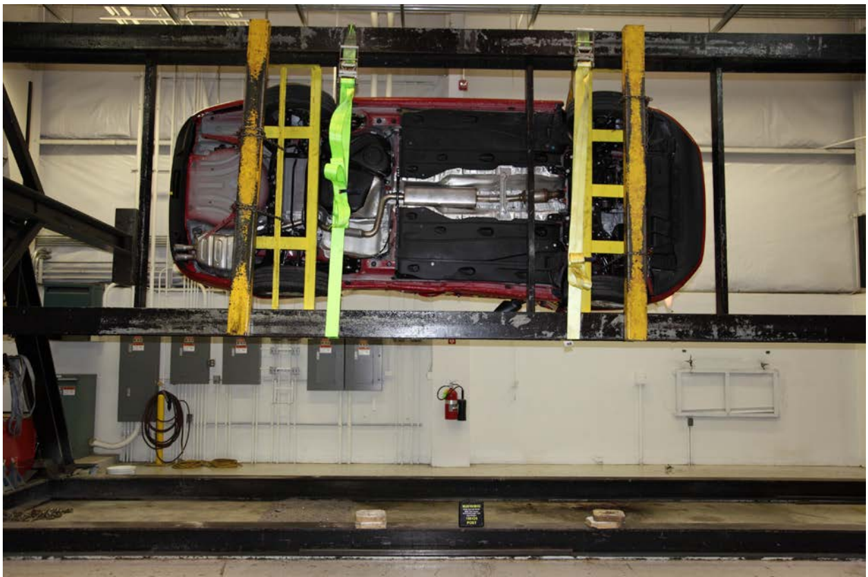
099 FMVSS No. 301 Static Rollover 270 Degrees
