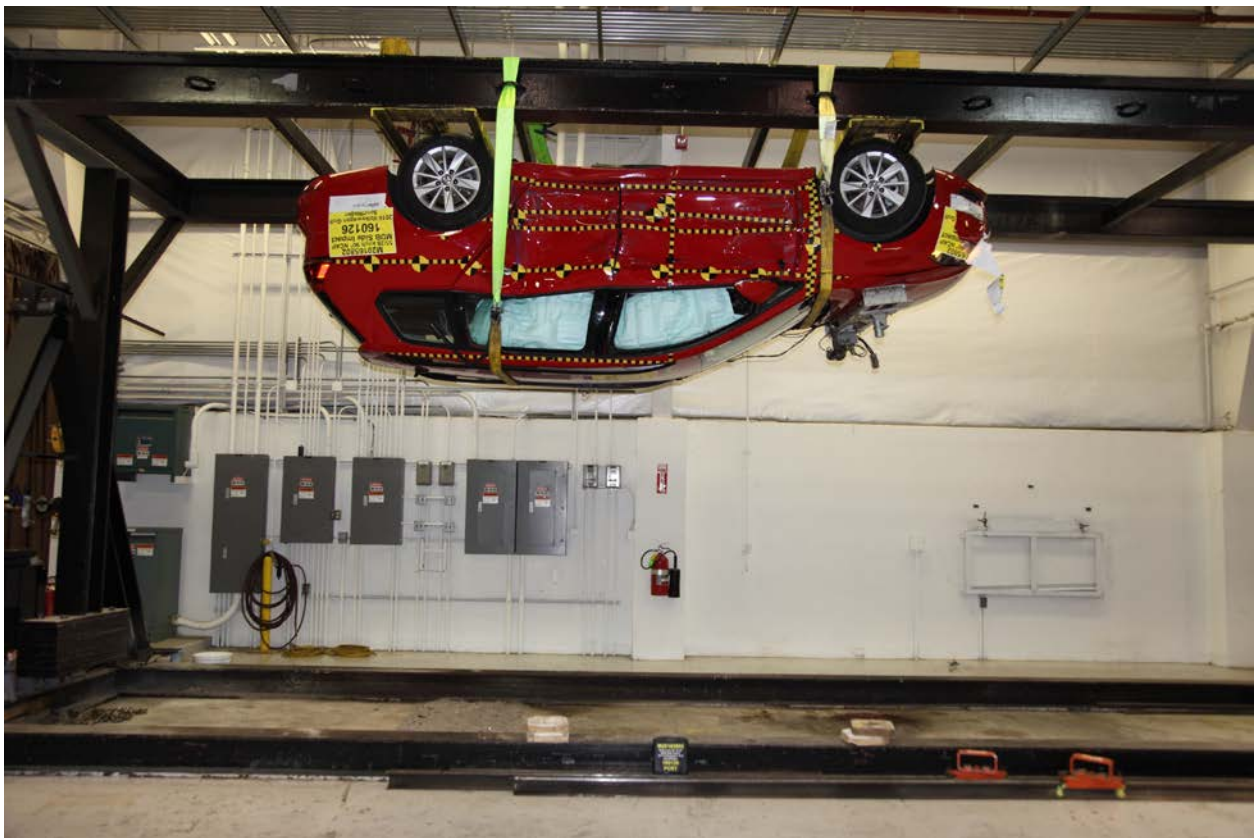
098 FMVSS No. 301 Static Rollover 180 Degrees
