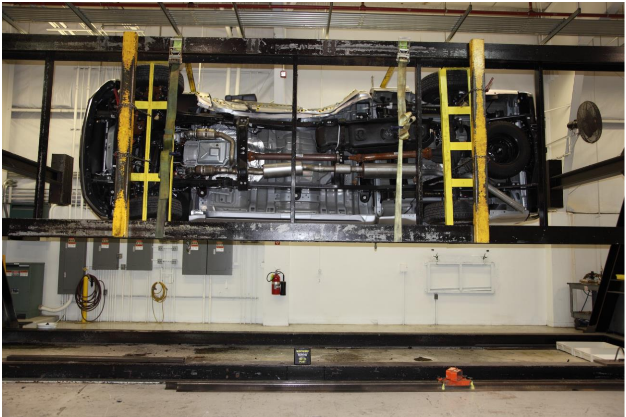
099 FMVSS No. 301 Static Rollover 270 Degrees
