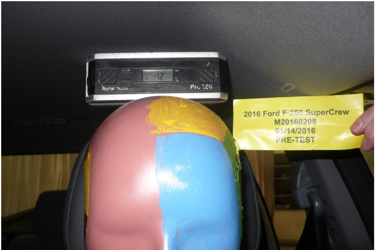
025 Pre-Test Front Close-up View of Driver Dummy
