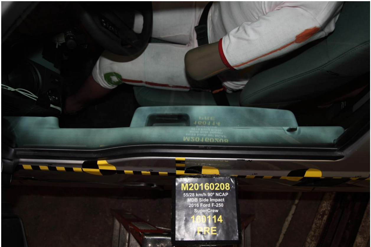
042 Pre-Test Driver Dummy and Door Clearance View
