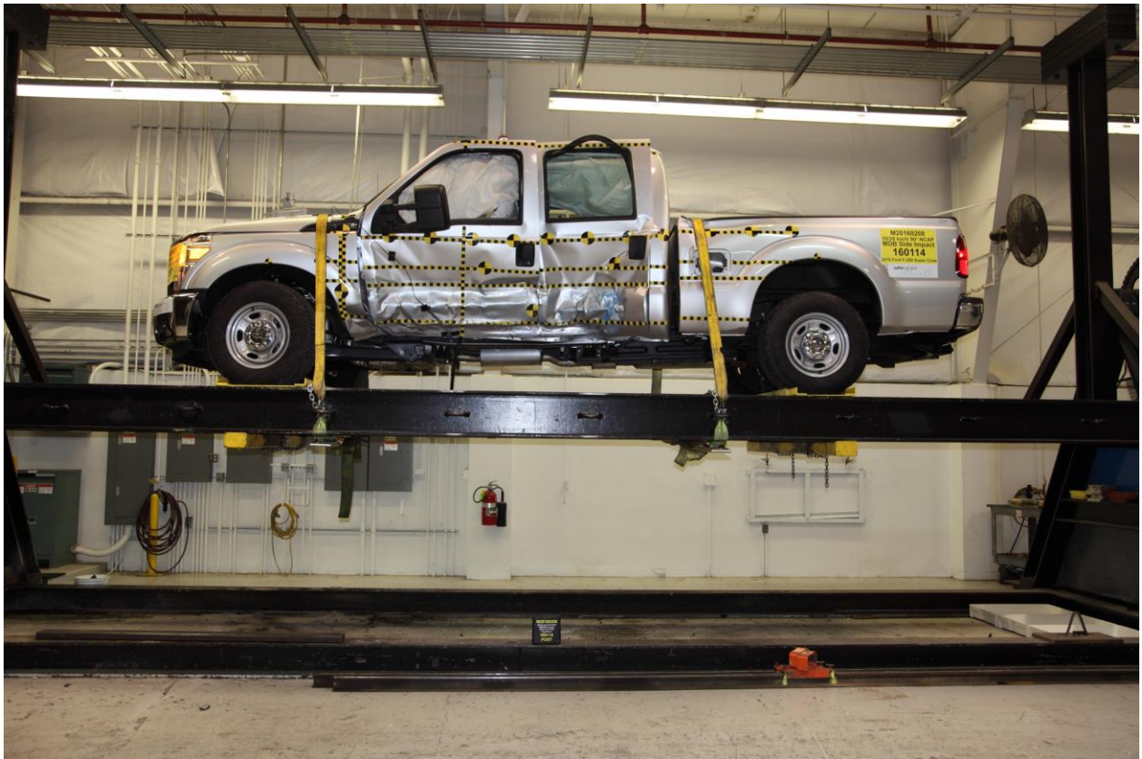
100 FMVSS No. 301 Static Rollover 360 Degrees
