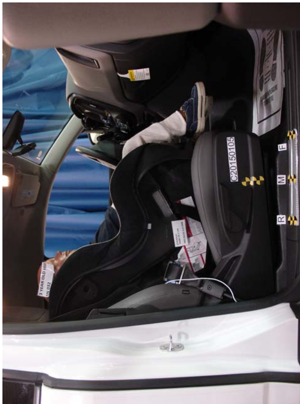
3-Year-Old Forward Facing Evenflo Tribute Cinched With Harness, Middle Seat Track
