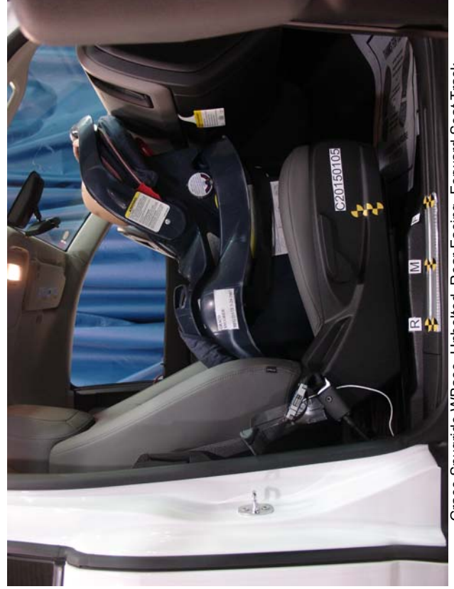
Graco Snuggly WBase, Unbelted, Rear Facing, Forward Seat Track
