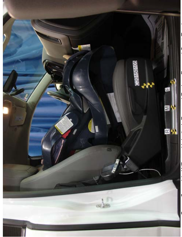
Graco Snuggly WBBase, Unbelted, Forward Facing, Forward Seat Track
