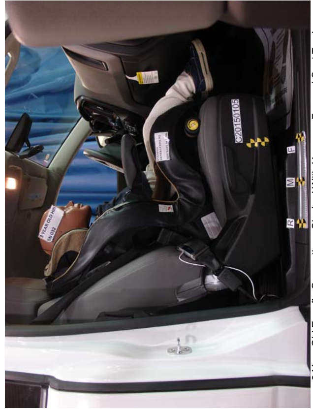
3-Year-Old Evenflo Generations Cinched With Harness, Forward Seat Track
