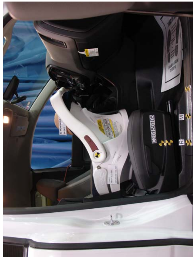
Cosco Arriva WBase, Belted, Rear Facing, Rearward Seat Track
