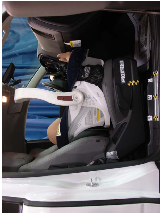
Cosco Arriva WBBase, Unbelted, Forward Facing, Forward Seat Track
