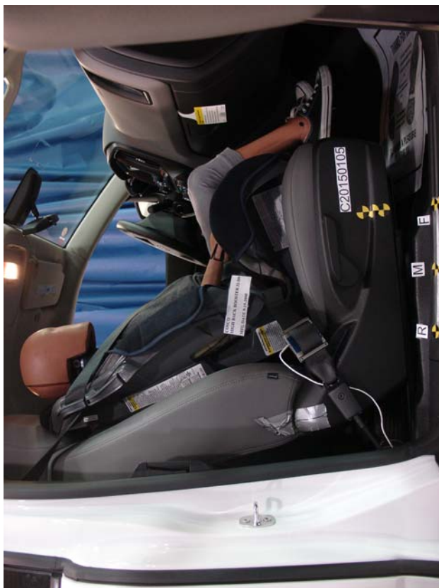
6-Year-Old Cosco High Back Booster Belted, Forward Seat Track
