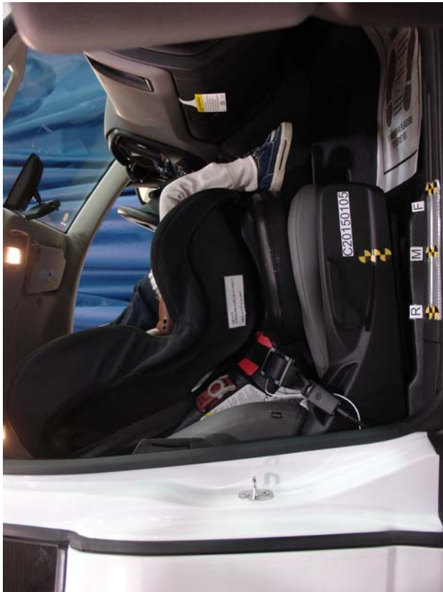
3-Year-Old Forward Facing Graco Toddler Safeseat Step 2 Cinched With Harness, Middle
