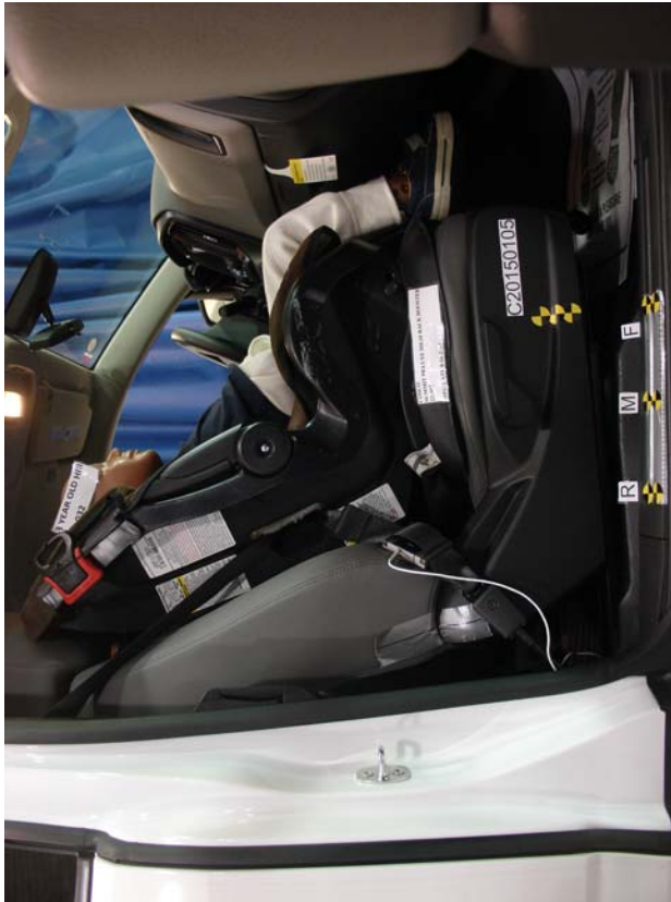
3-Year-Old Forward Facing Cosco Summit Deluxe Cinched With Harness, Forward Seat
