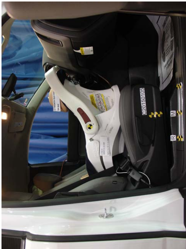
Cosco Arriva WBase, Belted, Rear Facing, Middle Seat Track
