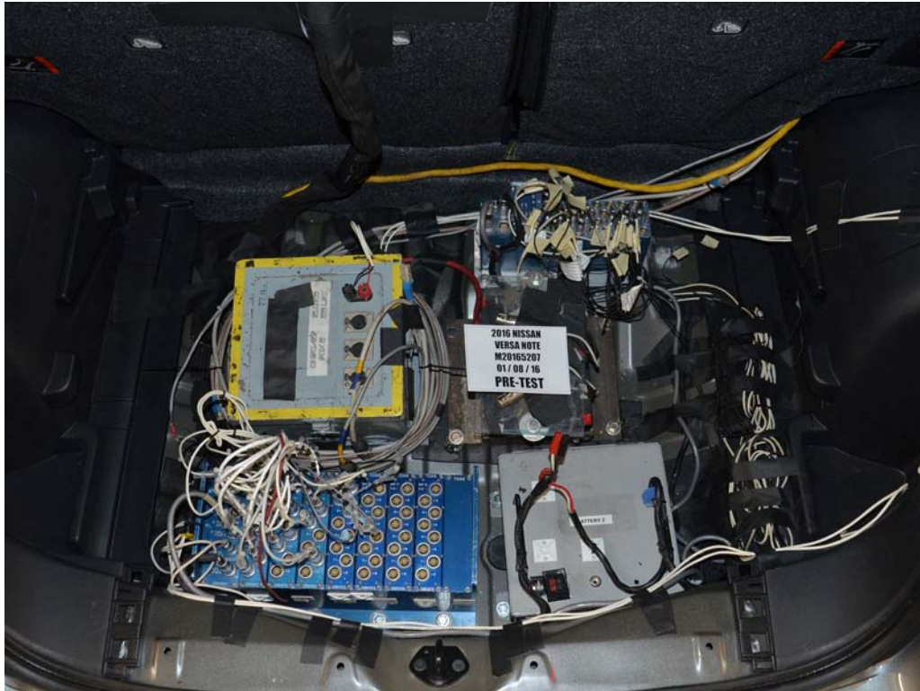
FIGURE 61. Pre-Test Ballast View
