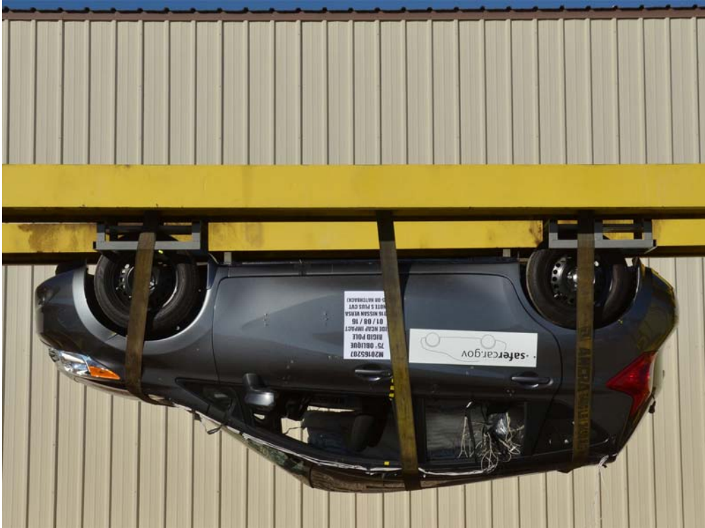
FIGURE 65. FMVSS No. 301 Static Rollover 180 Degrees
