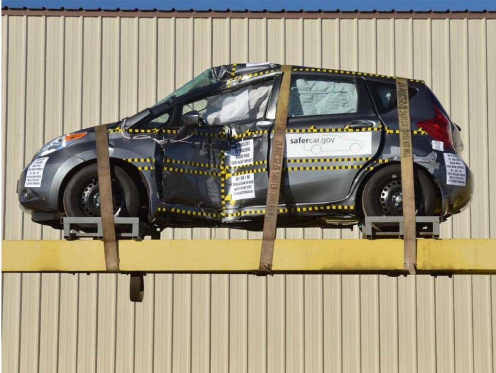
FIGURE 67. FMVSS No. 301 Static Rollover 360 Degrees
