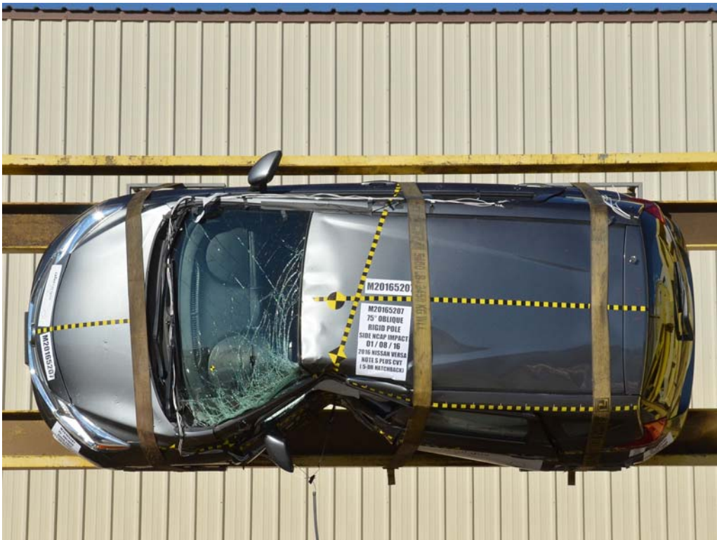
FIGURE 64. FMVSS No. 301 Static Rollover 90 Degrees
