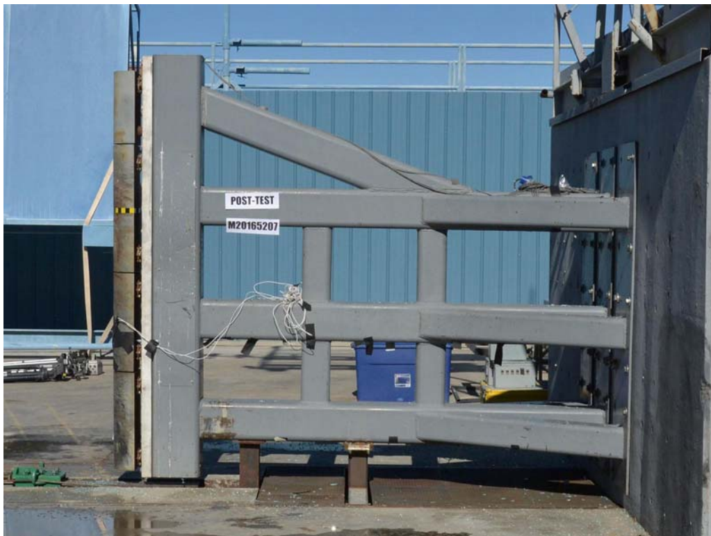
FIGURE 60. Post-Test Pole Barrier Side View
