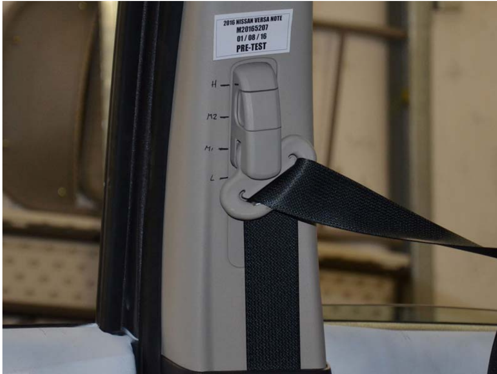
FIGURE 33. Pre-Test View of Belt Anchorage for Dummy
