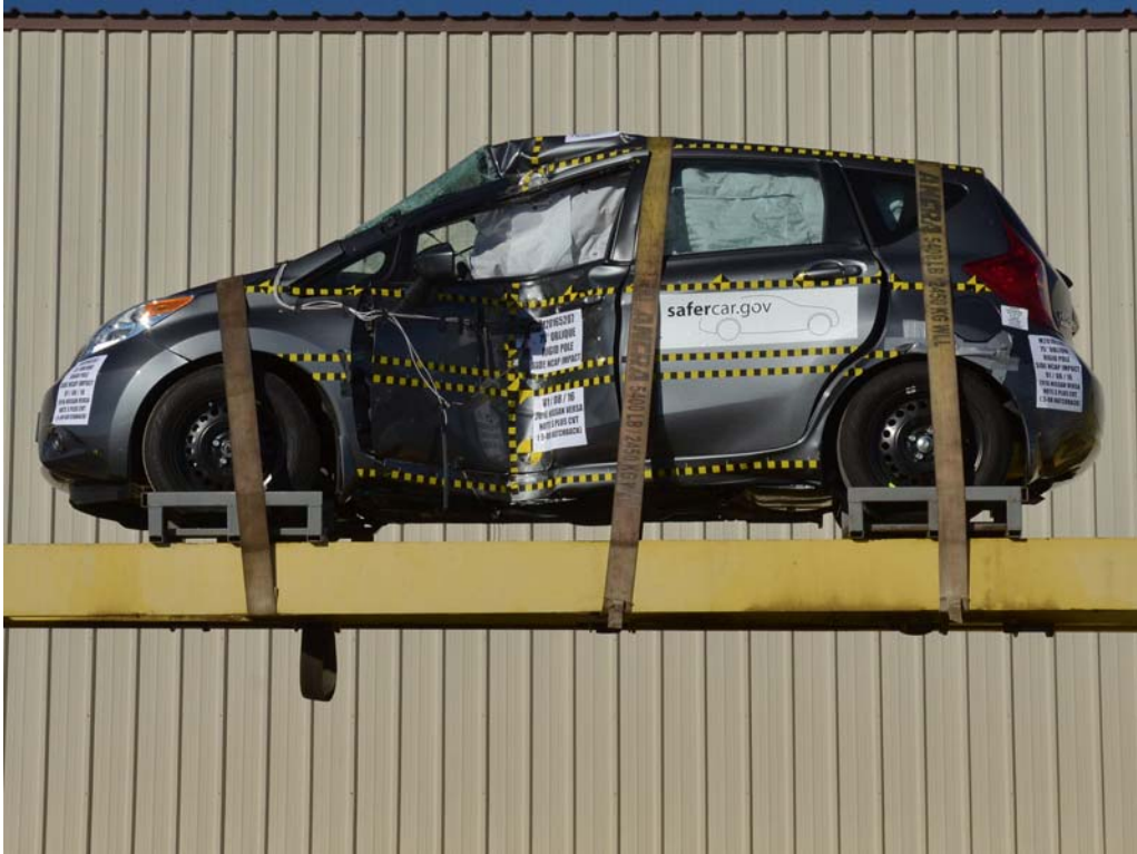
FIGURE 63. FMVSS No. 301 Static Rollover 0 Degrees
