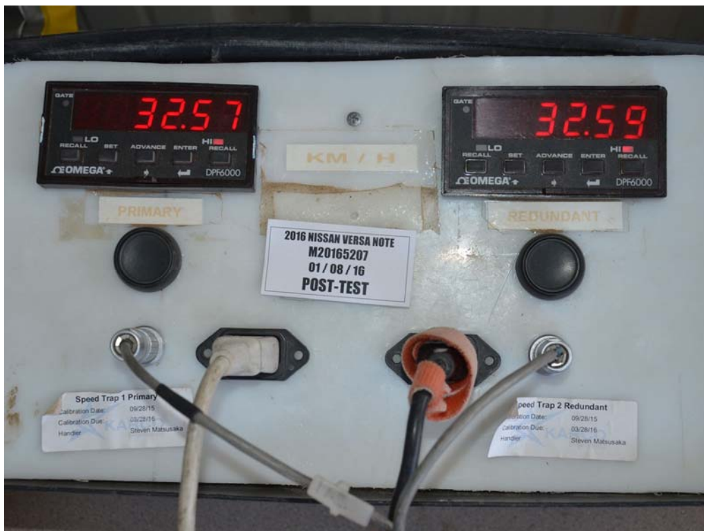
FIGURE 62. Post-Test Primary and Redundant Speed Trap Read-Out
