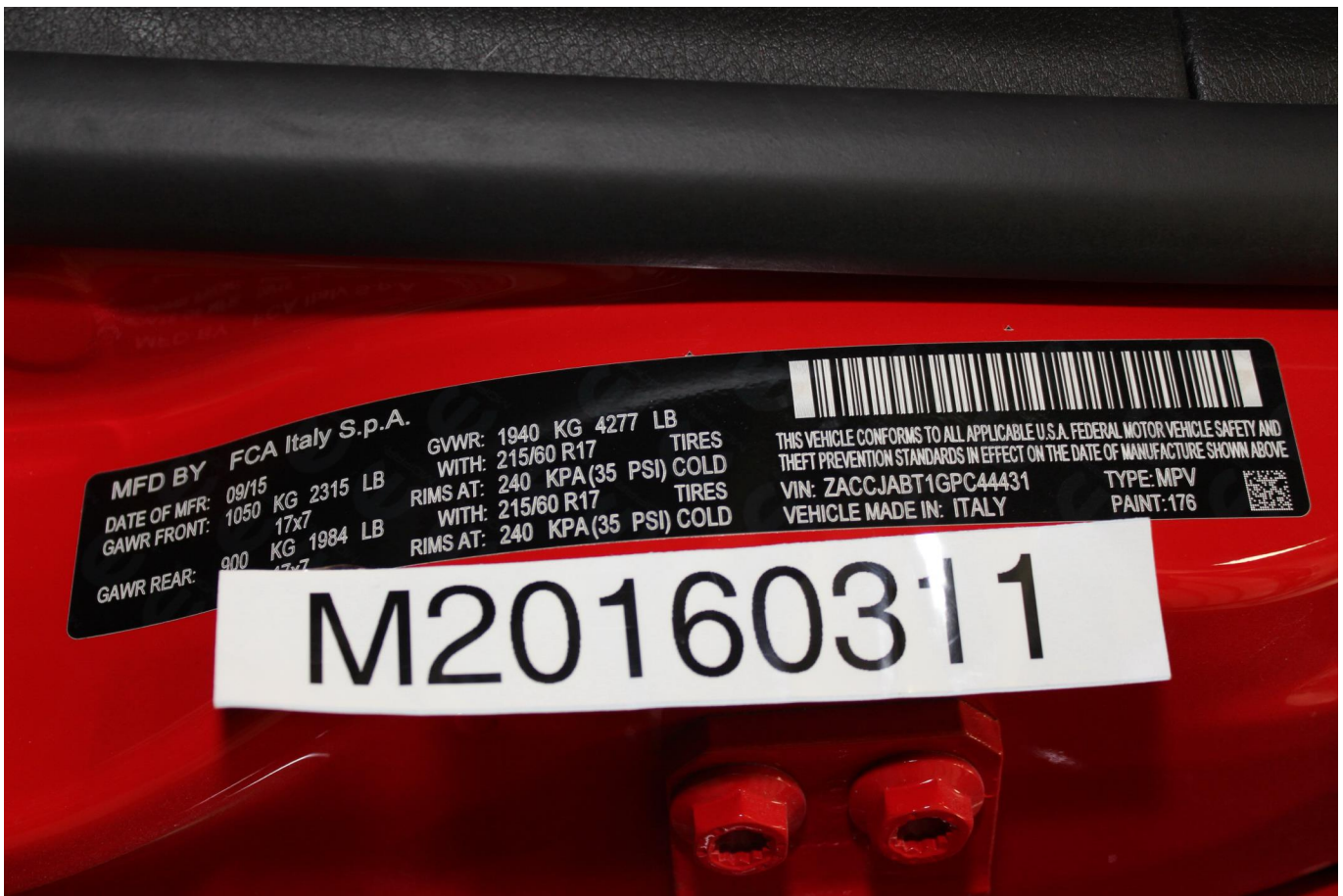
Photo No. 055 - Close-Up View of Vehicle's Certification Label
