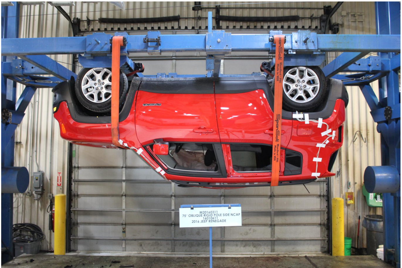
Photo No. 065 - FMVSS No. 301 Static Rollover 180 Degrees
