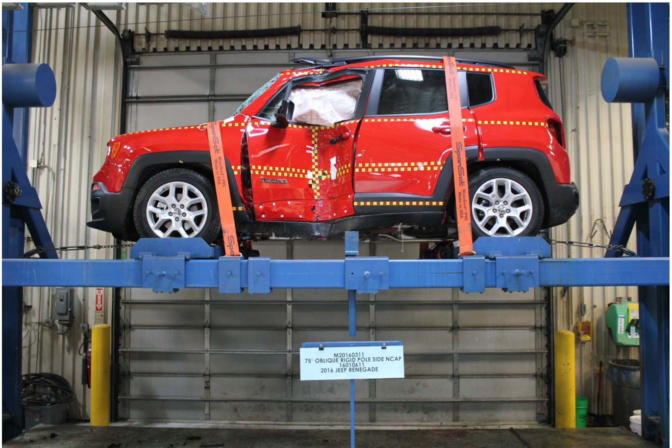
Photo No. 063 - FMVSS No. 301 Static Rollover 0 Degrees
