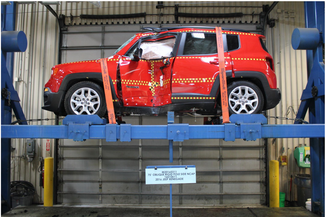
Photo No. 067 - FMVSS No. 301 Static Rollover 360 Degrees
