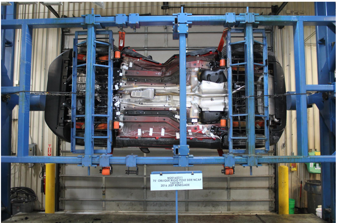
Photo No. 064 - FMVSS No. 301 Static Rollover 90 Degrees
