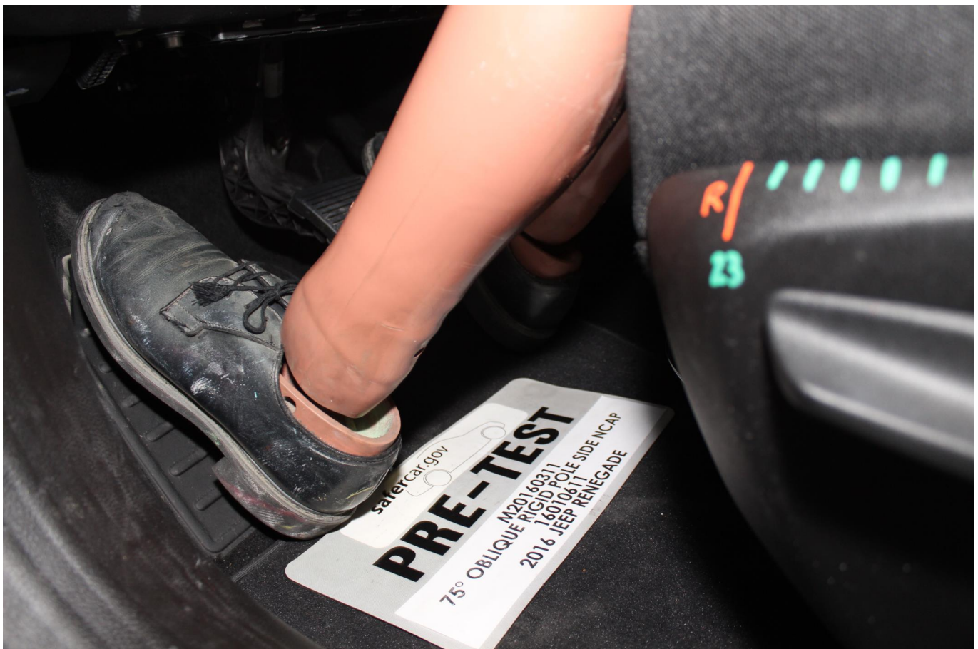
Photo No. 032 - Pre-Test Placement of Dummy's Feet
