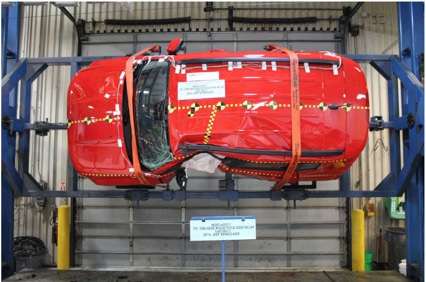
Photo No. 066 - FMVSS No. 301 Static Rollover 270 Degrees
