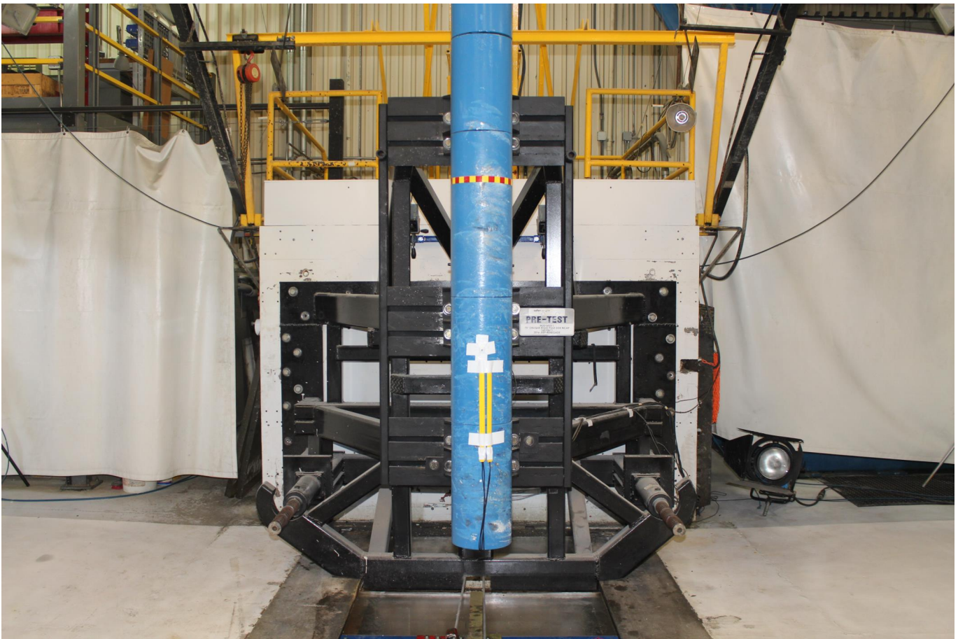
Photo No. 057 - Pre-Test Pole Barrier Front View
