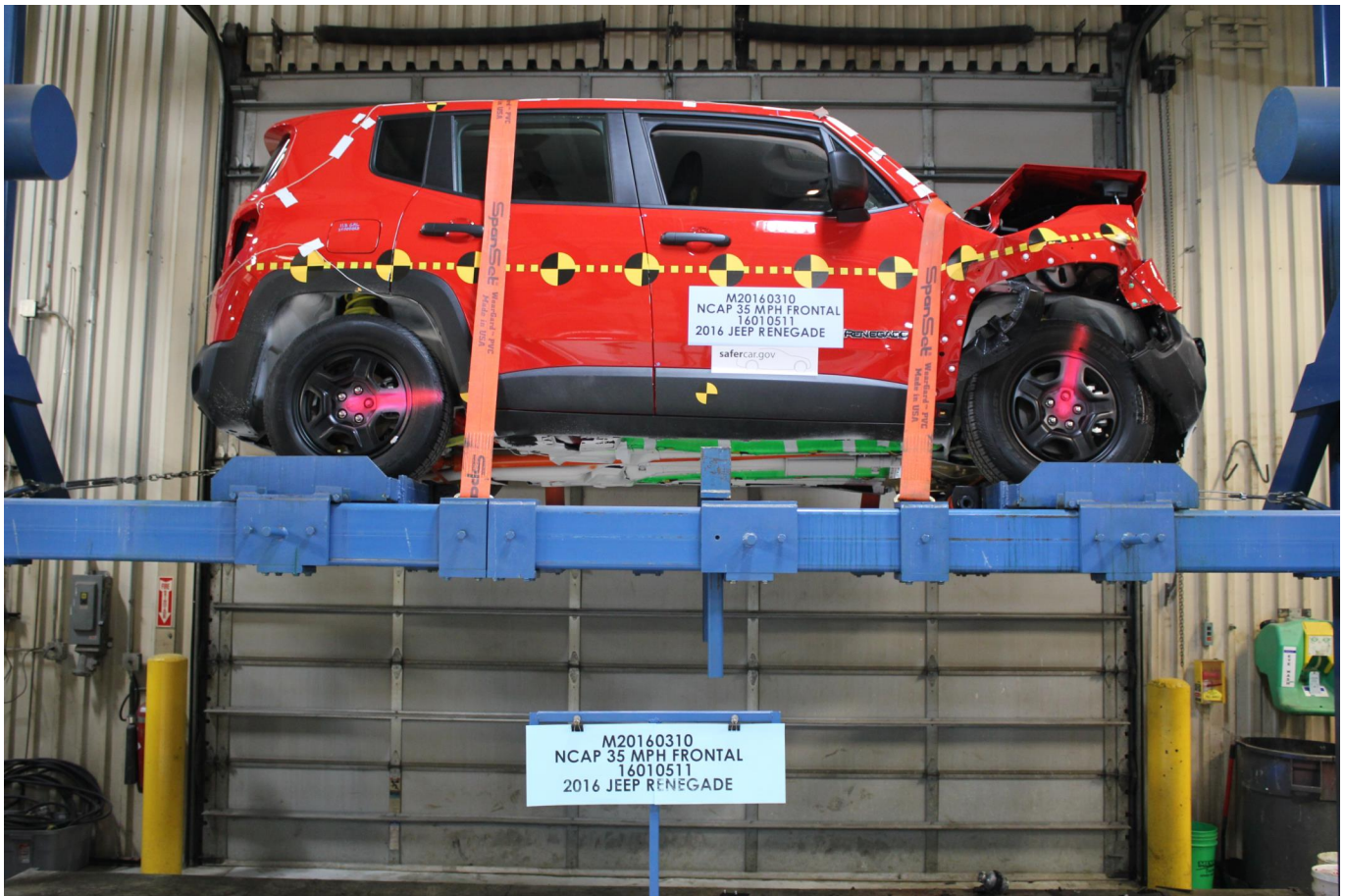
Photo No. 077 - Vehicle at 360 Degrees on Static Rollover Device
