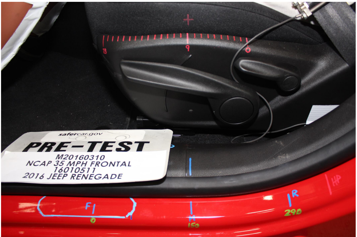
Photo No. 036 - Pre-Test Driver's Seat Fore-Aft Markings
