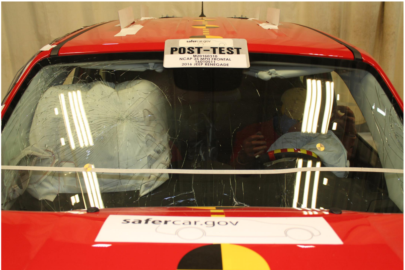
Photo No. 019 - Post-Test Windshield View
