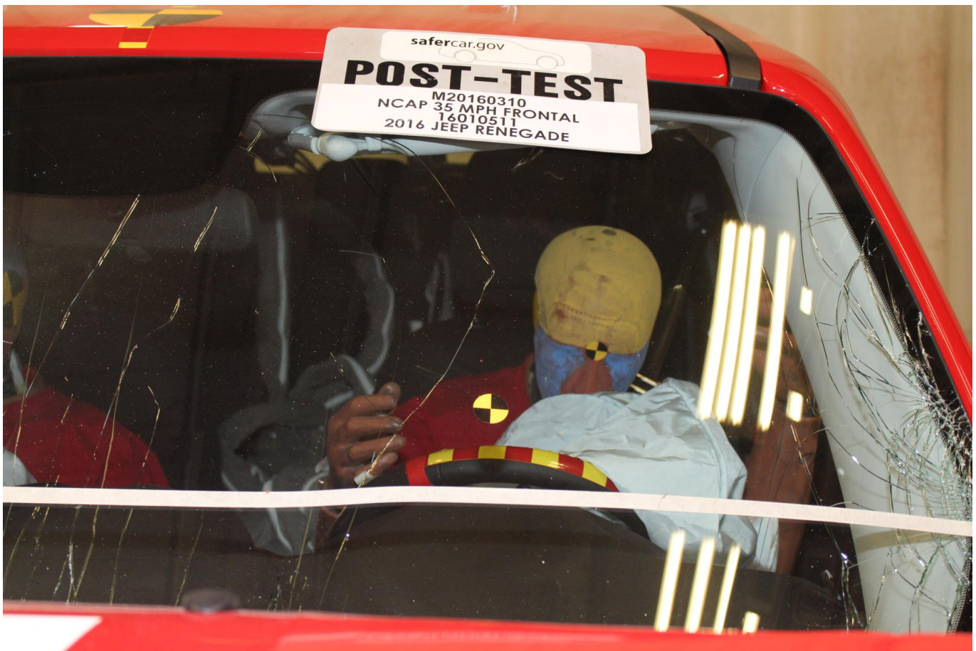
Photo No. 031 - Post-Test Driver Dummy Front View
