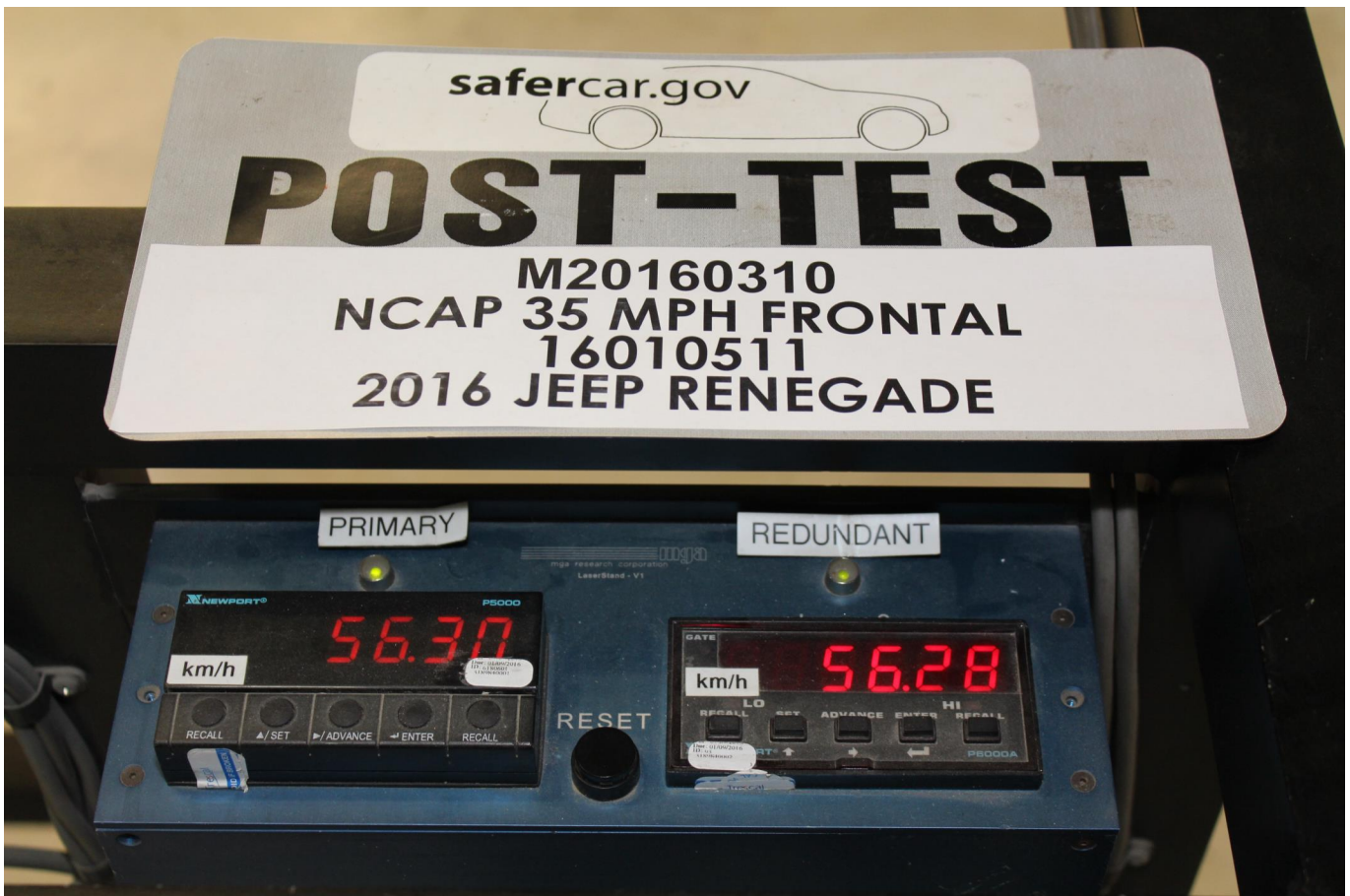
Photo No. 072 - Post-Test Speed Trap Read-Out
