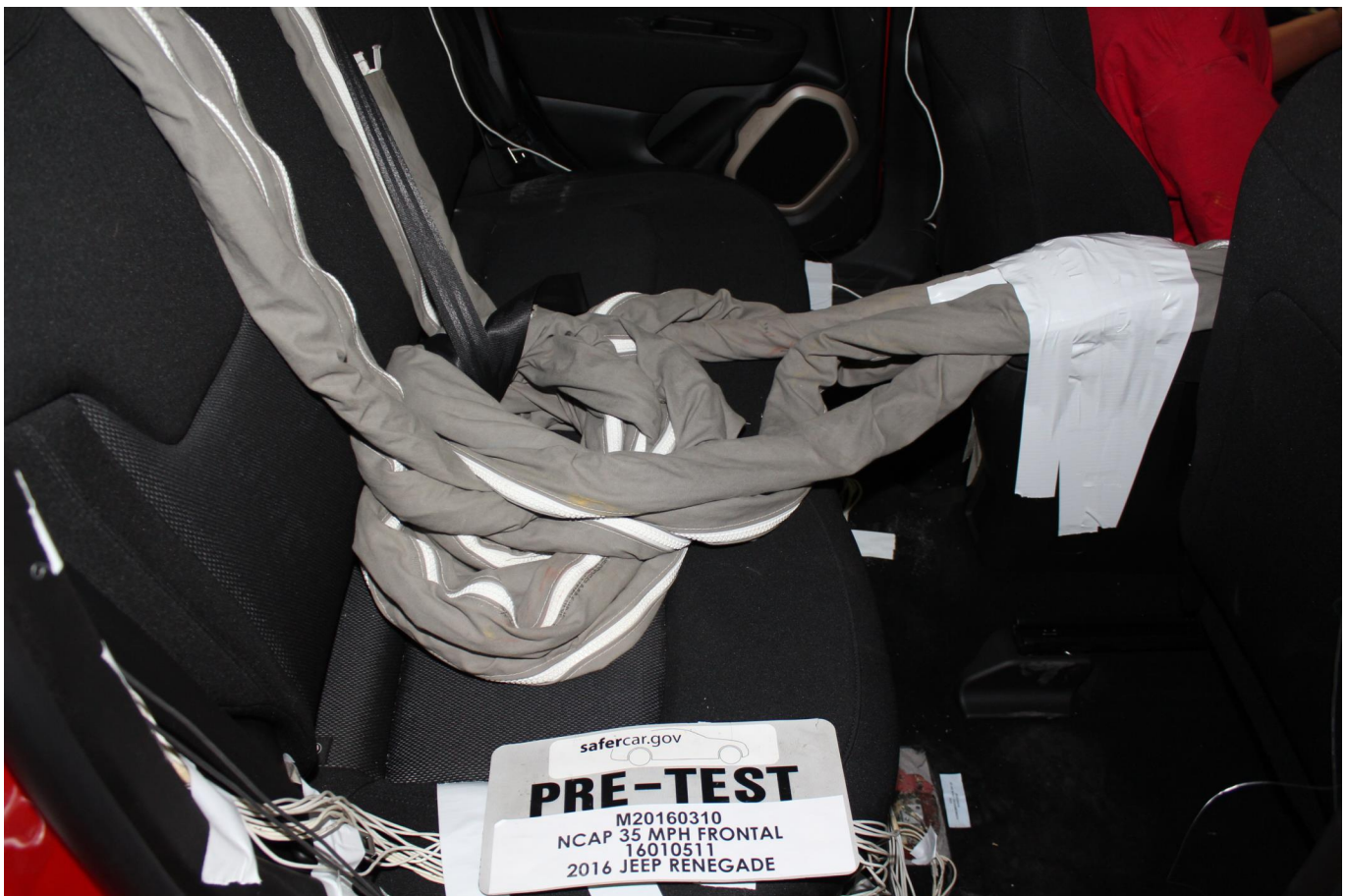
Photo No. 028 - Pre-Test Dummy Cable Routing
