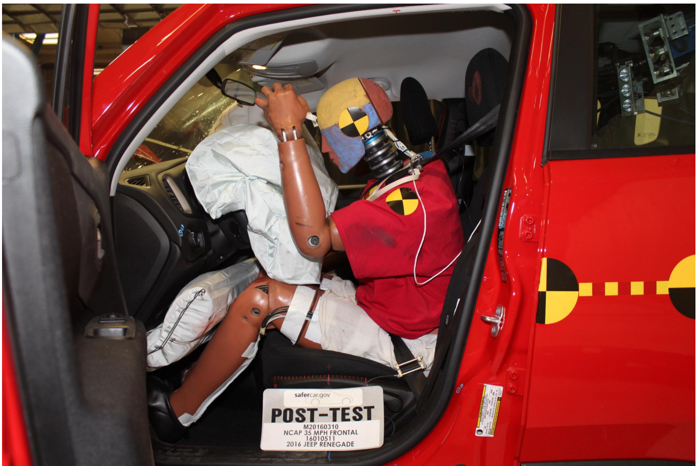
Photo No. 035 - Post-Test Driver Dummy and Vehicle Interior (Door Open)
