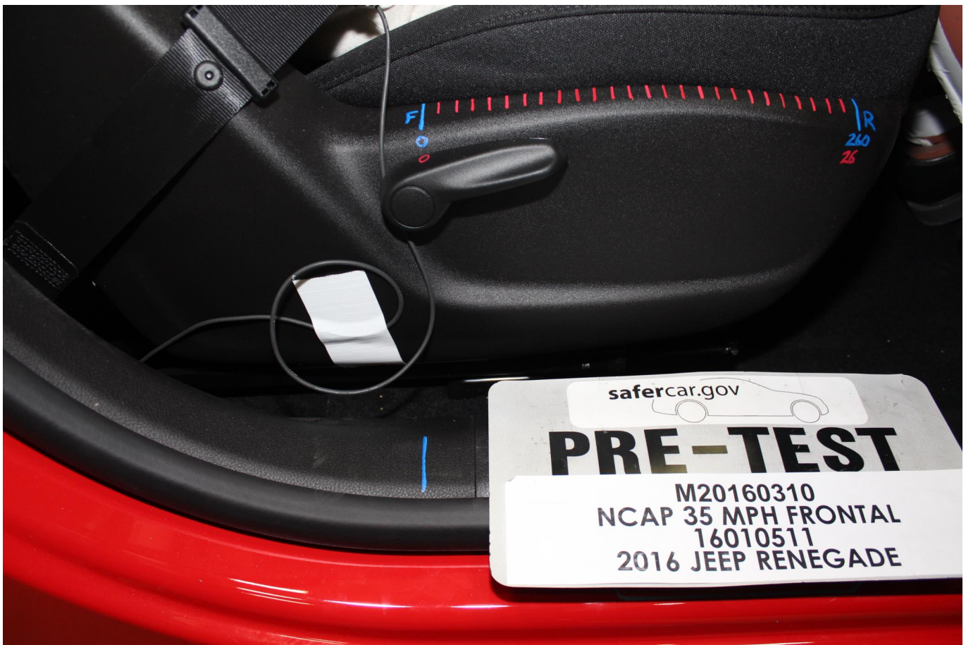
Photo No. 057 - Pre-Test Passenger's Seat Fore-Aft Markings
