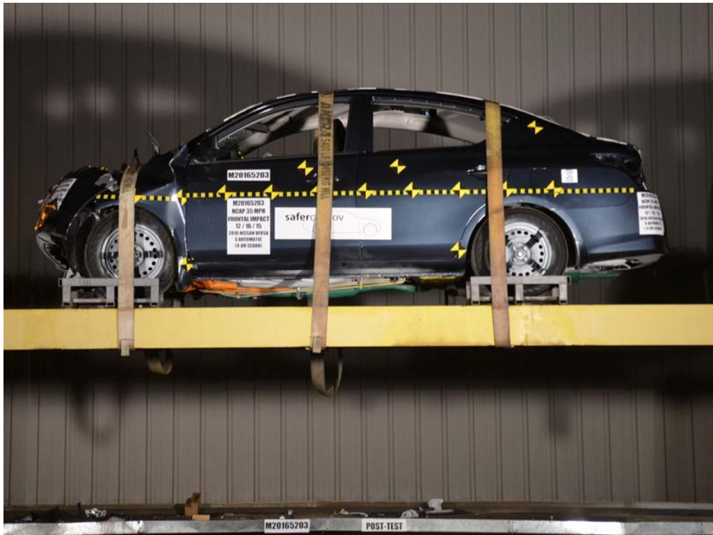
FIGURE 77. Vehicle at 360° on Static Rollover Device
