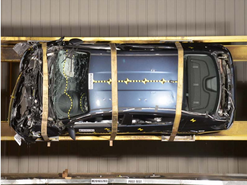
FIGURE 74. Vehicle at 90° on Static Rollover Device
