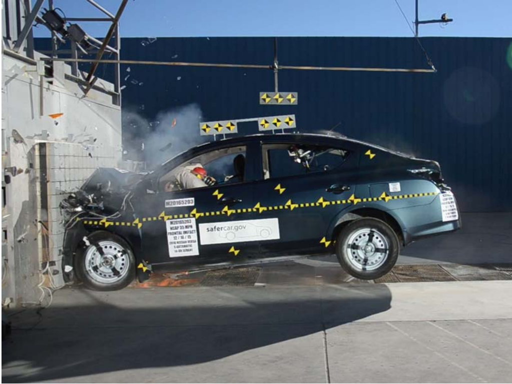
FIGURE 78. 2016 Nissan Versa Frontal Impact Event
