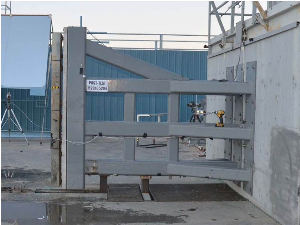
FIGURE 60. Post-Test Pole Barrier Side View
