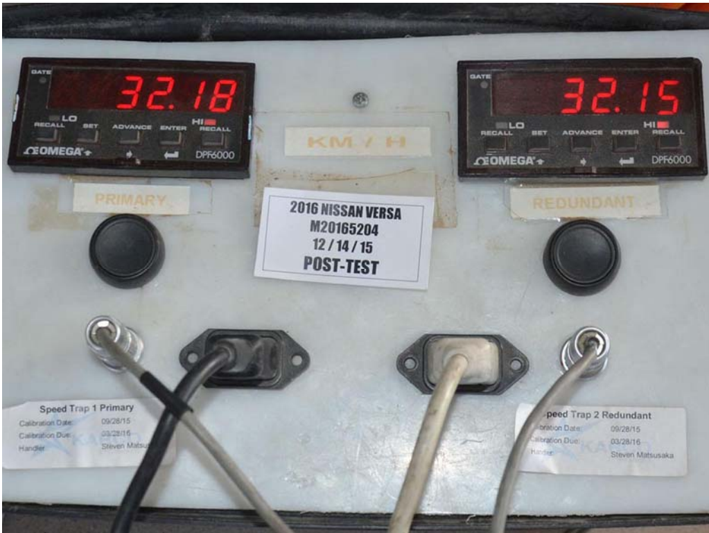
FIGURE 62. Post-Test Primary and Redundant Speed Trap Read-Out
