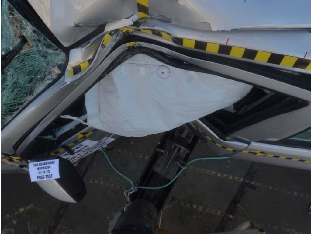
FIGURE 41. Post-Test Dummy and Door Clearance View
