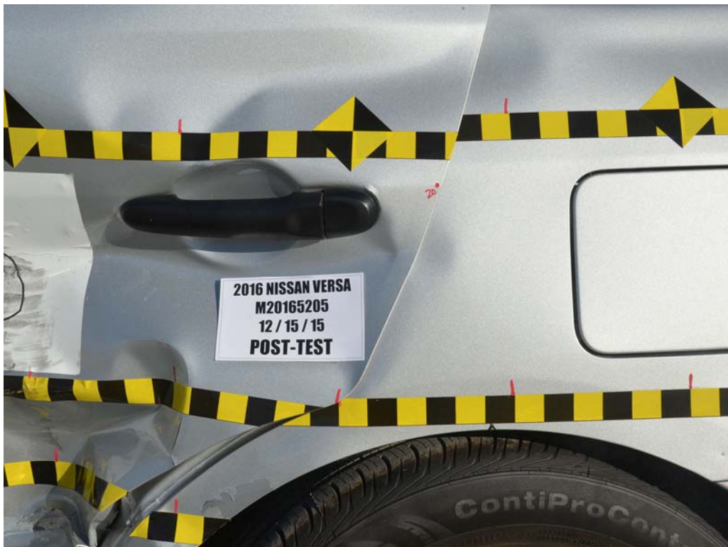
FIGURE 24. Post-Test Left Rear Door Latch Close-Up
