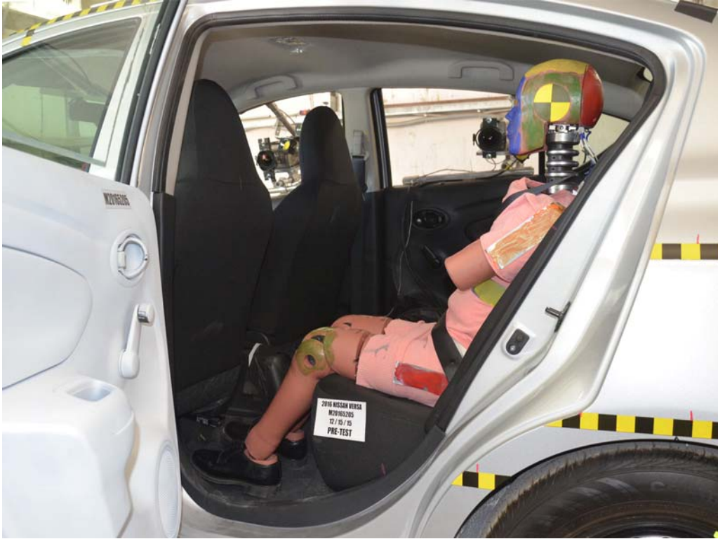
FIGURE 55. Pre-Test Left Side View of Rear Passenger Dummy Showing Belt and Chalking
