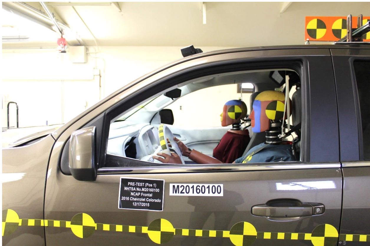
Figure A-31: Pre-Test Driver Dummy Window View
