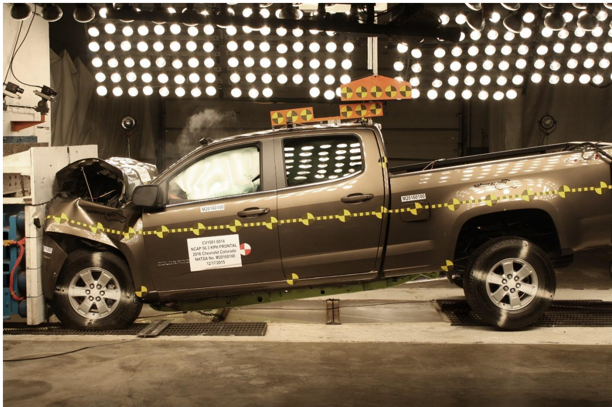
Figure A-77: 2016 Chevrolet Colorado Crew Cab Frontal Impact Event
