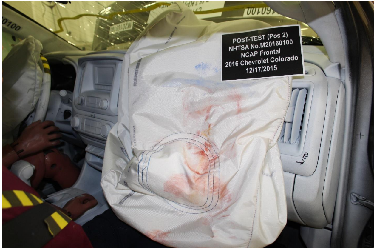
Figure A-67: Post-Test Passenger Dummy Contact With Airbag
