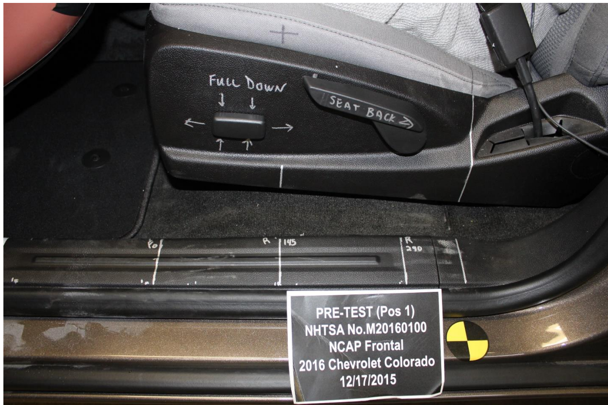
Figure A-35: Pre-Test Driver's Seat Fore-Aft Markings
