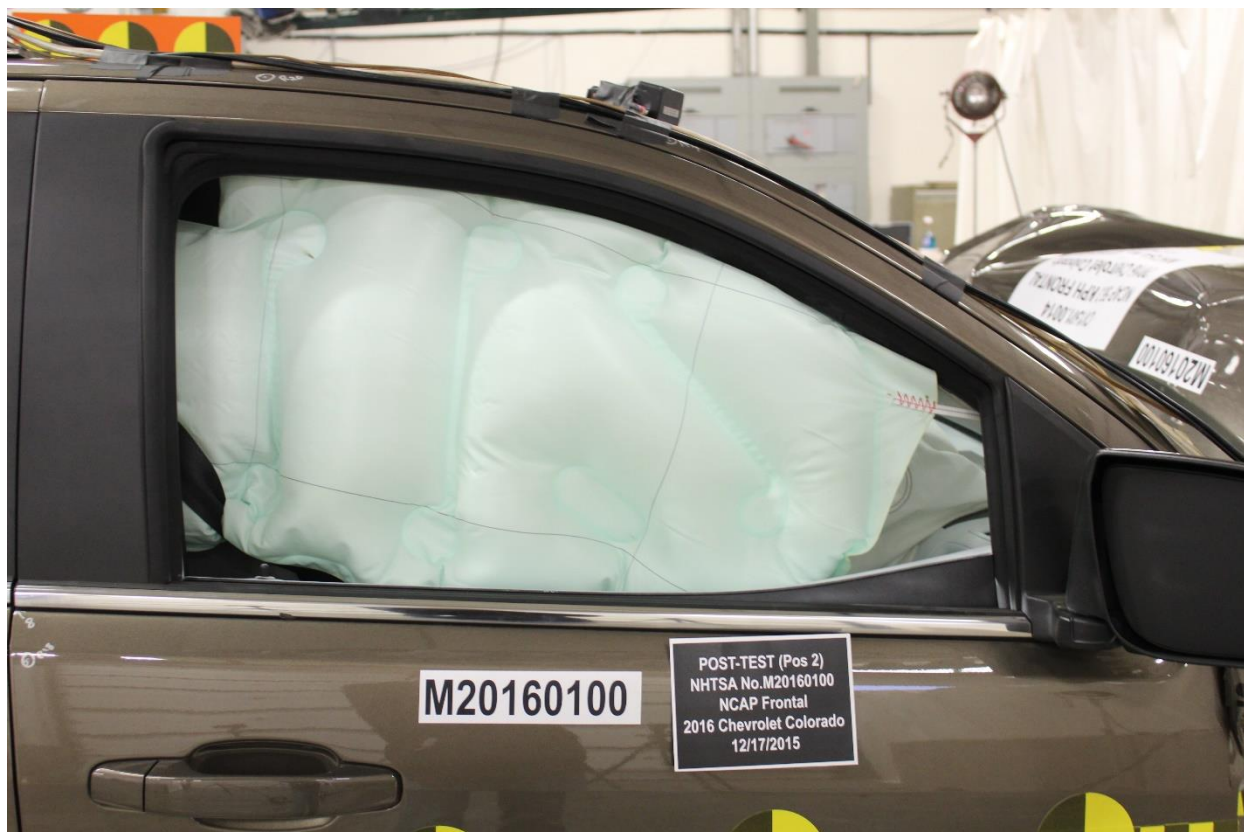
Figure A-53: Post-Test Passenger Dummy Window View
