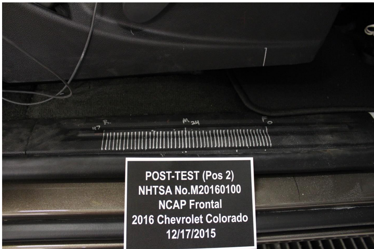
Figure A-57: Post-Test Passenger's Seat Fore-Aft Markings
