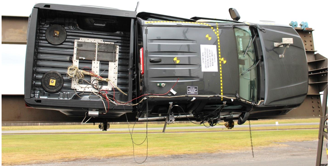
Figure A-99: FMVSS No. 301 Static Rollover 270 Degrees
