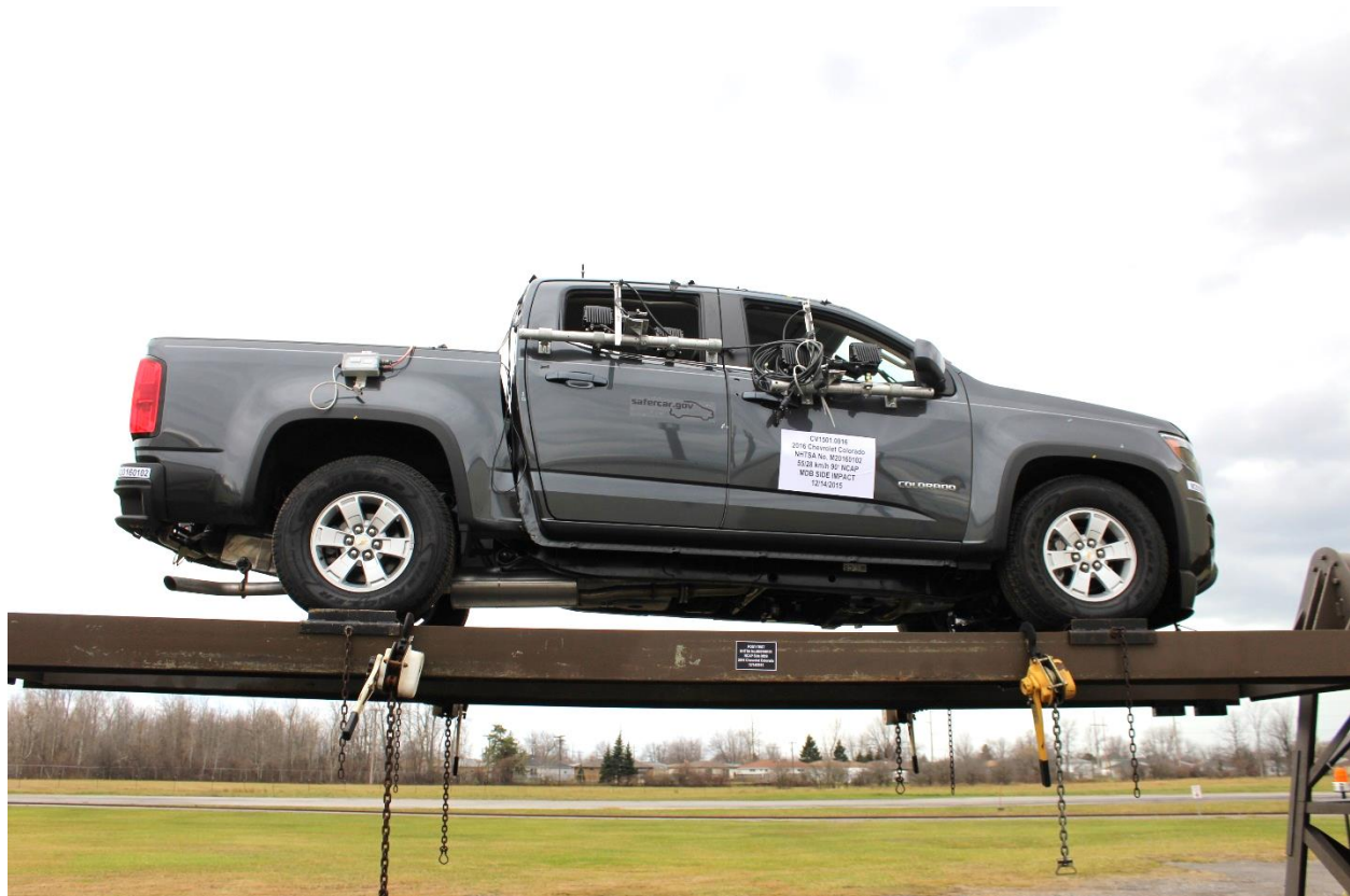
Figure A-96: FMVSS No. 301 Static Rollover 0 Degrees
