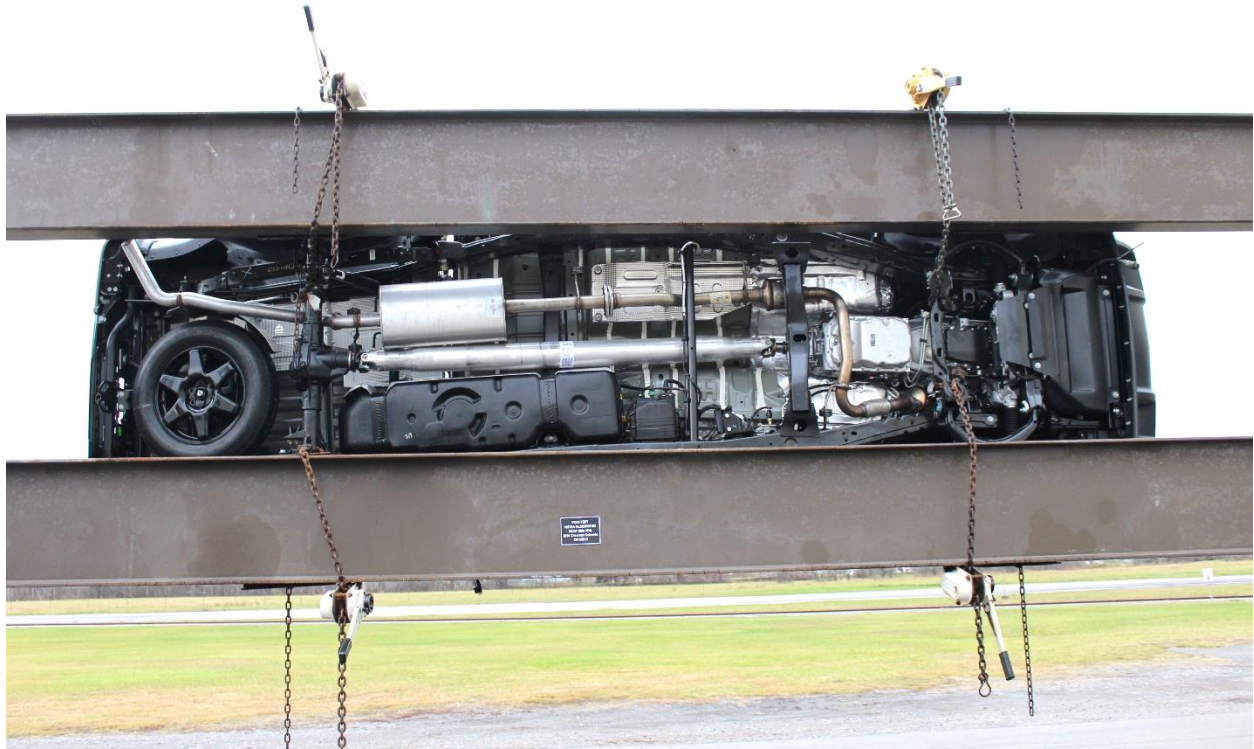
Figure A-97: FMVSS No. 301 Static Rollover 90 Degrees
