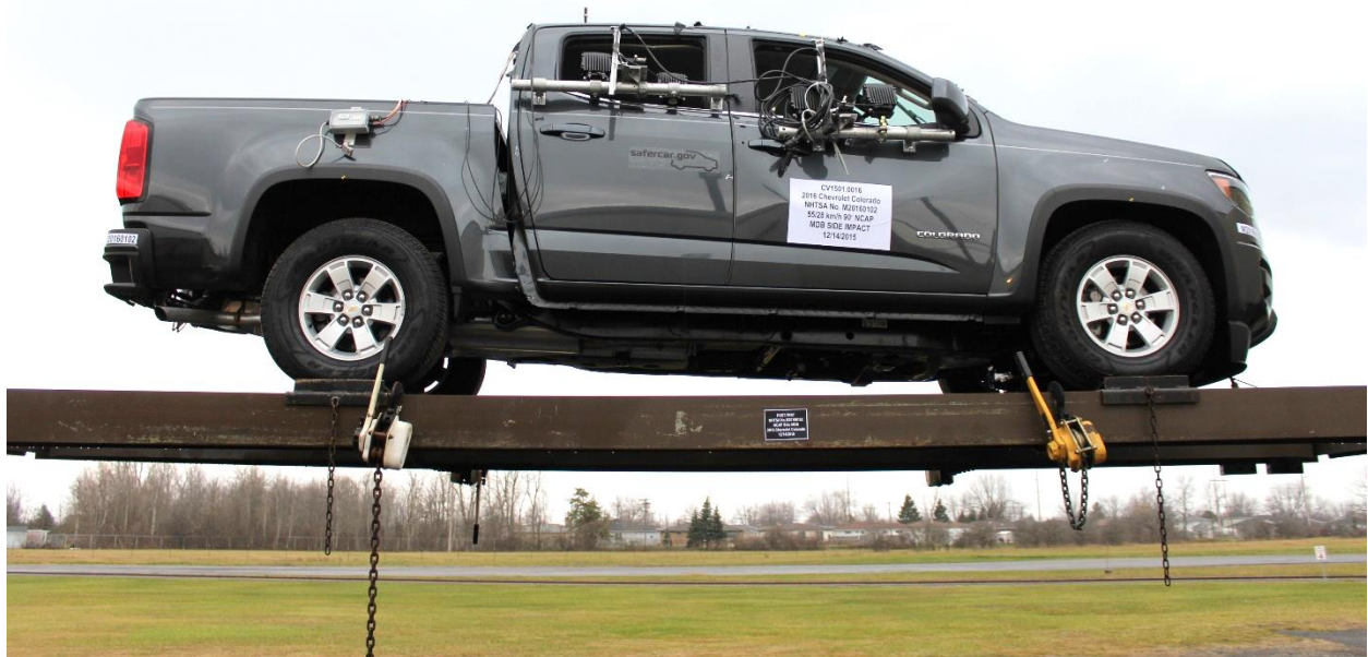
Figure A-100: FMVSS No. 301 Static Rollover 360 Degrees
