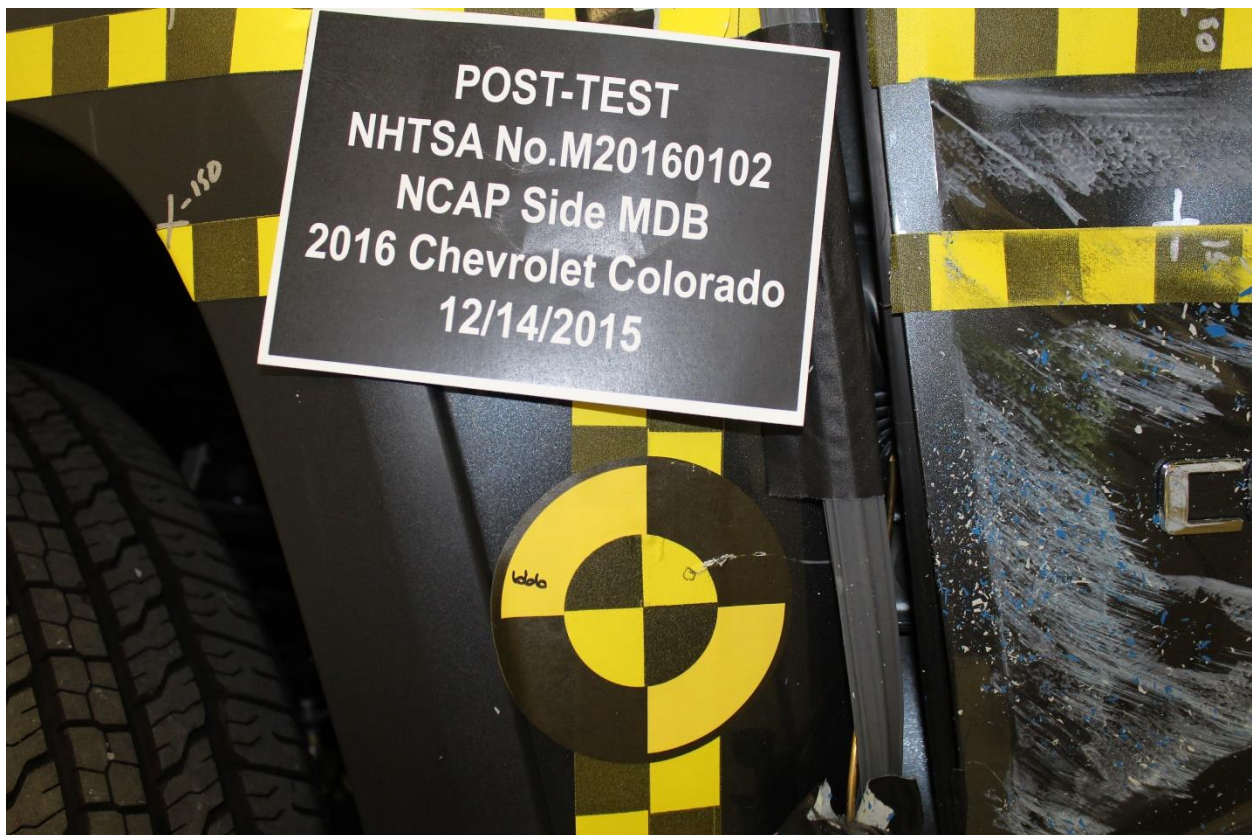
Figure A-20: Post-Test Close-up View of Impact Point Target
