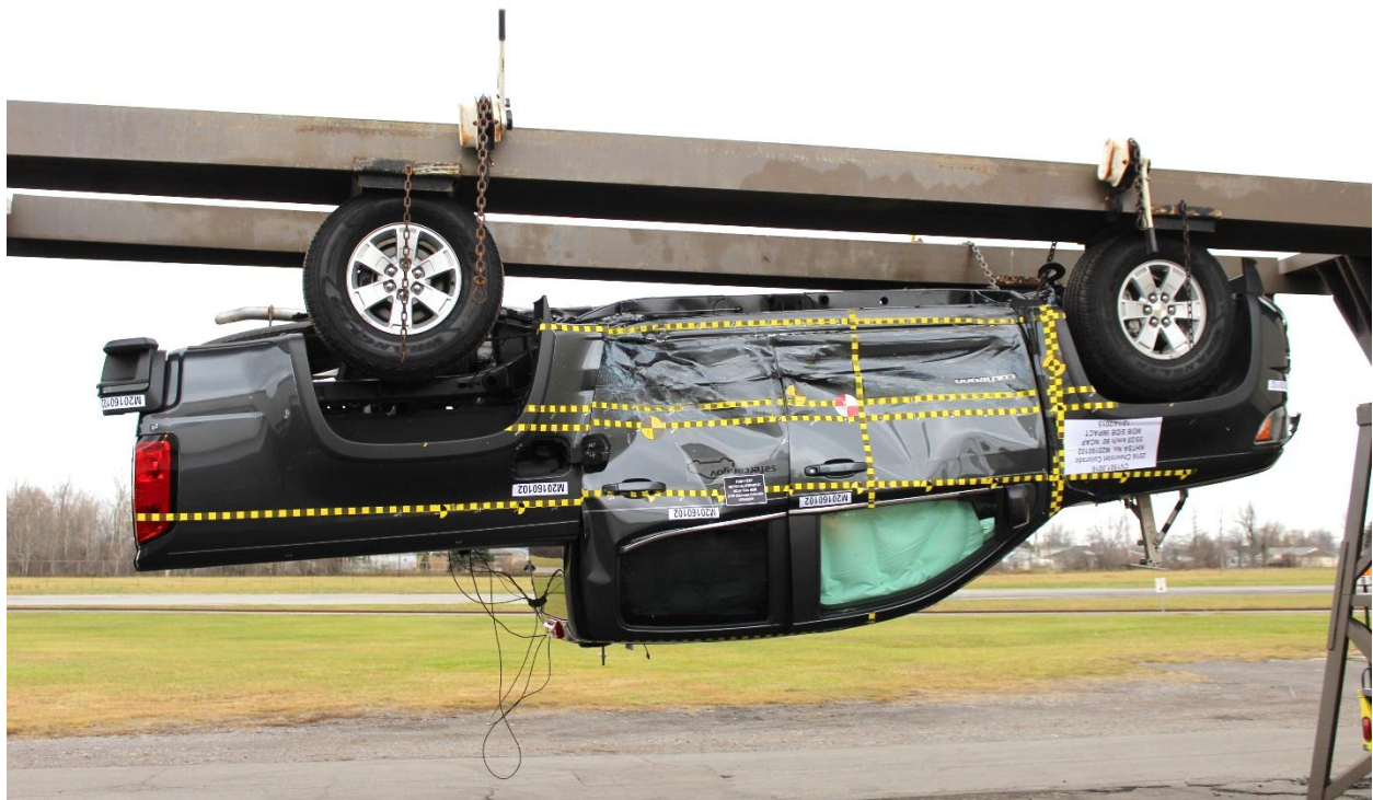
Figure A-98: FMVSS No. 301 Static Rollover 180 Degrees
