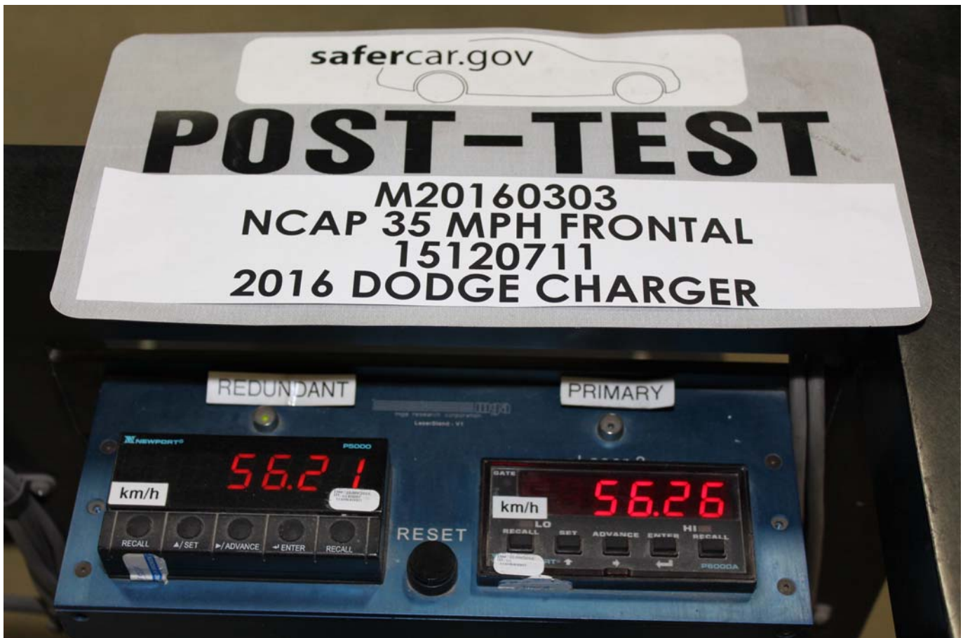
Photo No. 072 - Post-Test Speed Trap Read-Out
