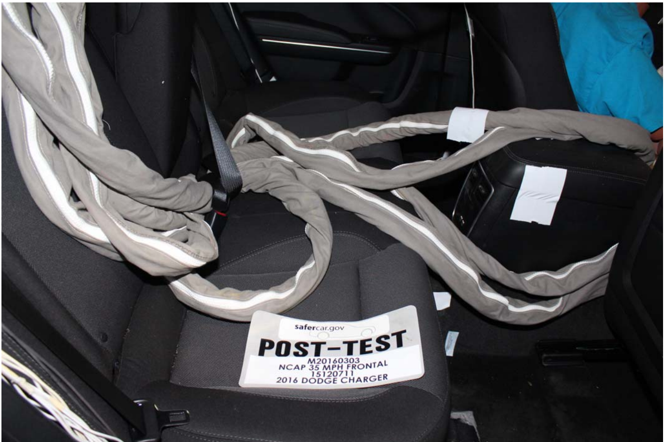
Photo No. 029 - Post-Test Dummy Cable Routing
