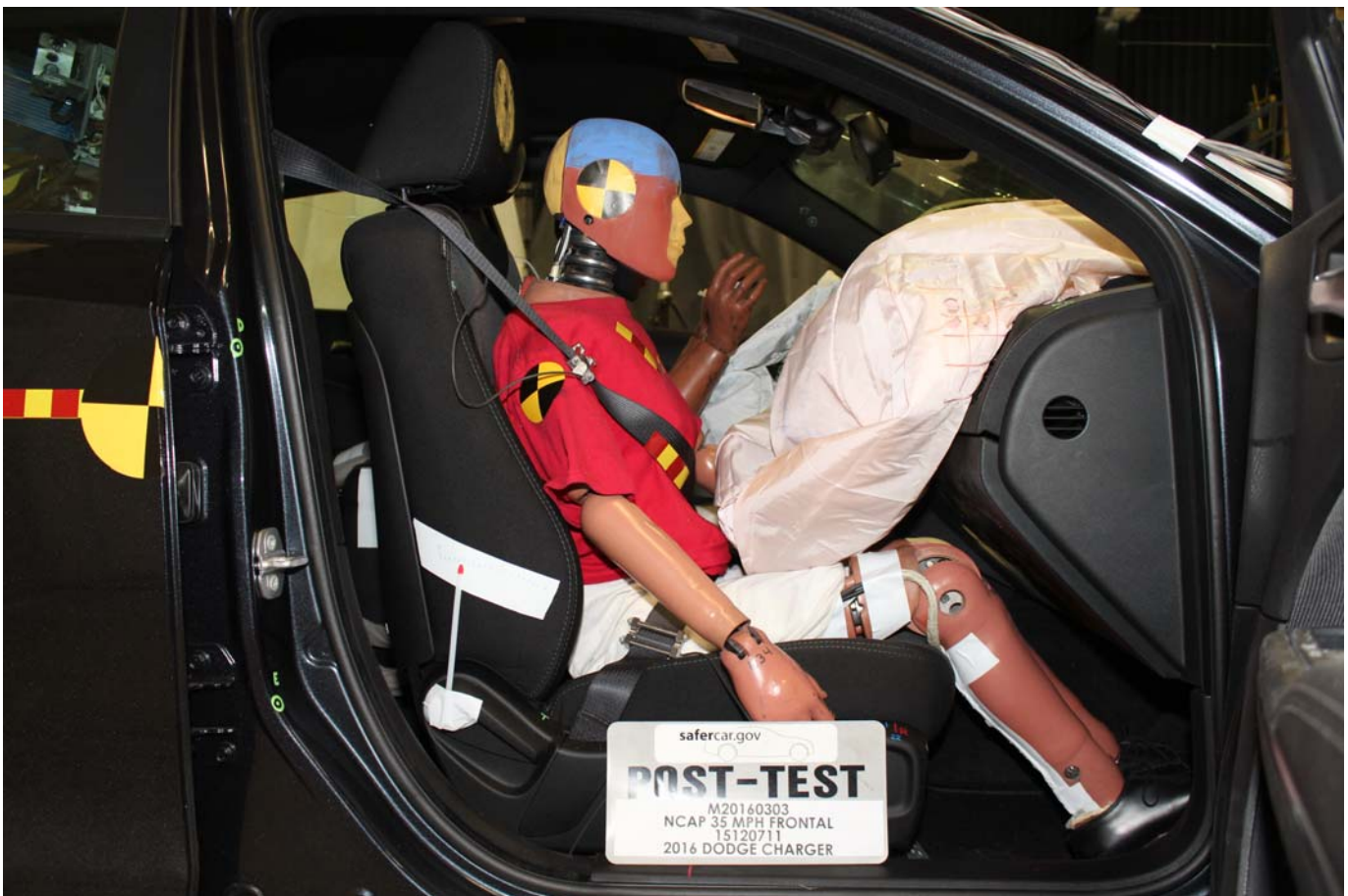
Photo No. 056 - Post-Test Passenger Dummy and Vehicle Interior (Door Open)
