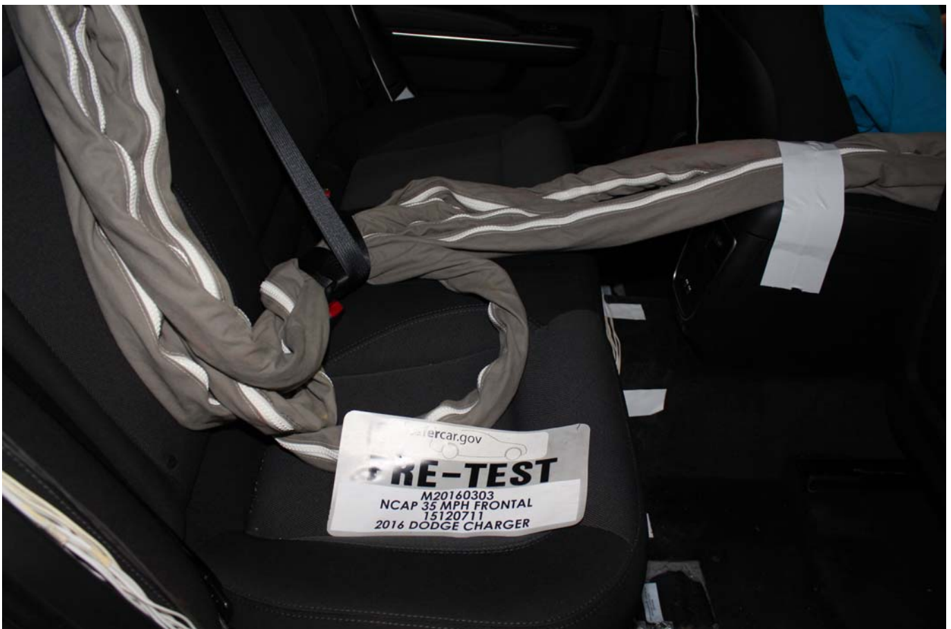
Photo No. 028 - Pre-Test Dummy Cable Routing
