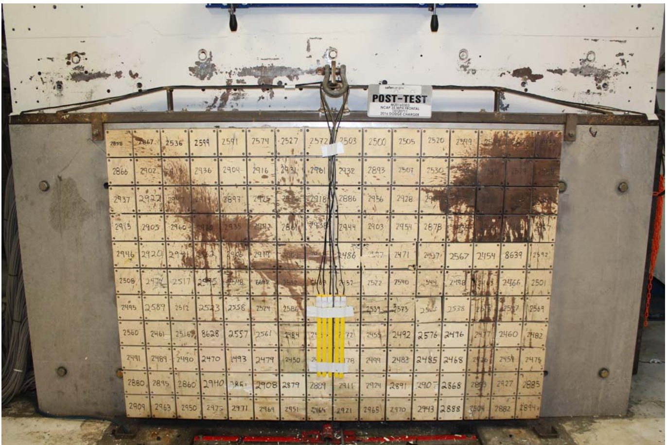
Photo No. 003 - Post-Test Load Cell Wall
