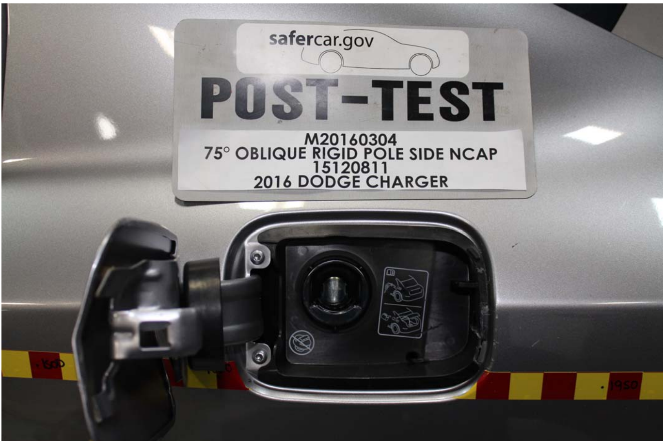
Photo No. 054 - Post-Test View of Fuel Filler Cap or Fuel Filler Neck
