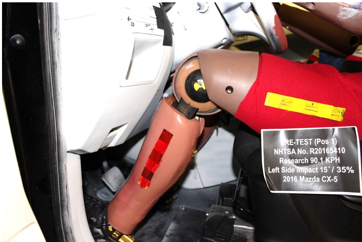
No. 071 Pre-Test View of Driver Left Knee and Bolster
