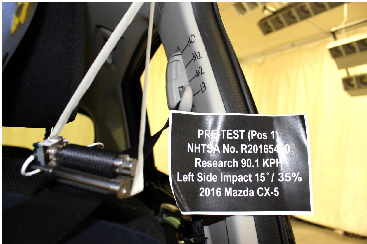
No. 065 Pre-Test Driver Adjustable D-Ring
