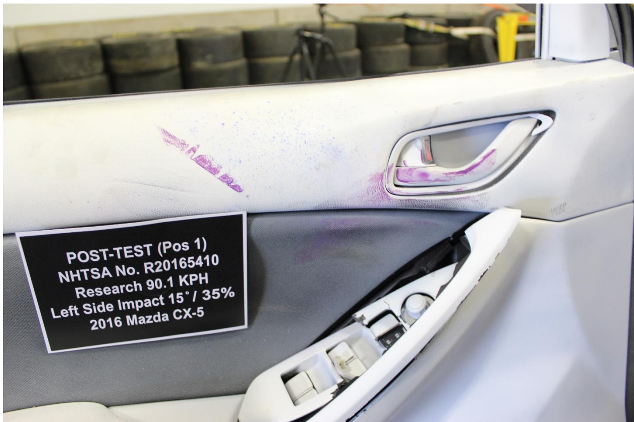
No. 080: Post-Test View of Driver Body Contact with Vehicle Interior - B
