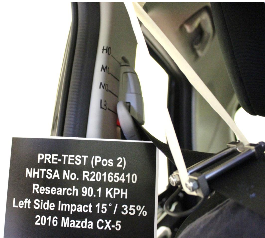
No. 108: Pre-Test Passenger Adjustable D-ring
