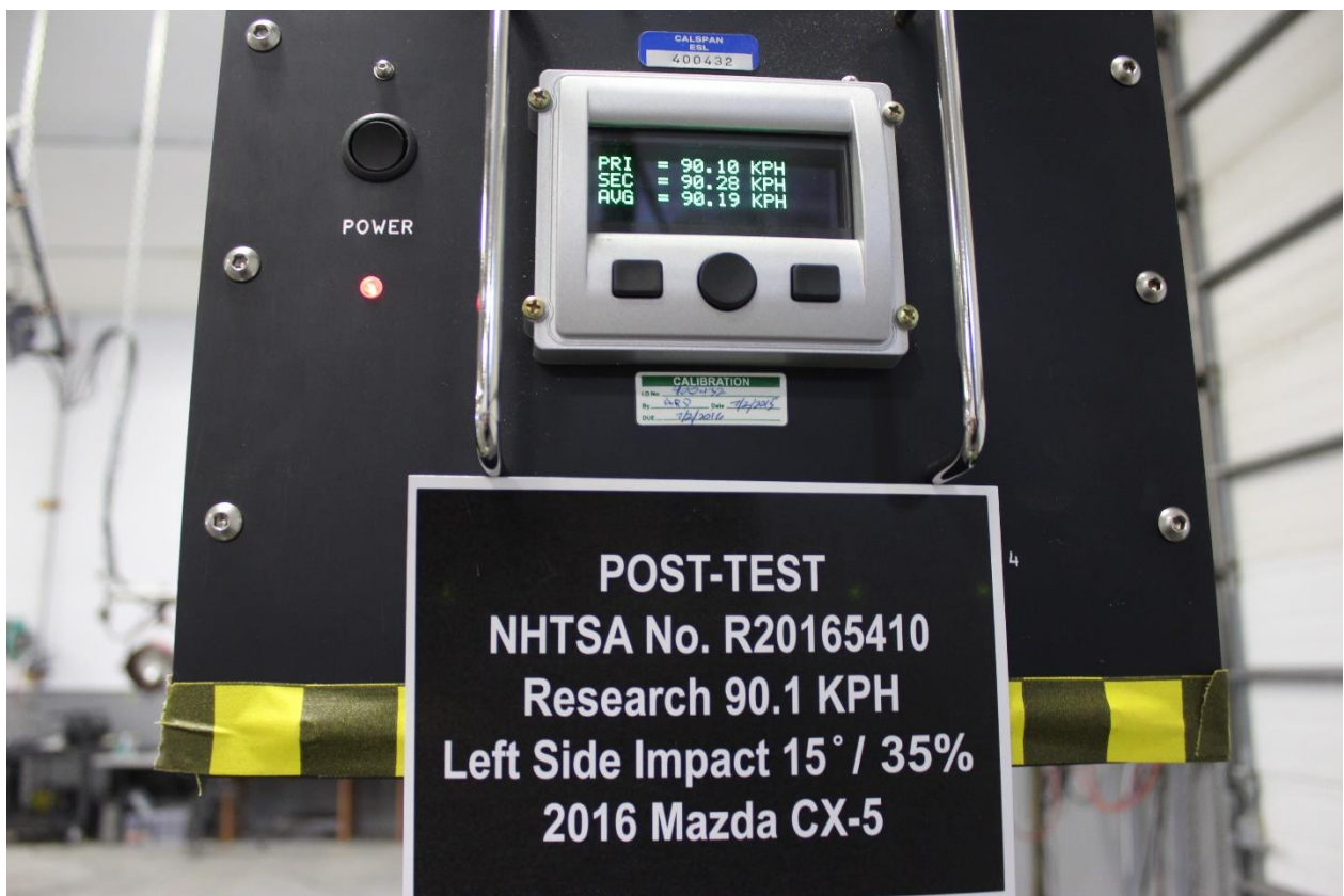
No. 125: Post-Test Speed Trap Readout
