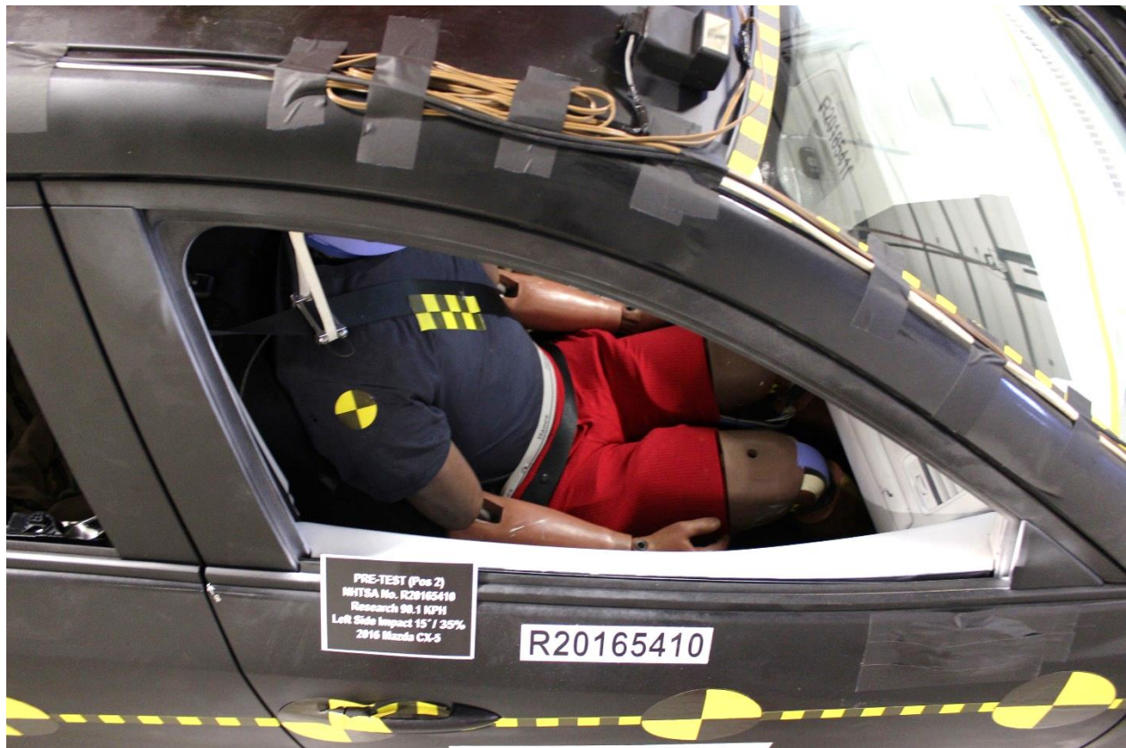
No. 102: Pre-Test View of Passenger Door Clearance
