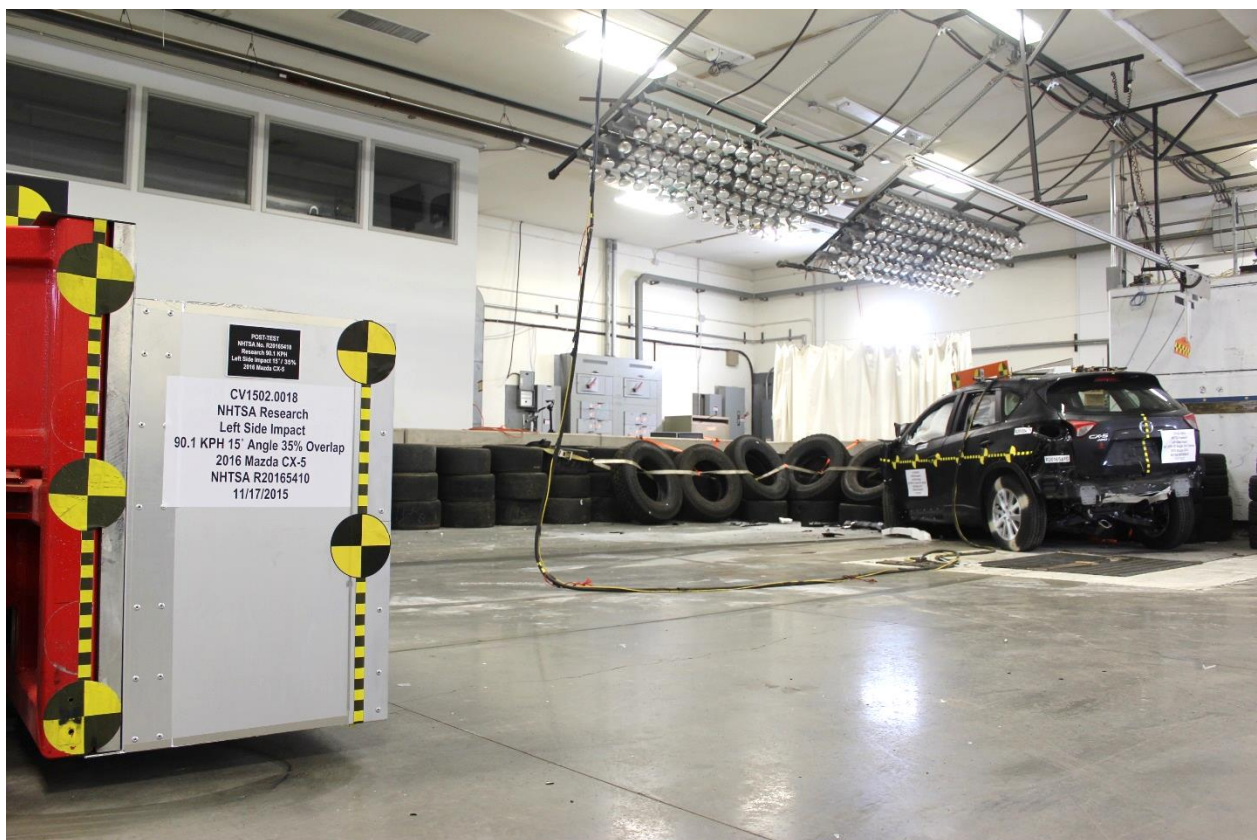
No. 184: Post-Test OMDB & Vehicle, Right Side
