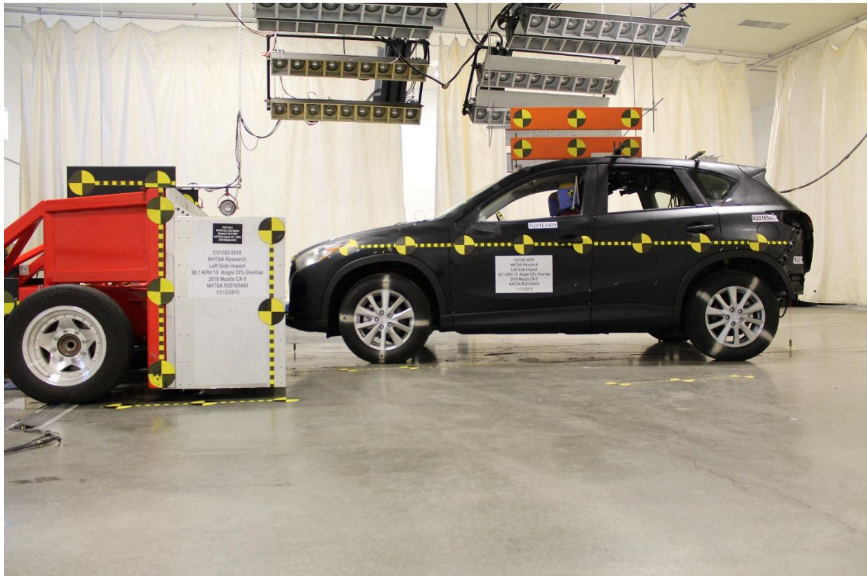
No. 183: Pre-Test OMDB & Vehicle, Right Side
