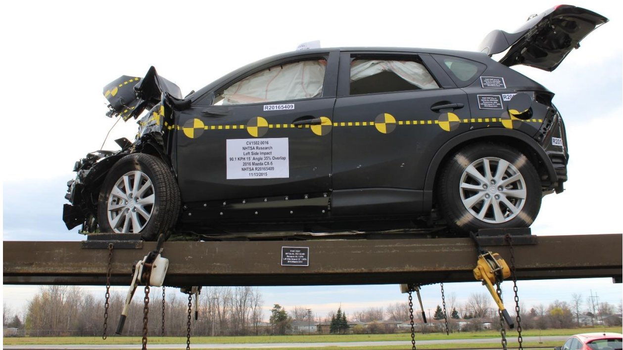
No. 194: Vehicle at 0 Degrees on Static Rollover Device
