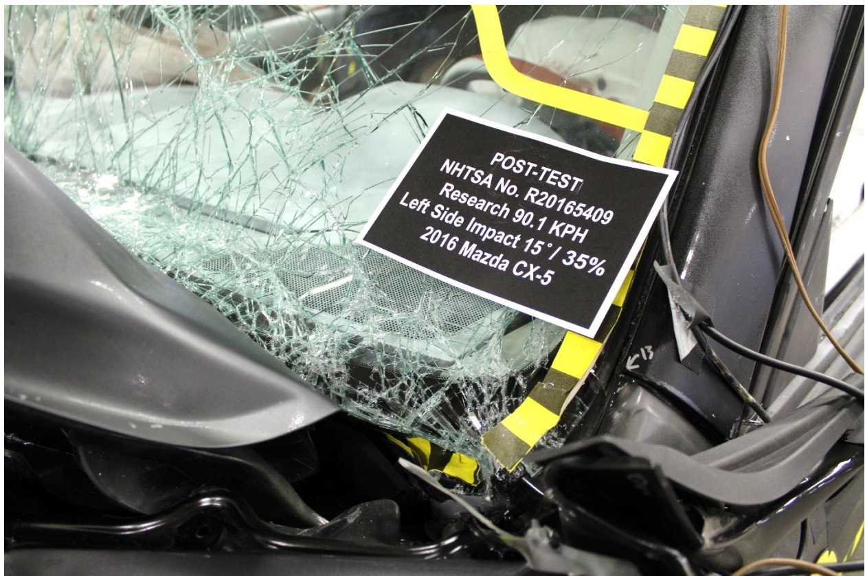
No. 166: Post-Test View of Windshield Separation
