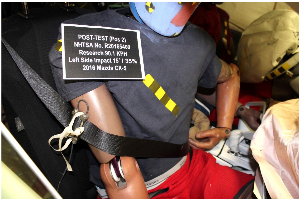
No. 117: Post-Test View of Passenger Abdomen
