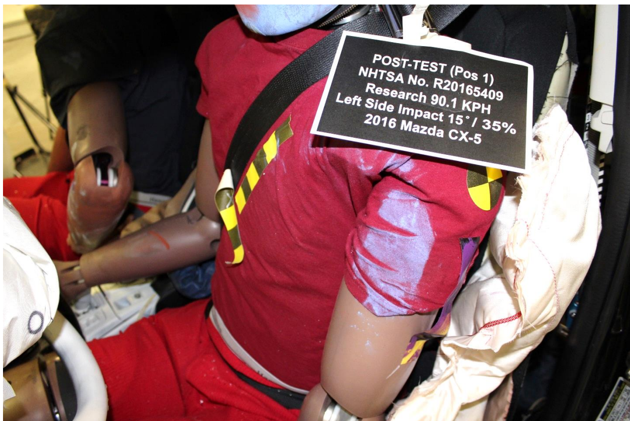
No. 074 Post-Test View of Driver Abdomen
