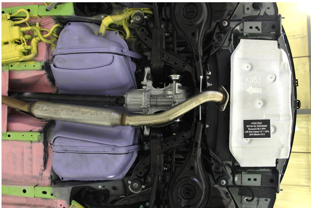
No. 139: Post-Test View of Rear Underbody (perpendicular to vehicle)
