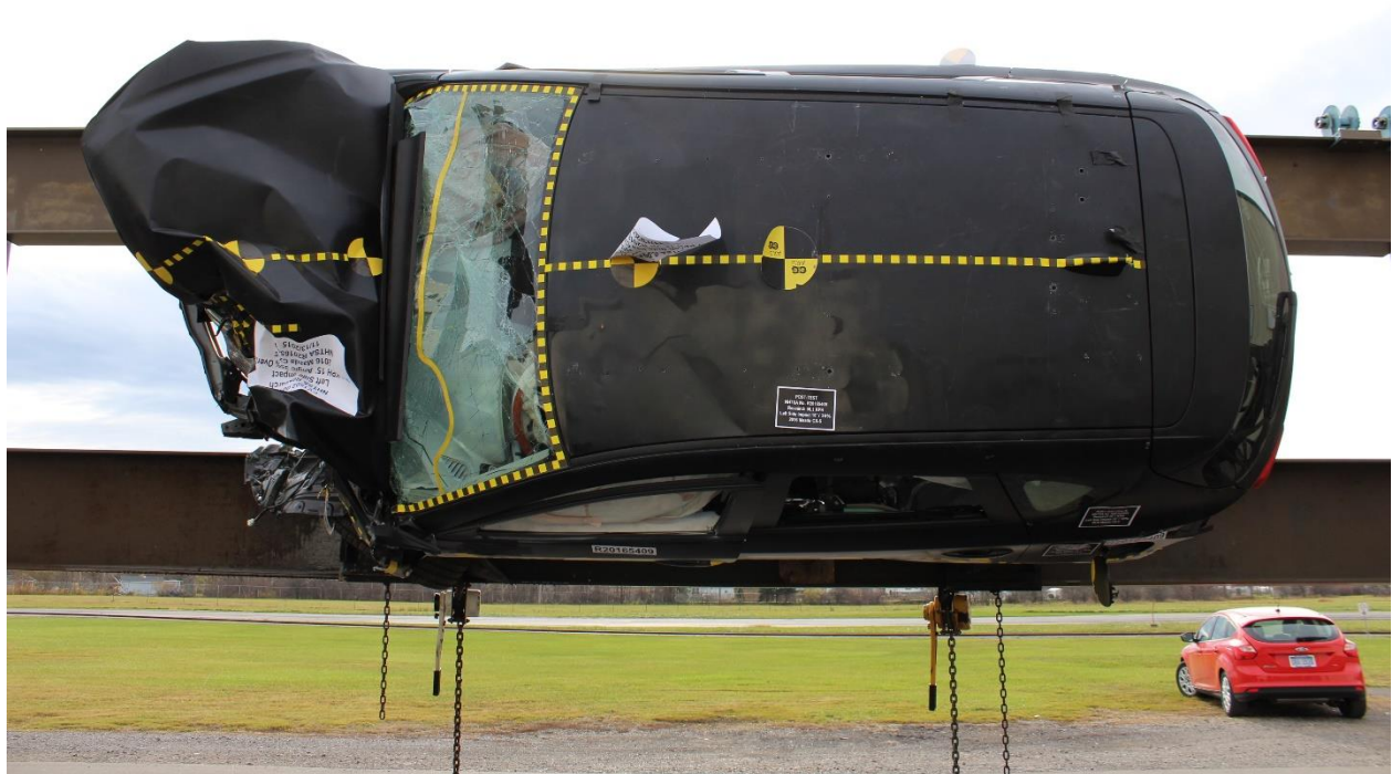
No. 195: Vehicle at 90 Degrees on Static Rollover Device
