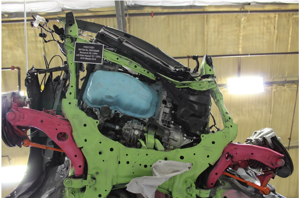
No. 144: Post-Test View of Front Sub-Frame Deformation
