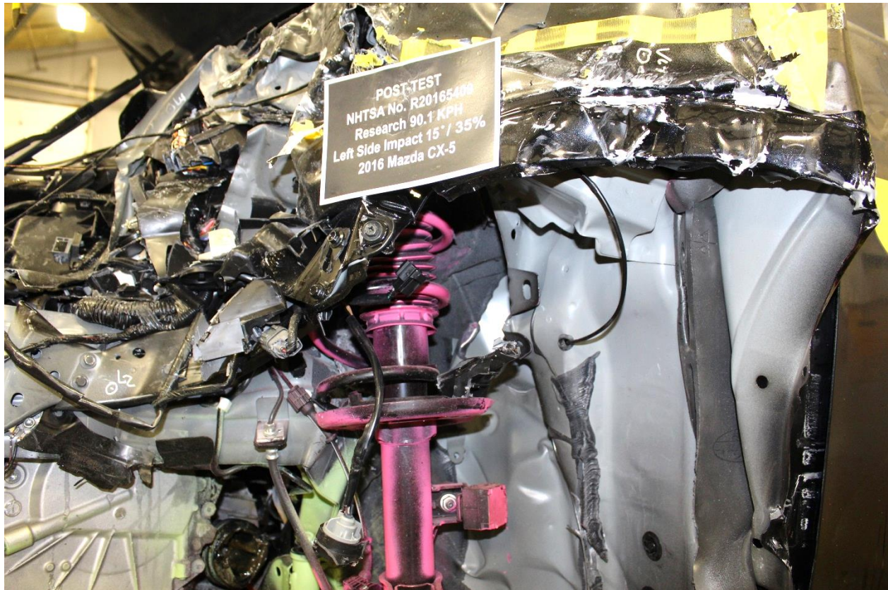
No. 153: Post-Test Front Driver Close up View of Suspension w/ Tire Removed
