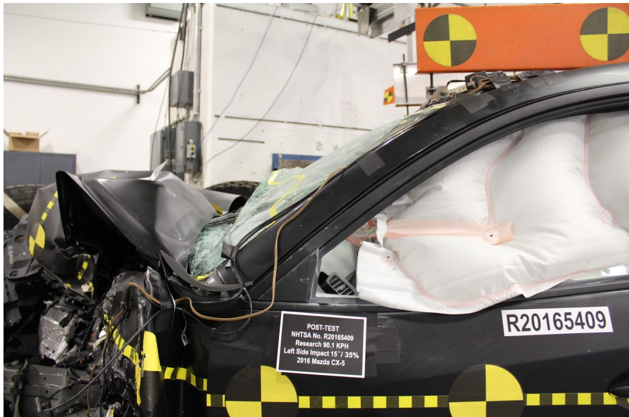
No. 161: Post-Test View of Deformation of A pillar-Struck Side
