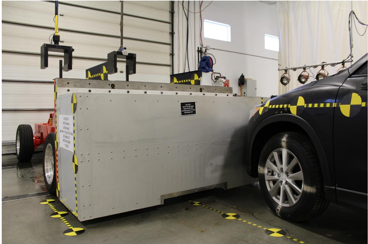
No. 193: Pre-Test OMDB & Vehicle Alignment
