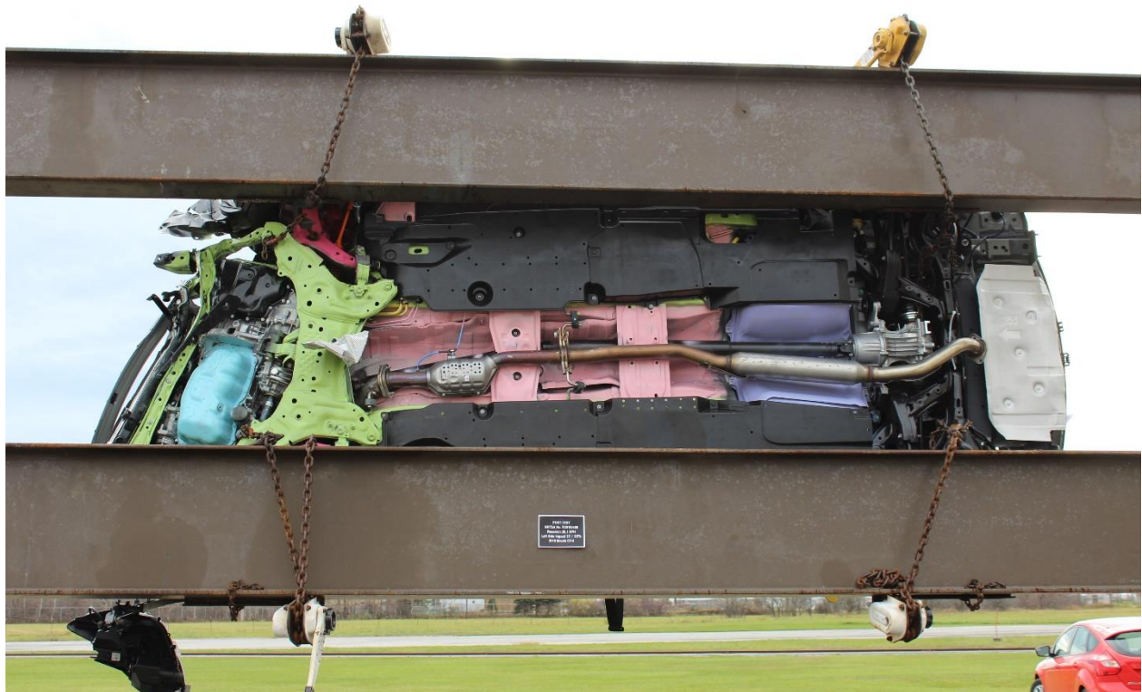
No. 197: Vehicle at 270 Degrees on Static Rollover Device
