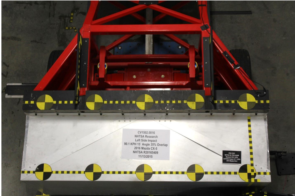
No. 171: Pre-Test Top View of OMDB
