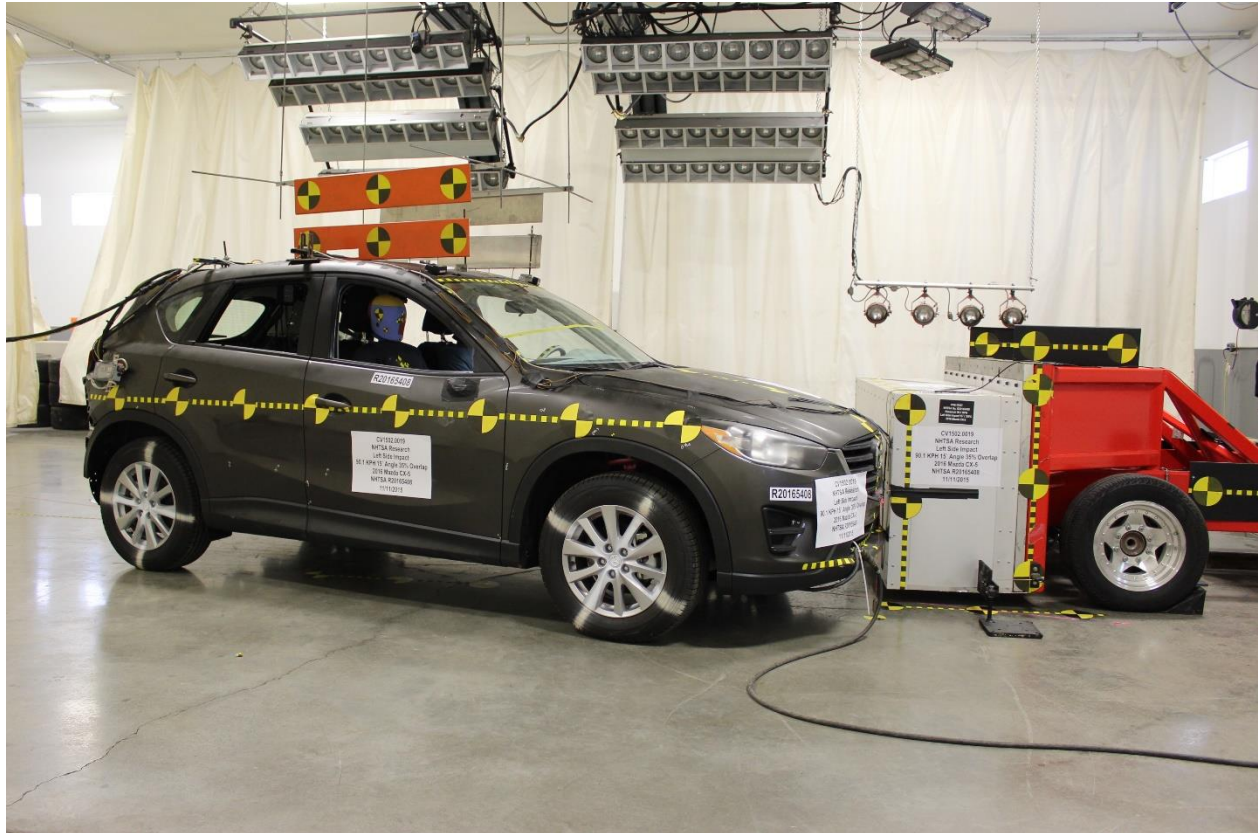
No. 185: Pre-Test OMDB & Vehicle, Left Side
