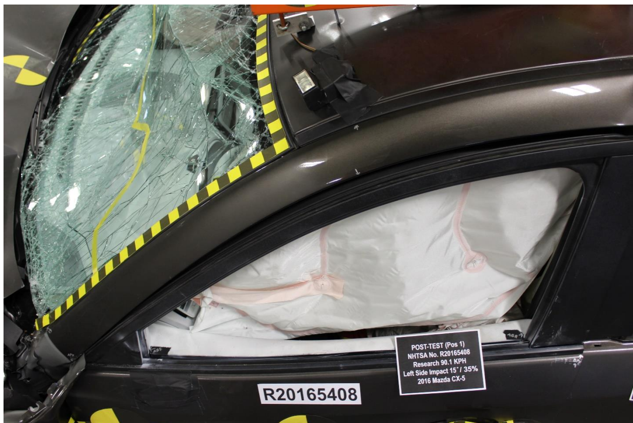
No. 059 Post-Test View of Driver Door Clearance
