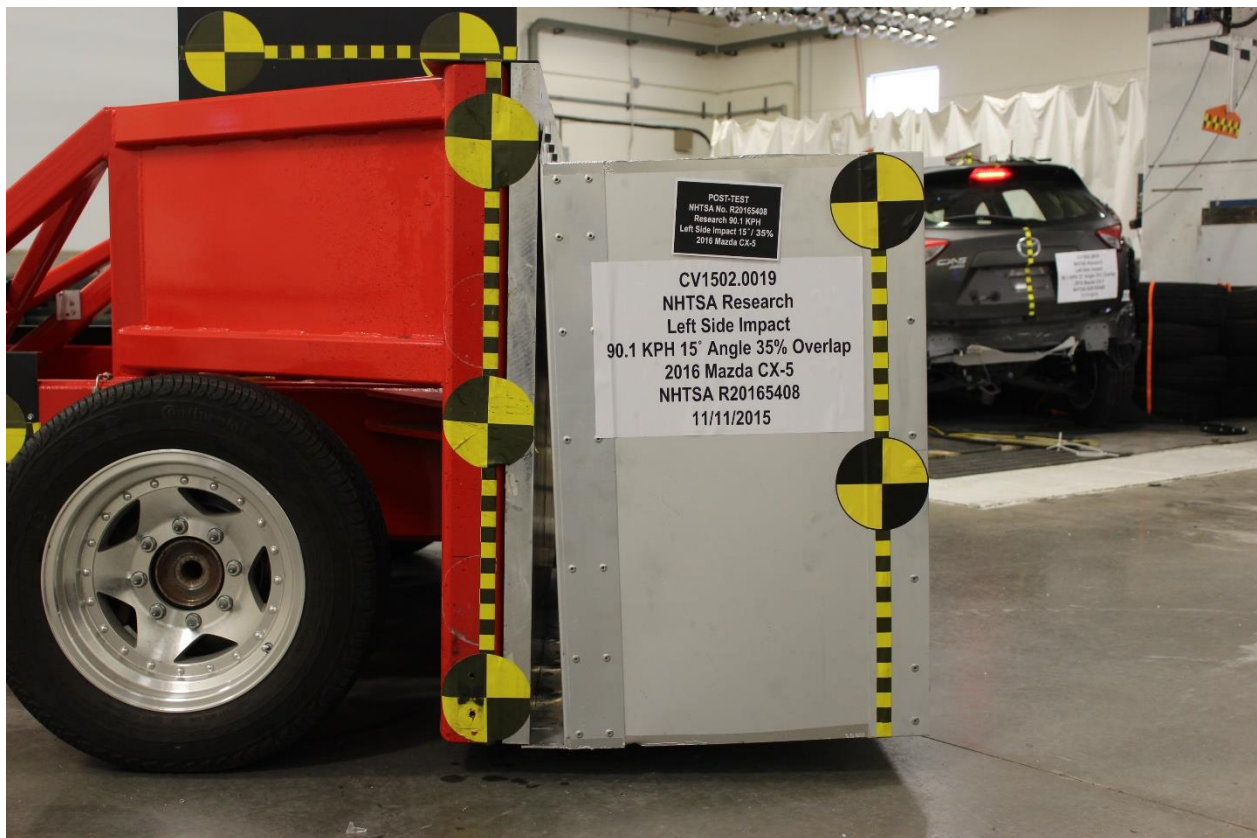
No. 170: Post-Test Right Side View of O MDB
