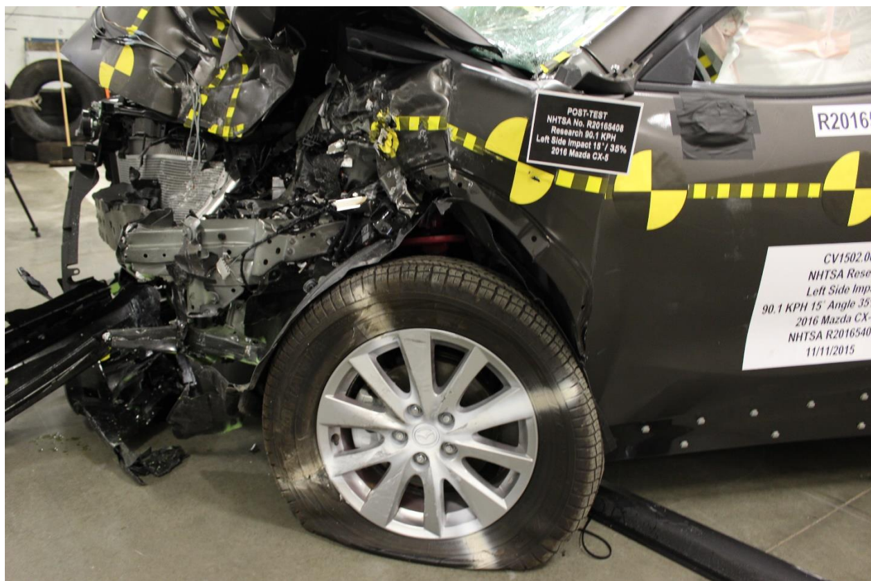
No. 164: Post-Test View of Wheel and/or Tire Deformation-Struck Side
