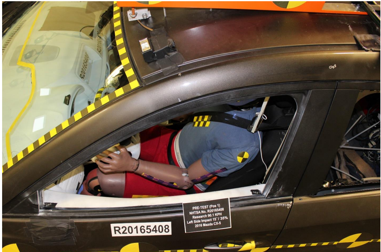
No. 058 Pre-Test View of Driver Door Clearance
