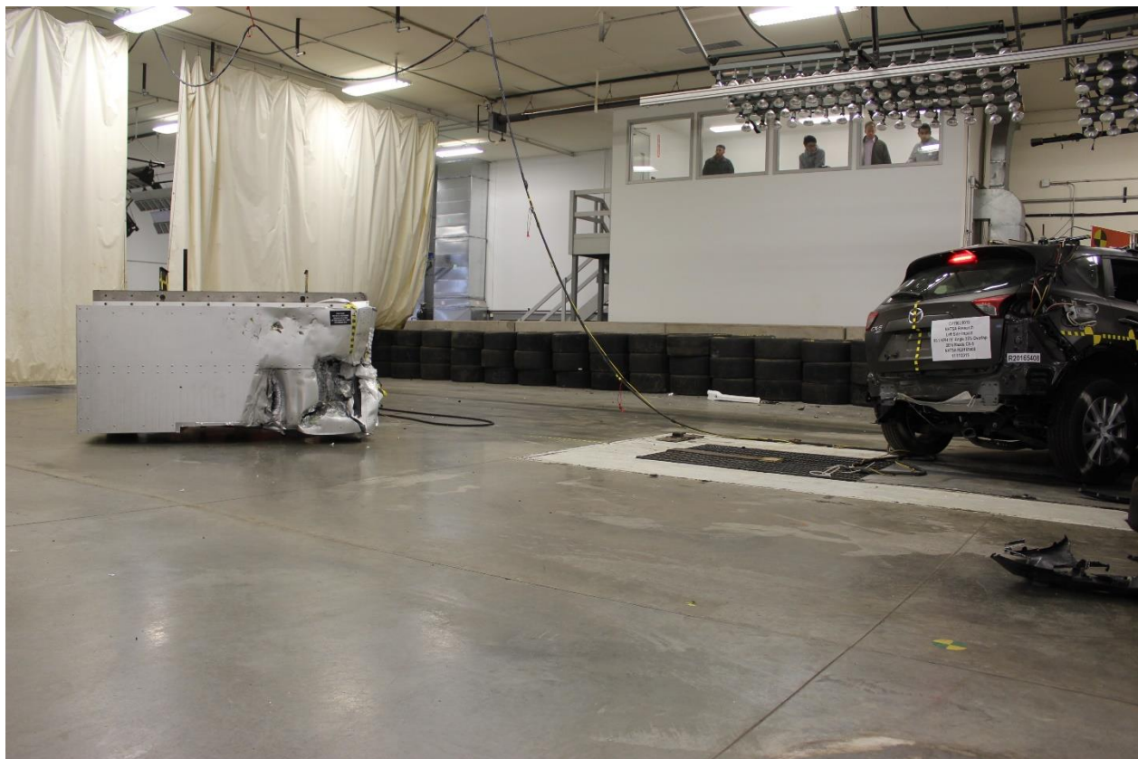
No. 192: Post-Test OMDB & Vehicle, Front View
