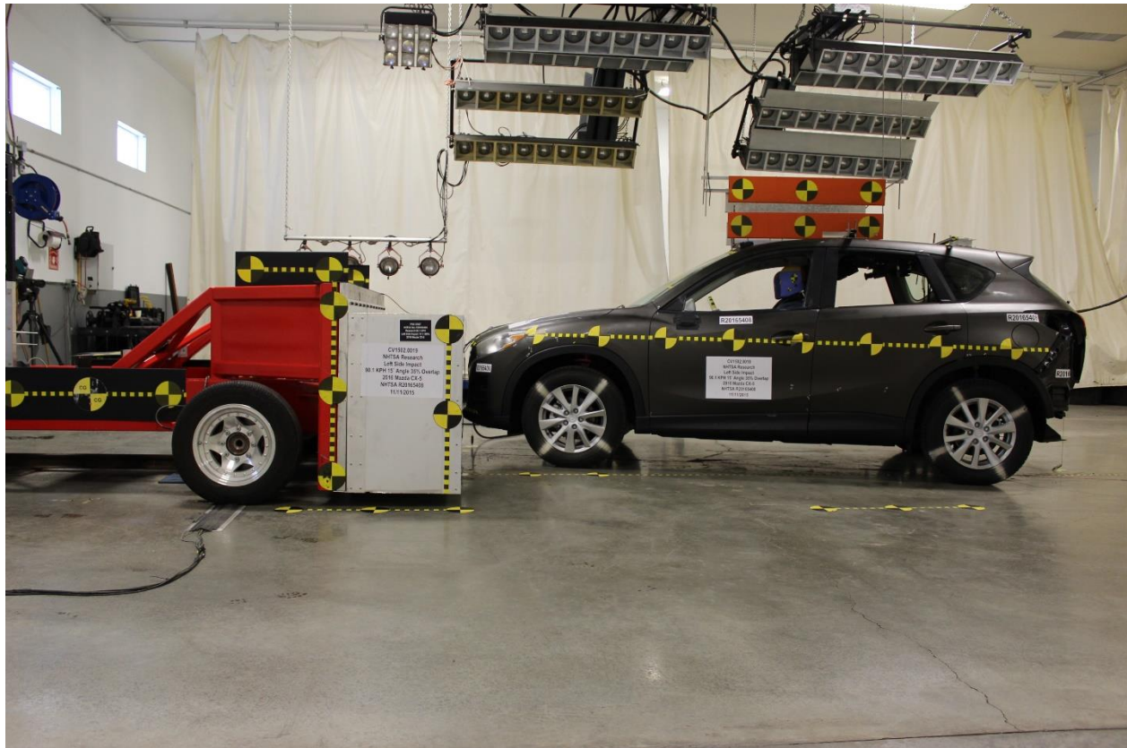
No. 183: Pre-Test OMDB & Vehicle, Right Side
