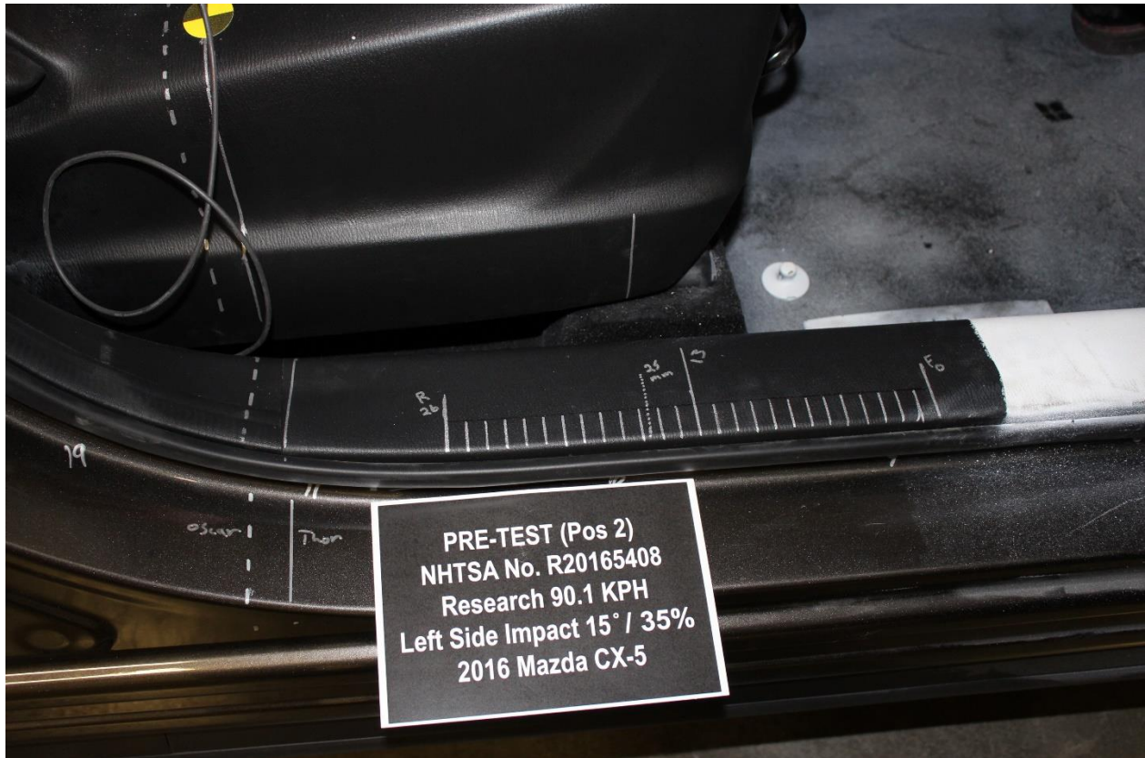
No. 104: Pre-Test Passenger Seat Fore-Aft Markings
