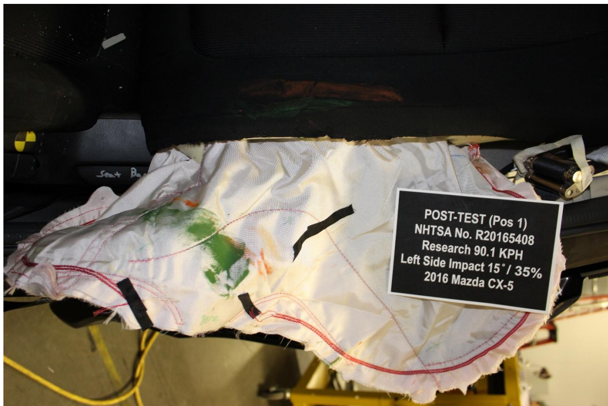
No. 081: Post-Test View of Driver Body Contact with Vehicle Interior - C
