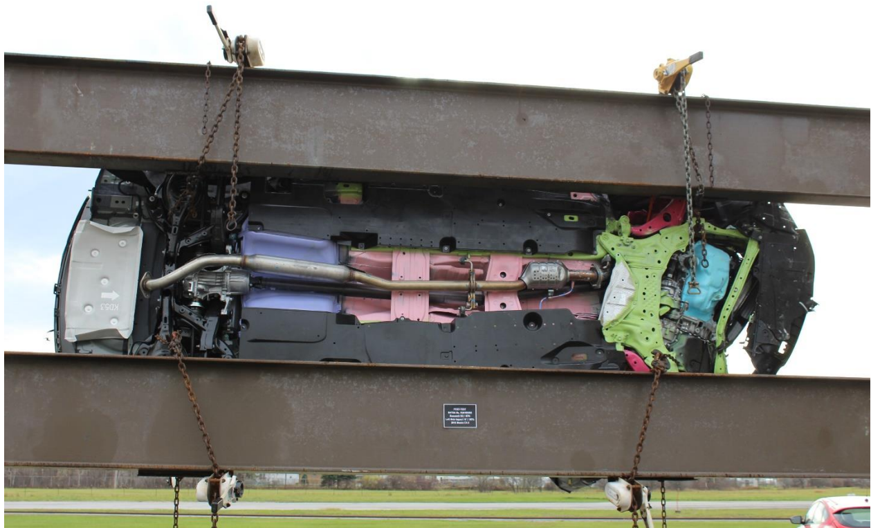
No. 195: Vehicle at 90 Degrees on Static Rollover Device
