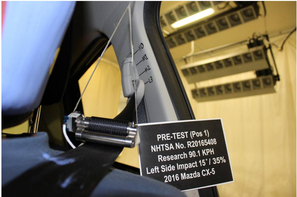
No. 065 Pre-Test Driver Adjustable D-Ring
