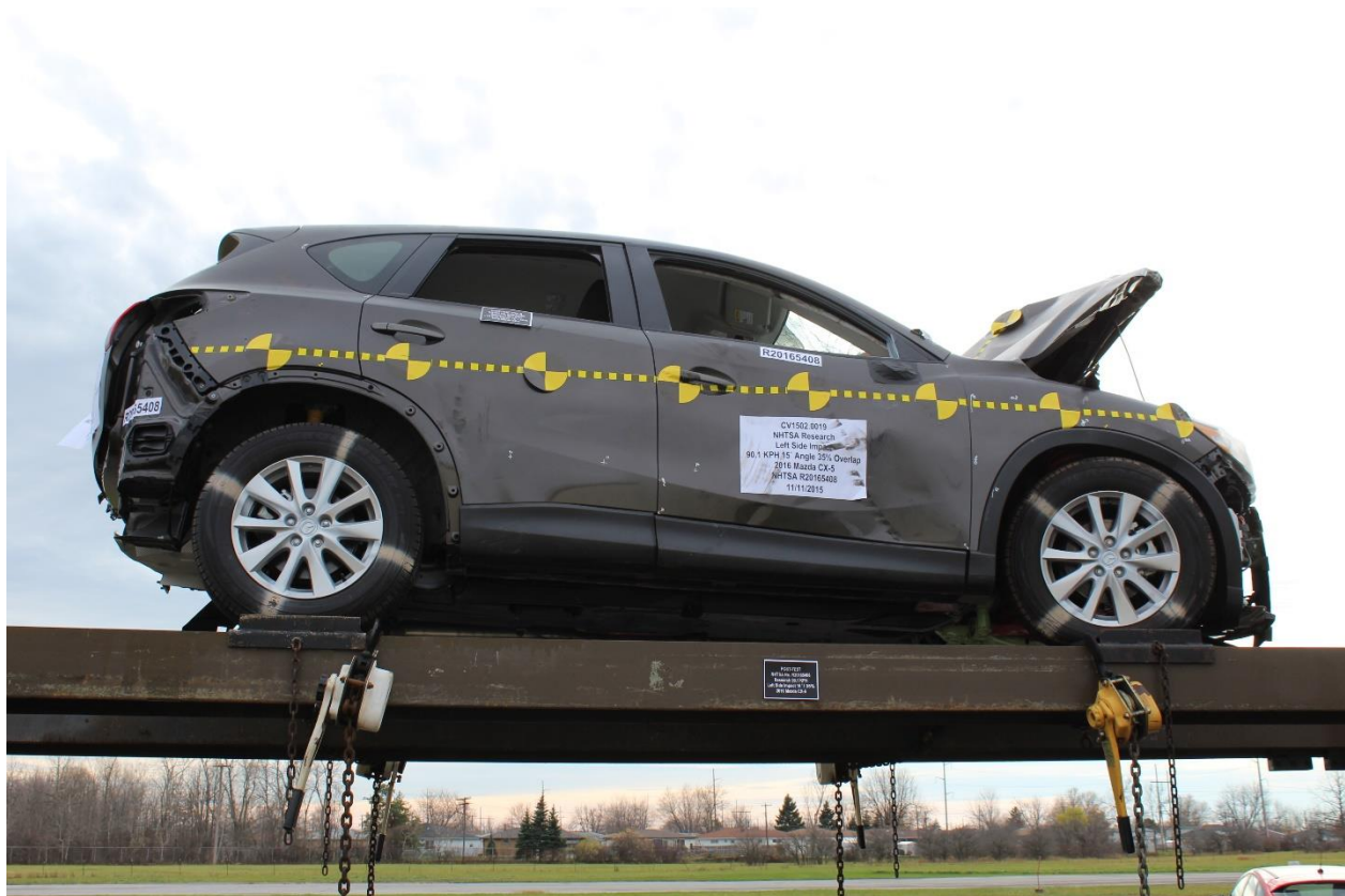
No. 194: Vehicle at 0 Degrees on Static Rollover Device
