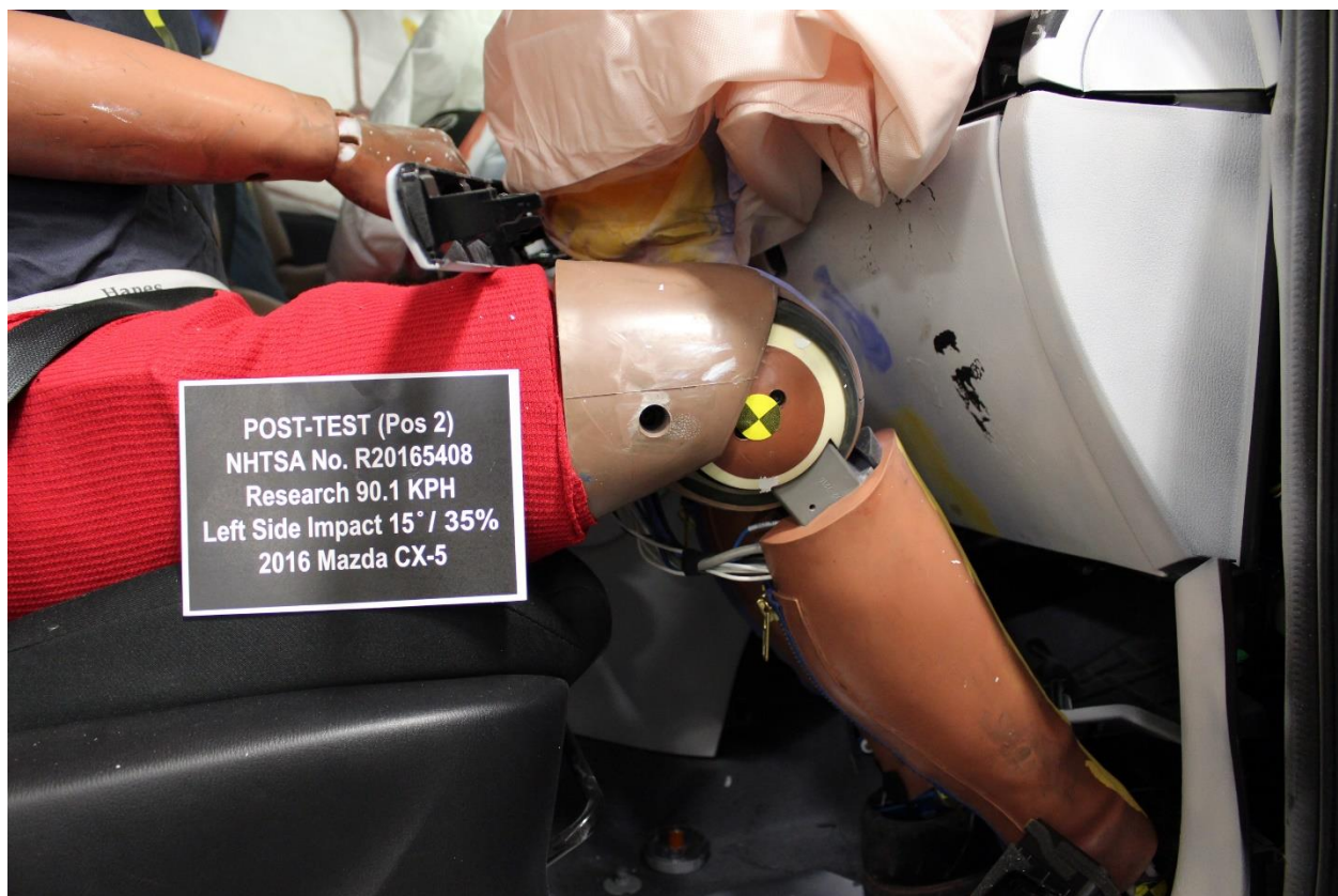
No. 113: Post-Test View of Passenger Right Knee and Bolster
