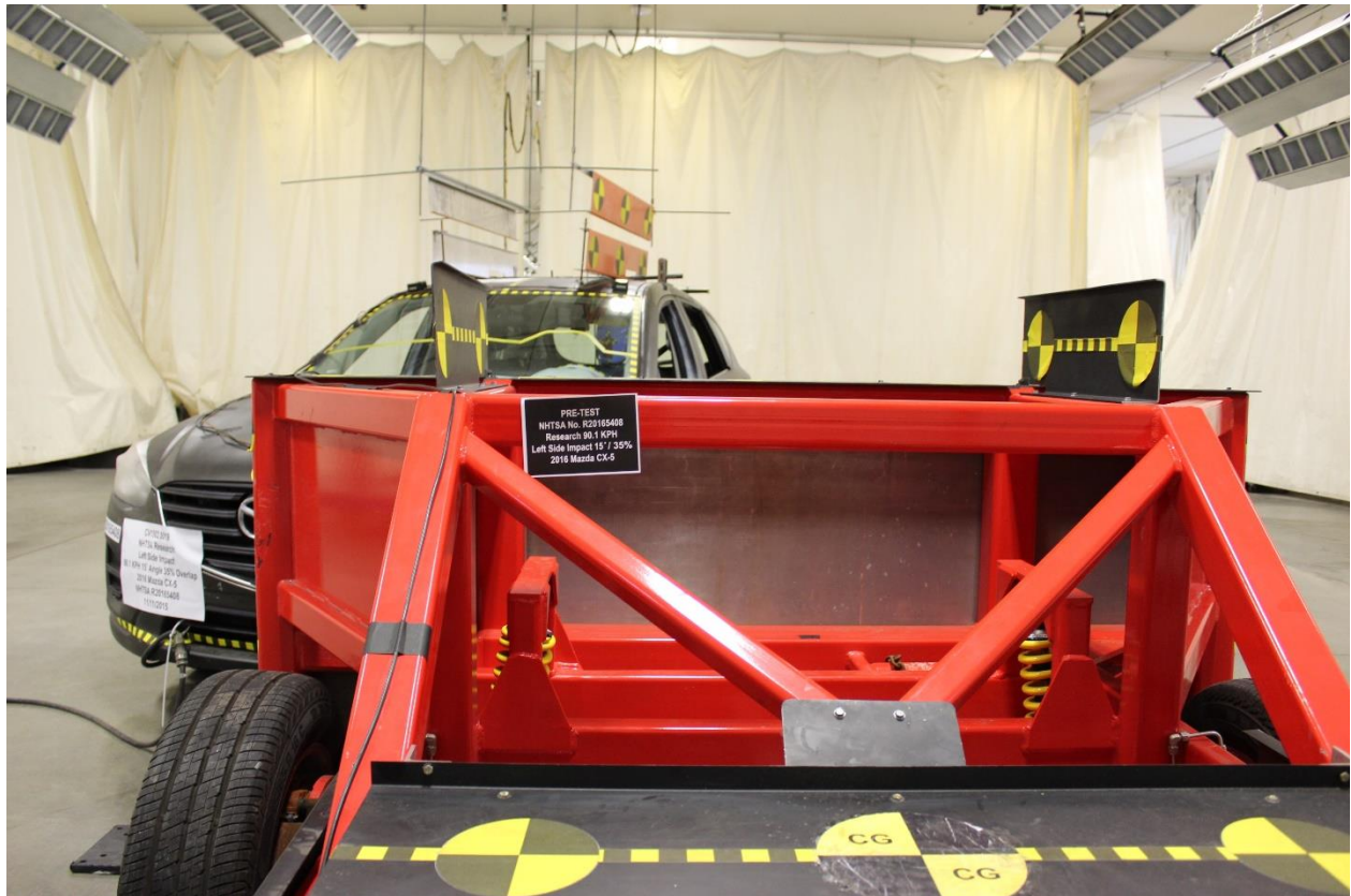
No. 189: Pre-Test OMDB & Vehicle, Rear View
