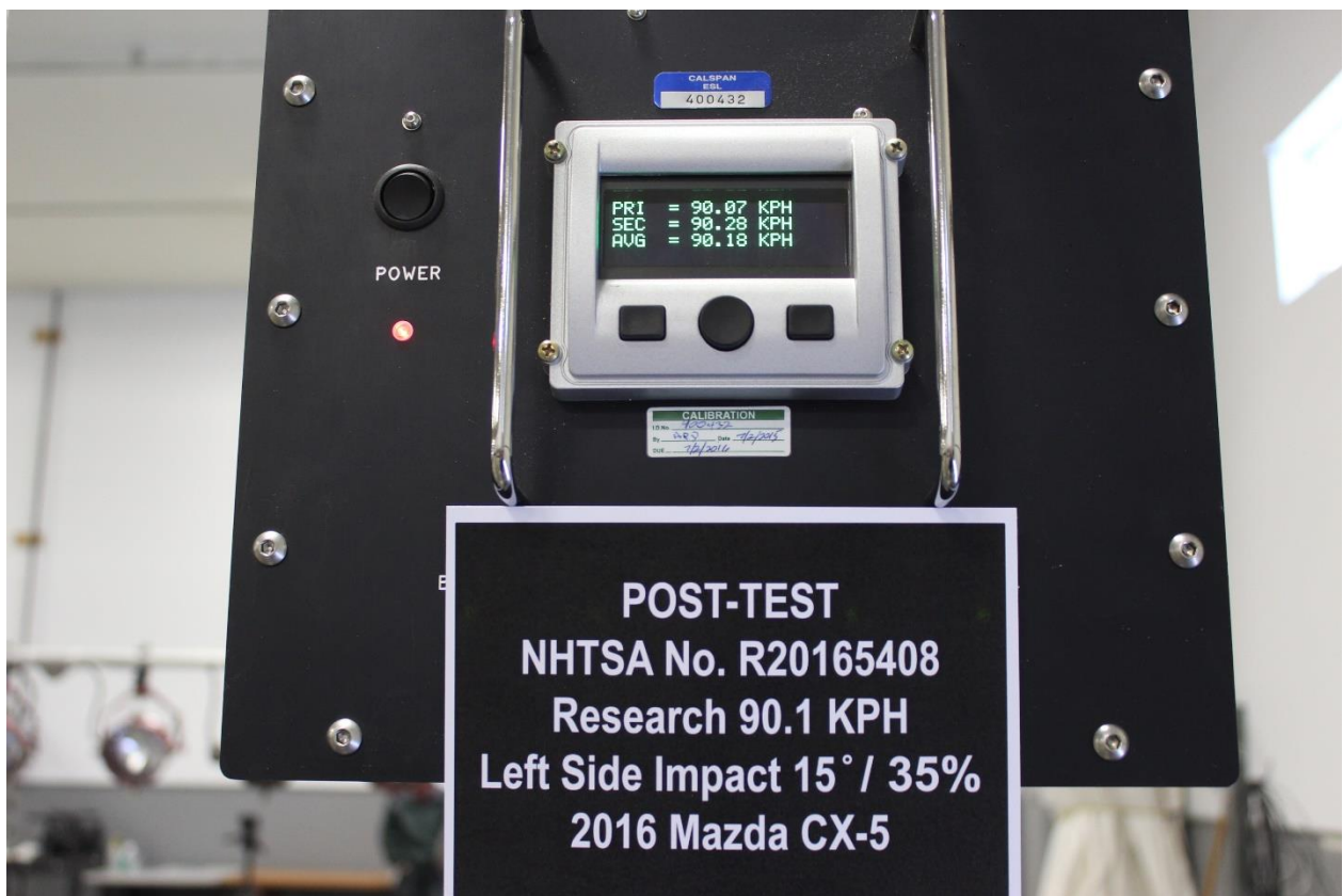
No. 125: Post-Test Speed Trap Readout
