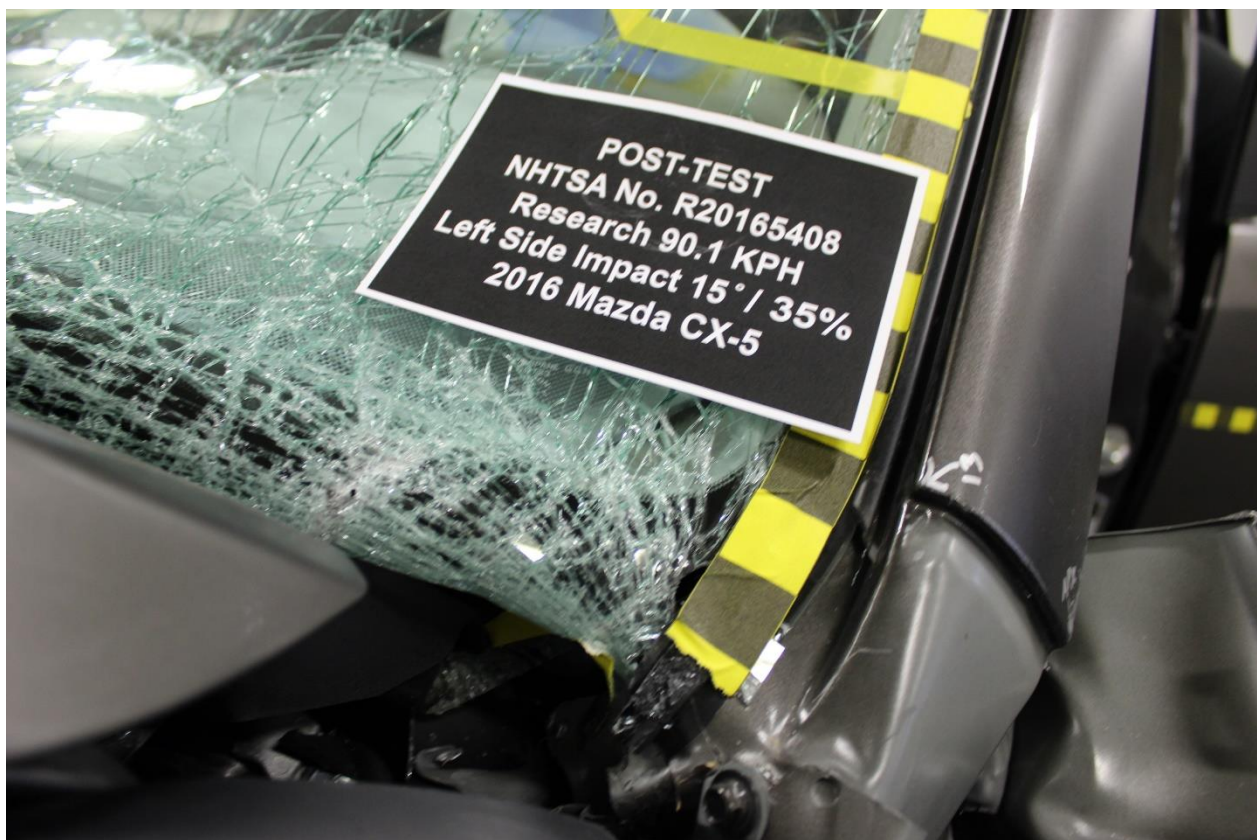
No. 166: Post-Test View of Windshield Separation
