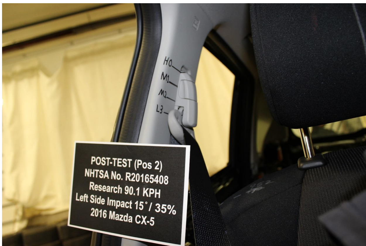
No. 109: Post-Test Passenger Adjustable D-ring
