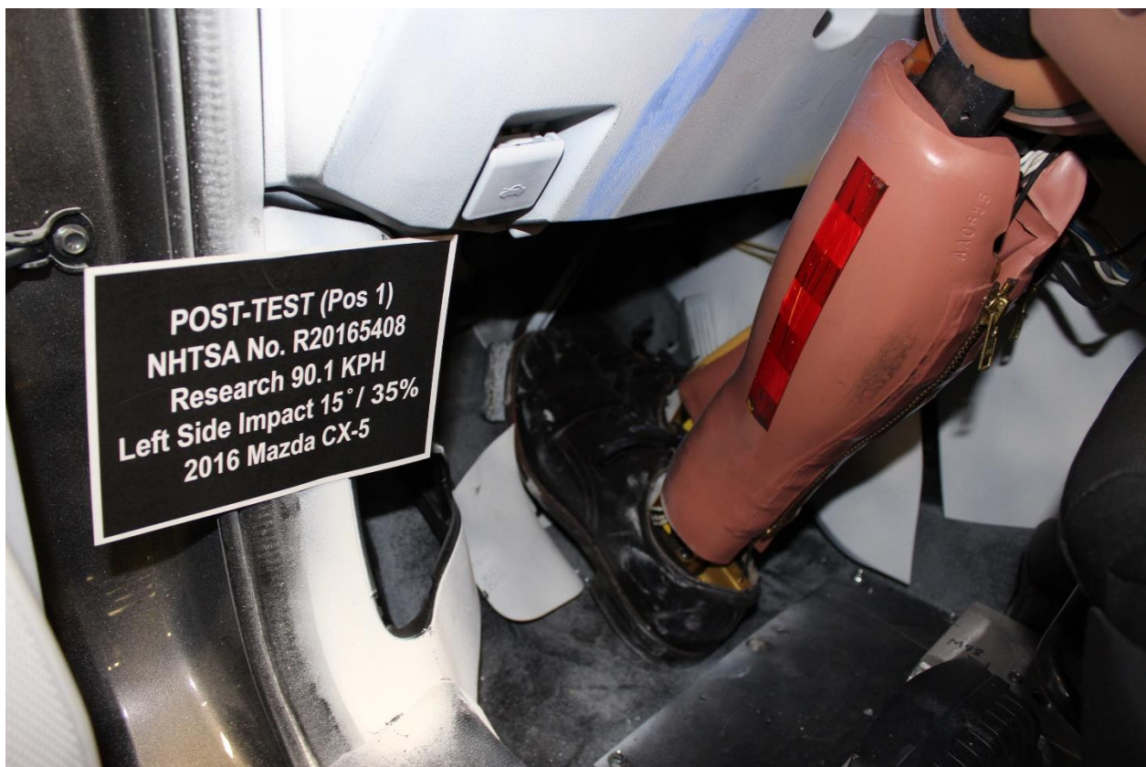
No. 068 Post-Test Driver Feet
