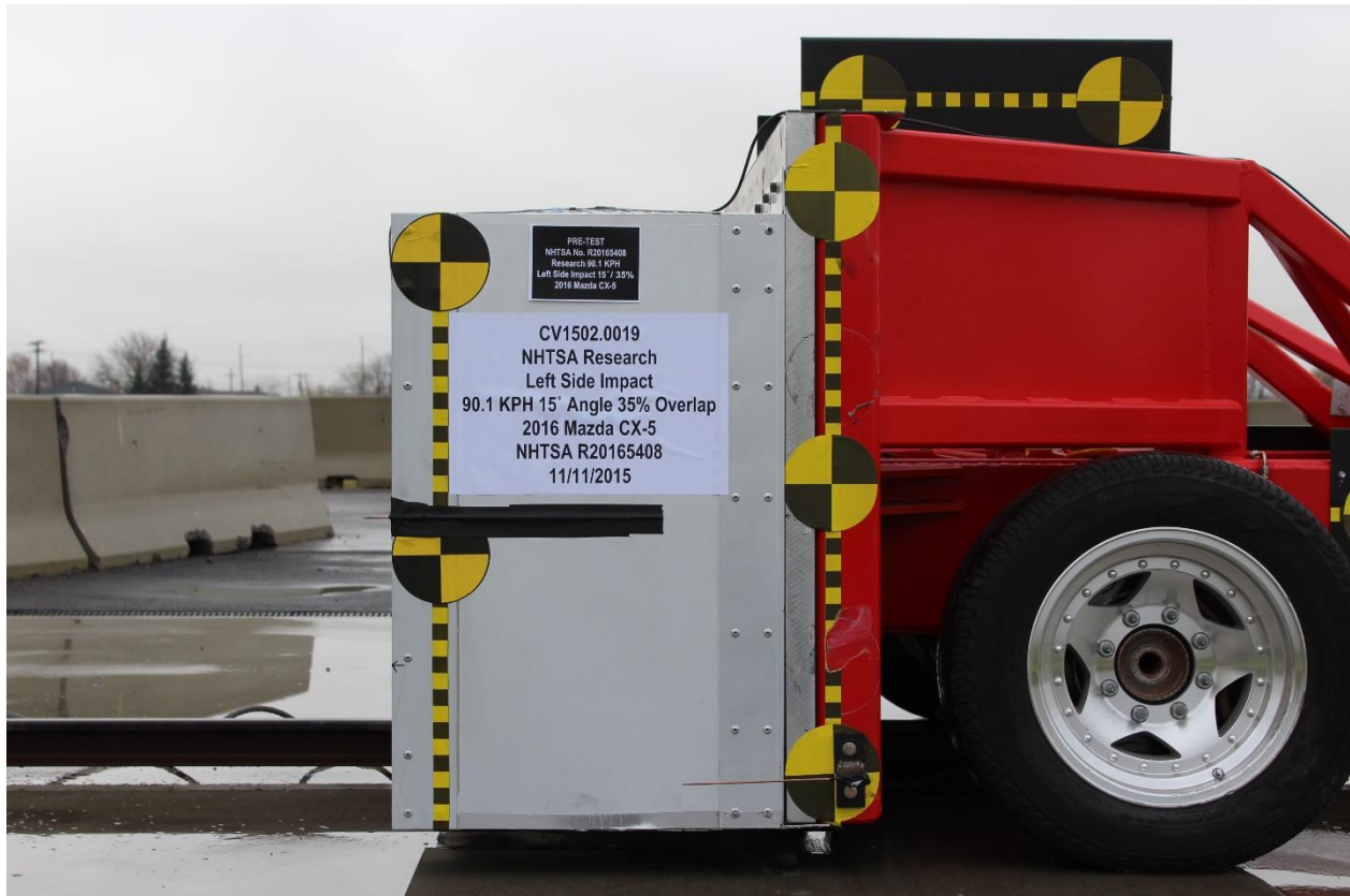
No. 167: Pre-Test Left Side View of OMDB
