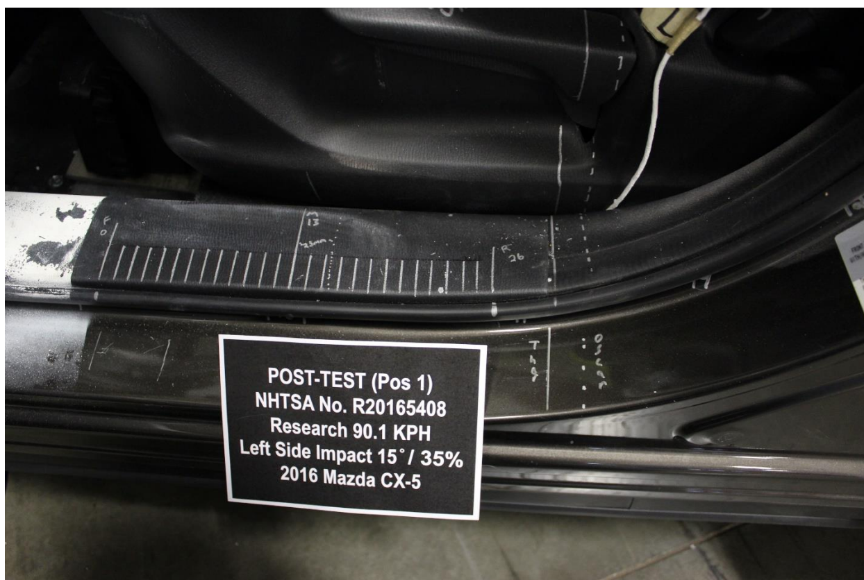
No. 062 Post-Test Driver Seat Fore Aft Markings
