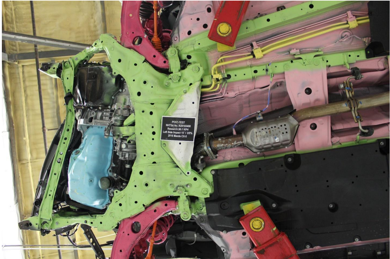
No. 144: Post-Test View of Front Sub-Frame Deformation
