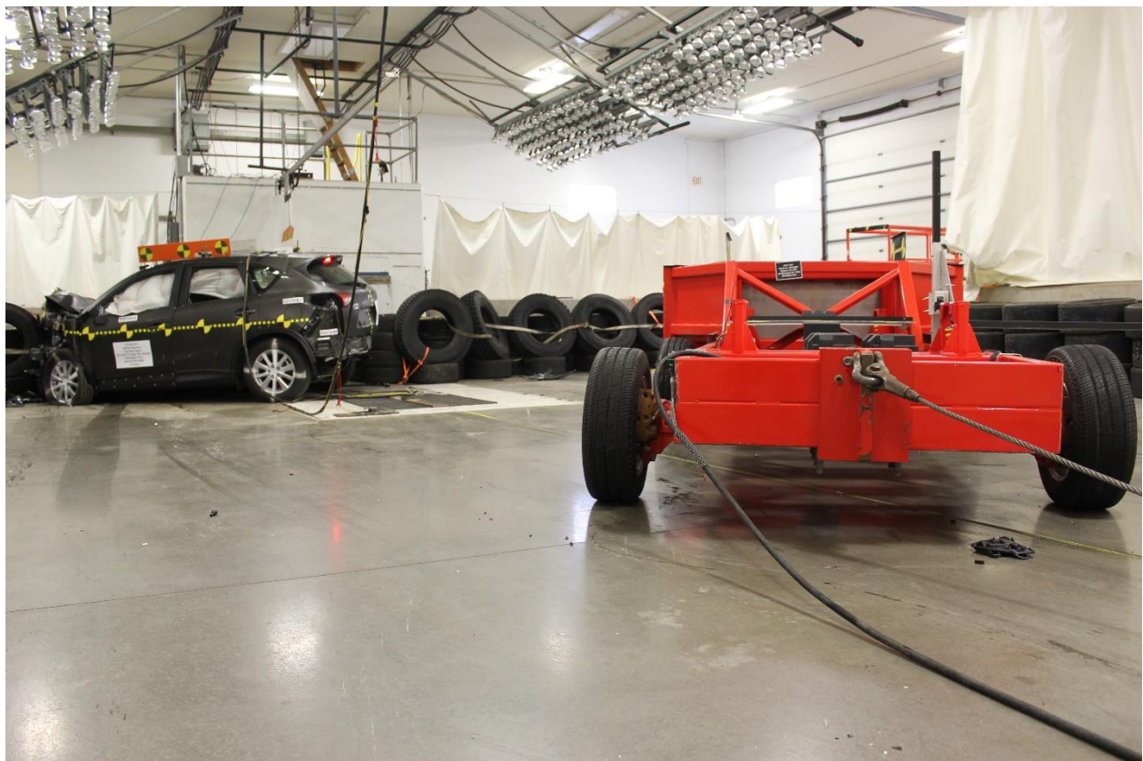
No. 190: Post-Test OMDB & Vehicle, Rear View
