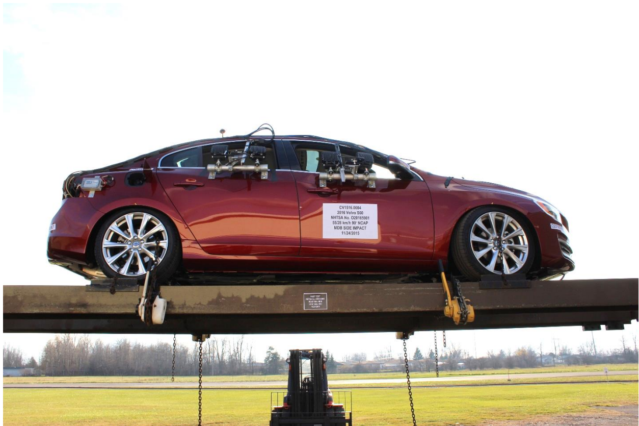
Figure A-100: FMVSS No. 301 Static Rollover 360 Degrees
