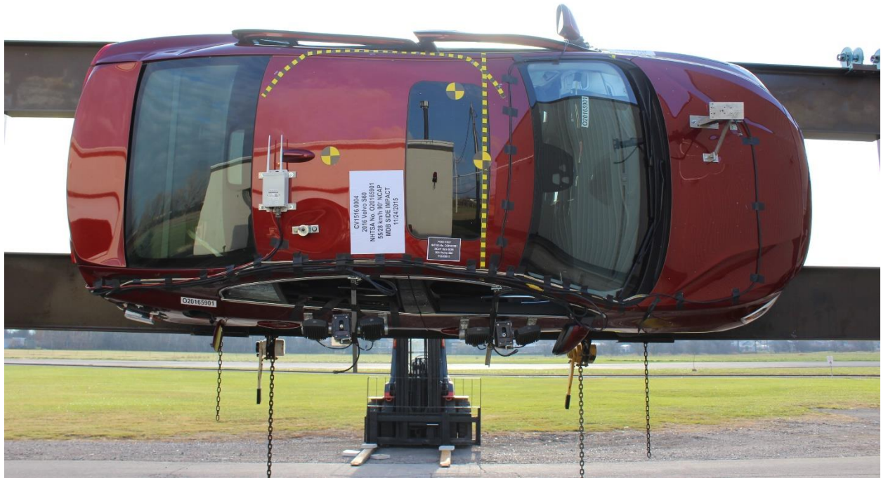
Figure A-97: FMVSS No. 301 Static Rollover 90 Degrees
