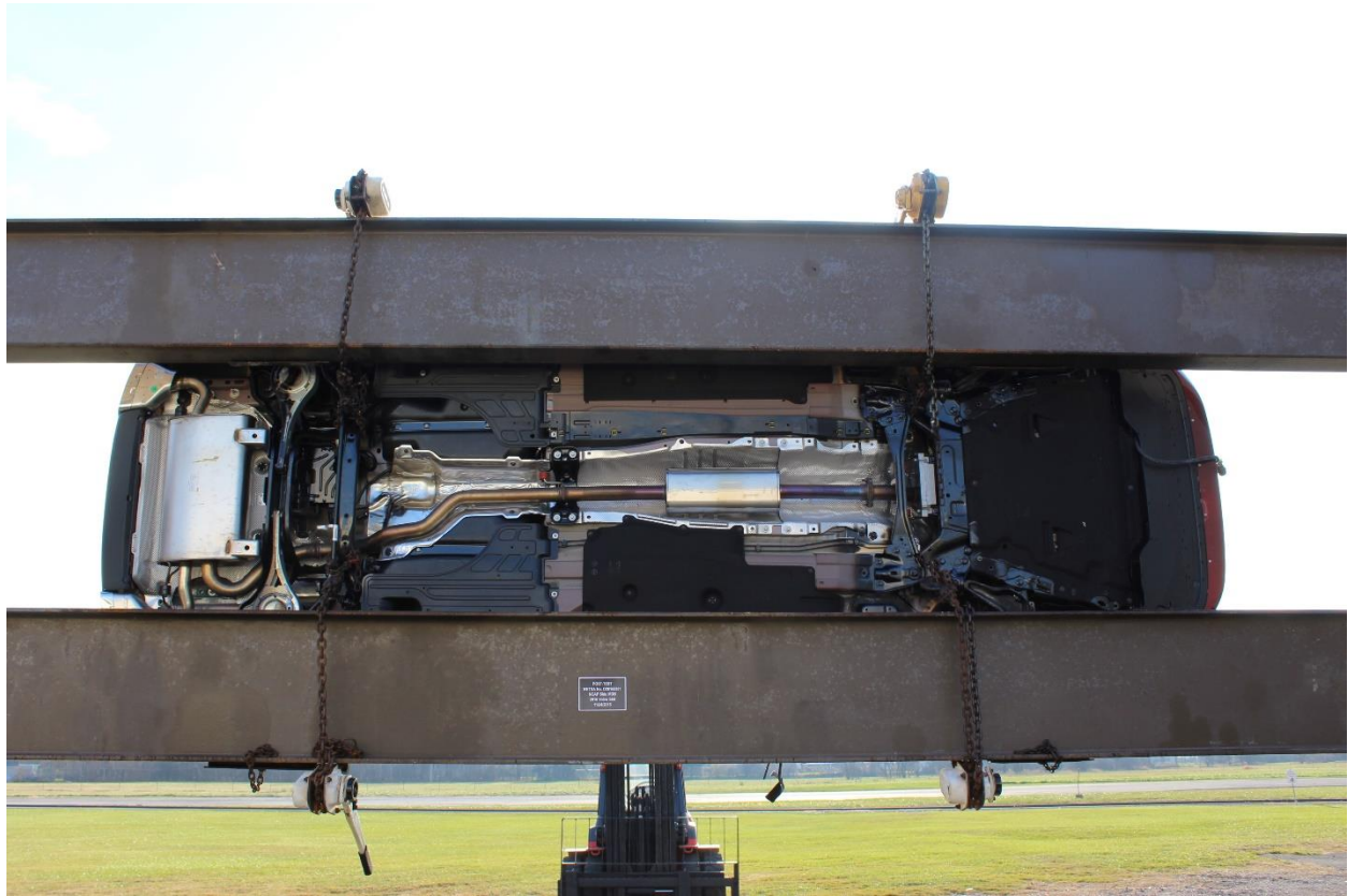
Figure A-99: FMVSS No. 301 Static Rollover 270 Degrees
