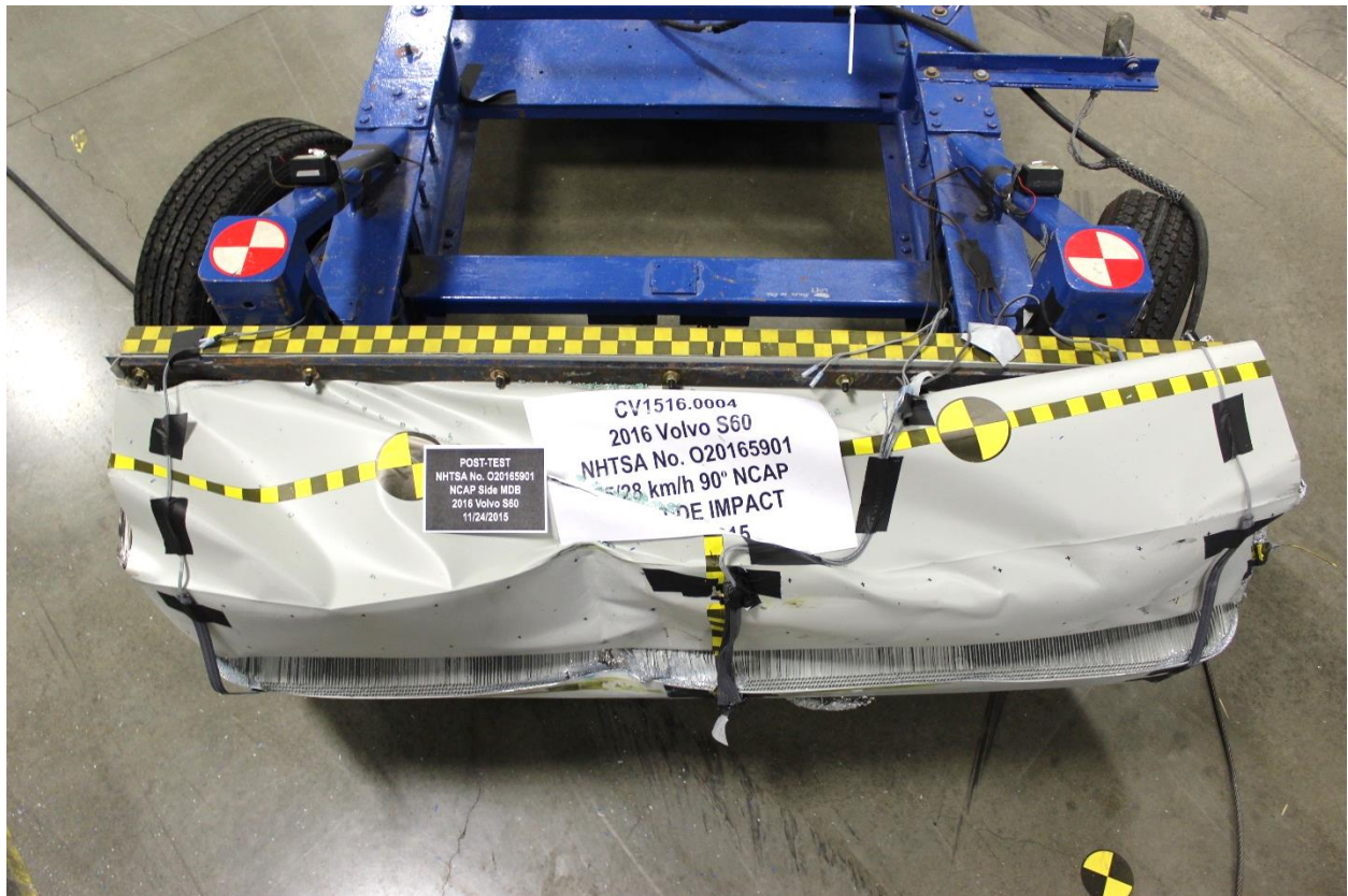
Figure A-87: Post-Test Top View of MDB Impactor Face
