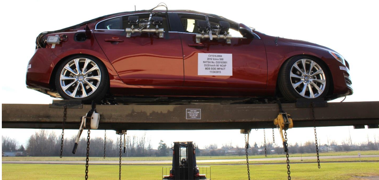
Figure A-96: FMVSS No. 301 Static Rollover 0 Degrees
