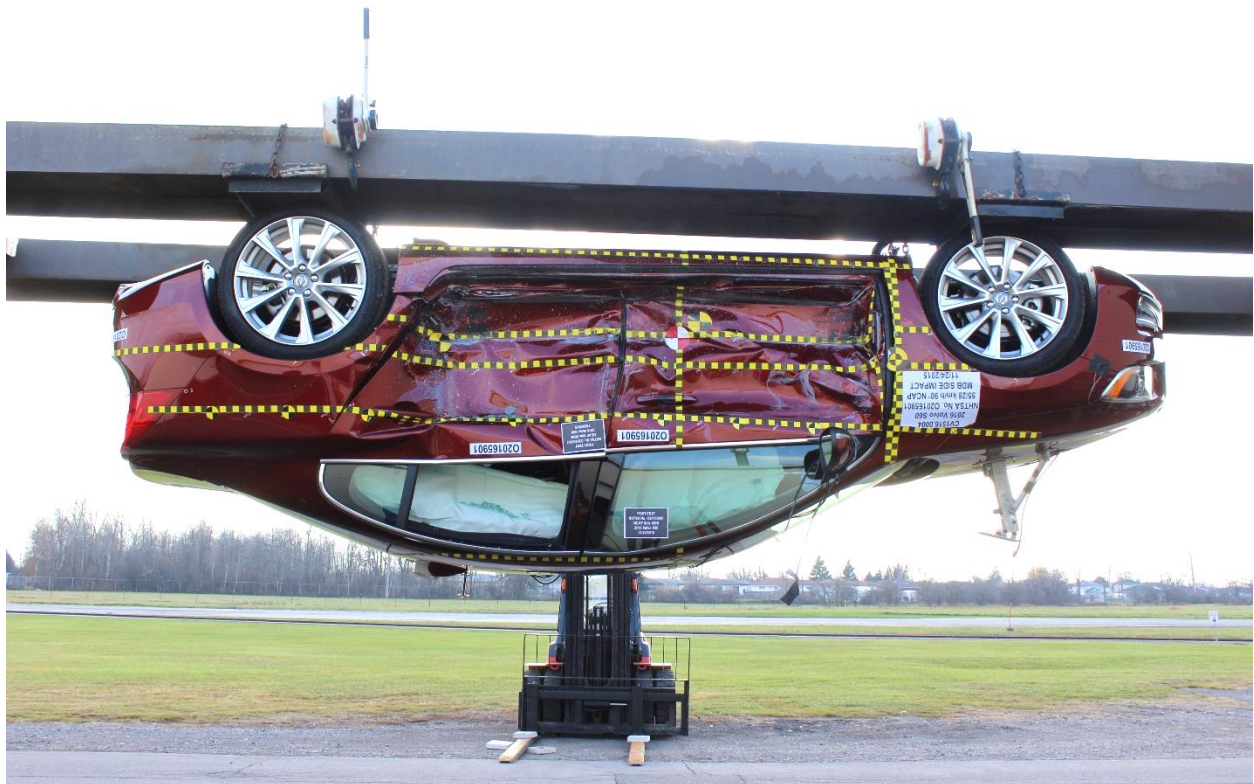
Figure A-98: FMVSS No. 301 Static Rollover 180 Degrees
