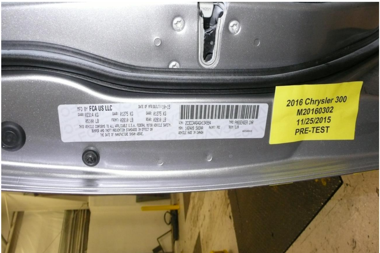
092 Close-Up View of Vehicle Certification Label
