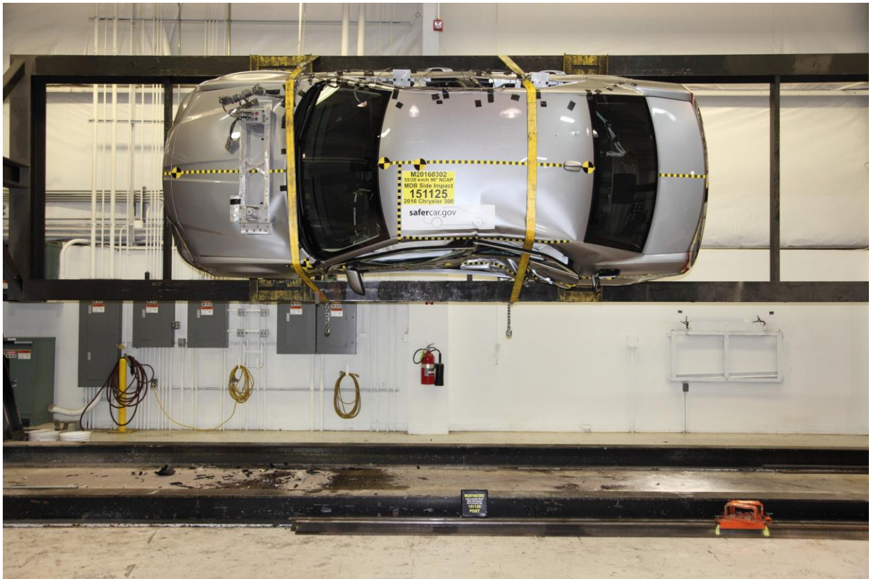
097 FMVSS No. 301 Static Rollover 90 Degrees
