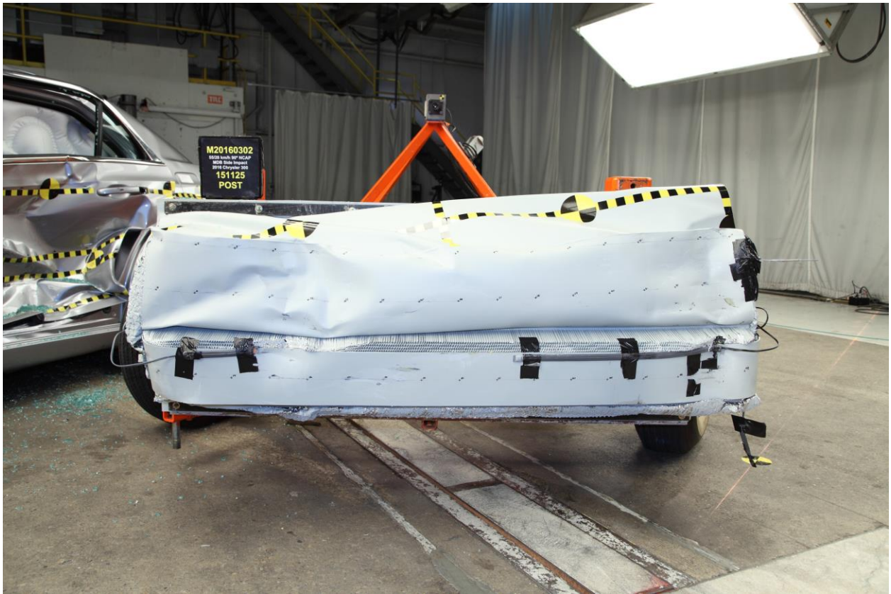
085 Post-Test Front View of MDB Impactor Face
