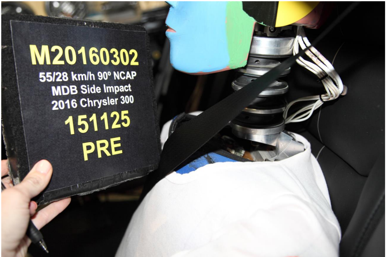
062 Pre-Test View of Rear Passenger Dummy Neck Showing Position of Adjustable Neck Bracket
