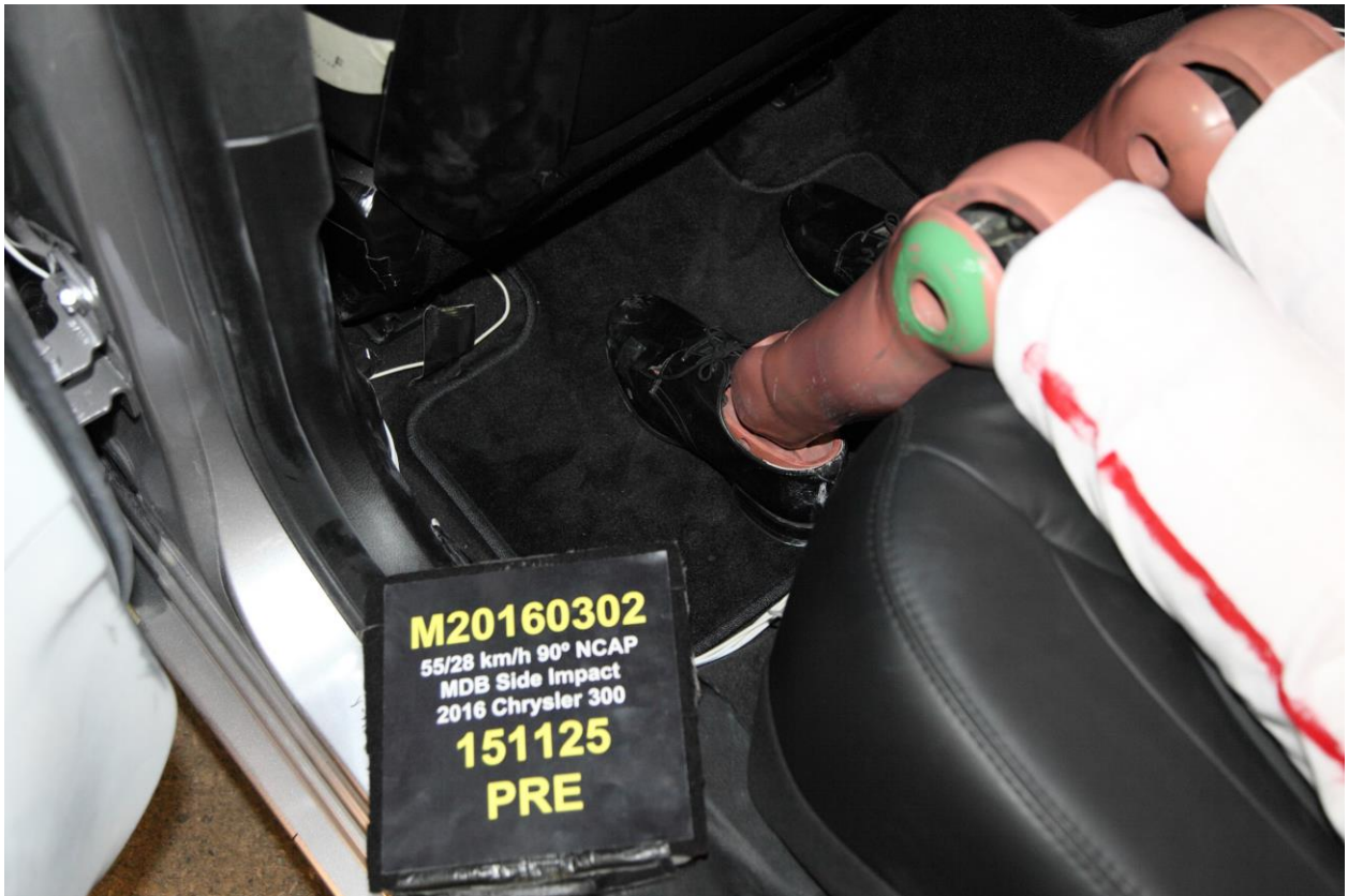
064 Pre-Test Placement of Rear Passenger Dummy Feet
