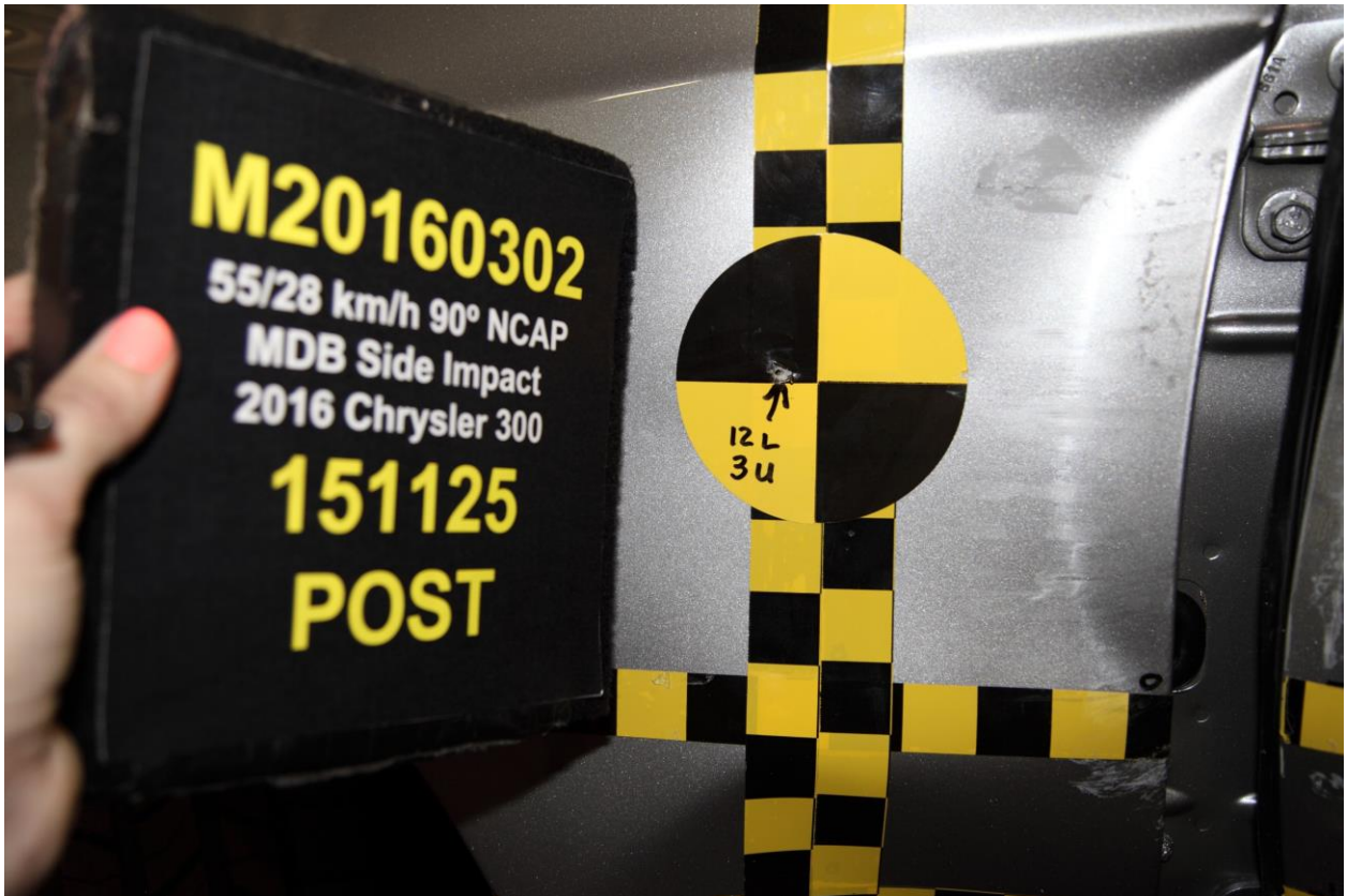
020 Post-Test Close-up View of Impact Point Target
