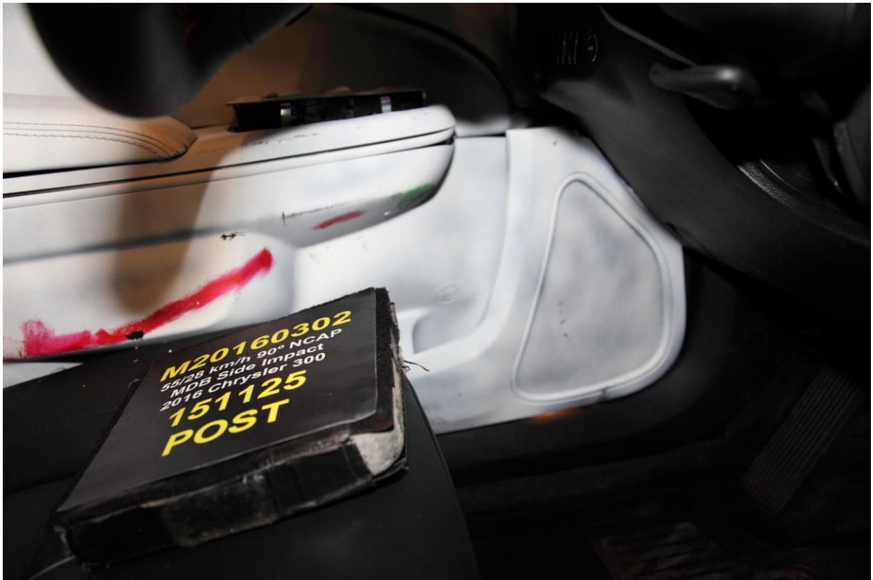
054 Post-Test Driver Dummy Close-Up Knee Contact View
