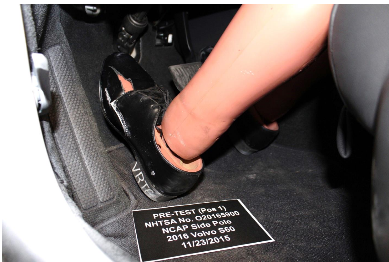
Figure A-32: Pre-Test Placement of Dummy's Feet
