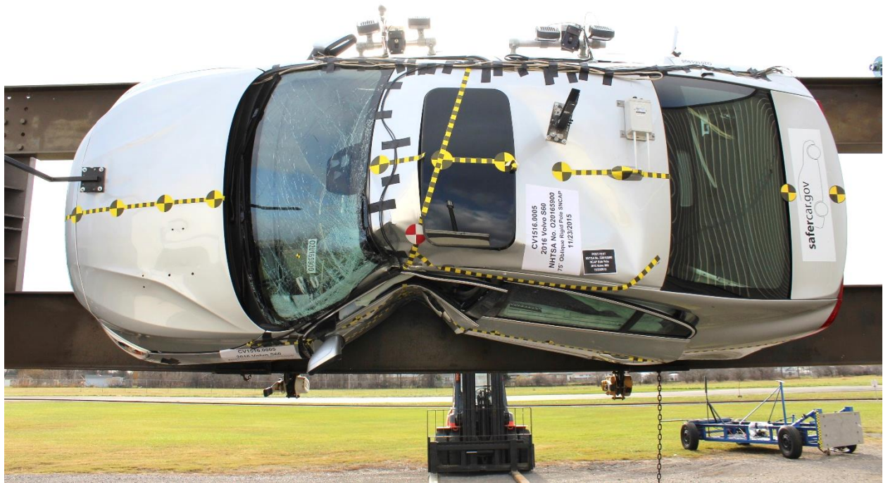
Figure A-66: FMVSS No. 301 Static Rollover 270 Degrees
