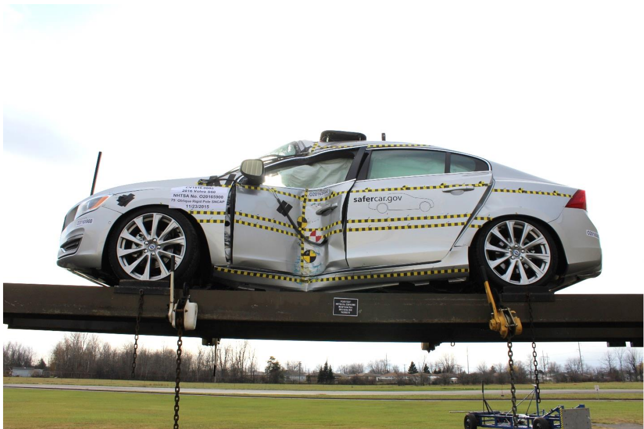
Figure A-67: FMVSS No. 301 Static Rollover 360 Degrees
