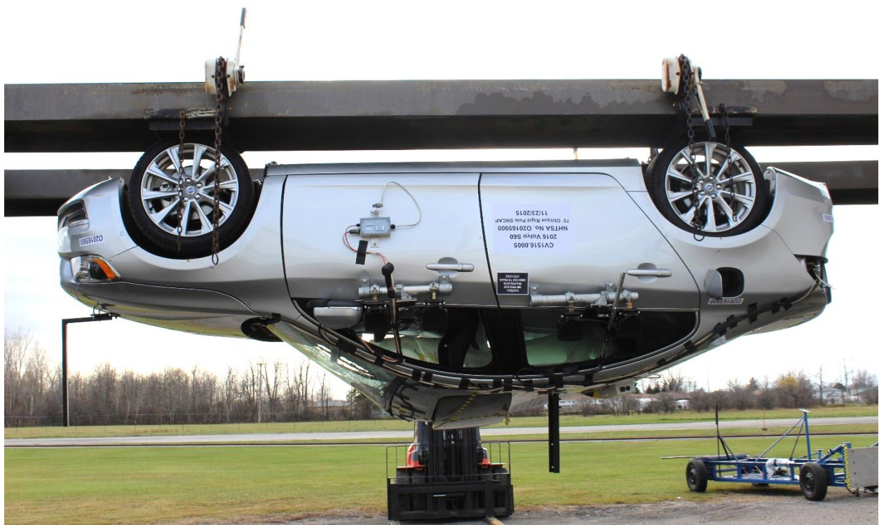
Figure A-65: FMVSS No. 301 Static Rollover 180 Degrees
