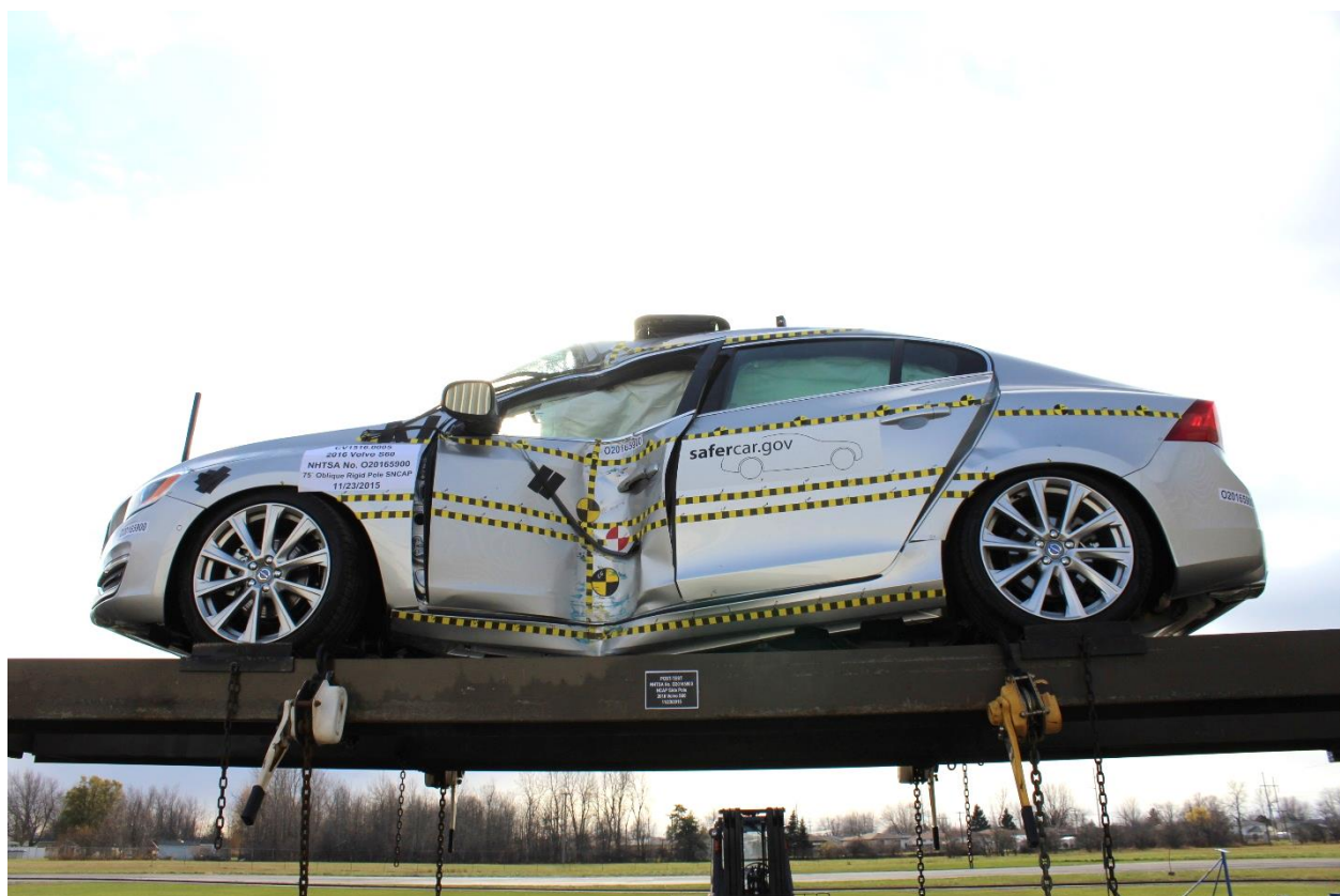
Figure A-63: FMVSS No. 301 Static Rollover 0 Degrees
