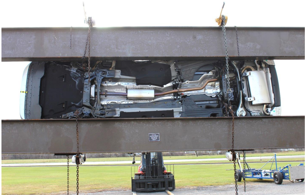
Figure A-64: FMVSS No. 301 Static Rollover 90 Degrees
