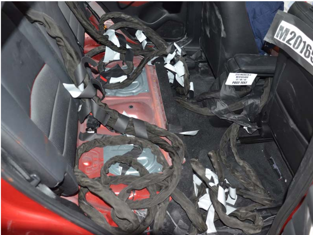
FIGURE 28. Post-Test Dummy Cable Routing
