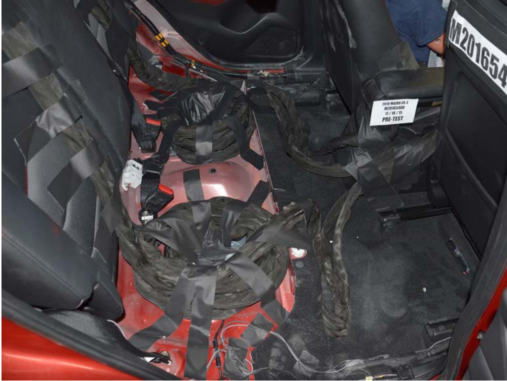
FIGURE 27. Pre-Test Dummy Cable Routing
