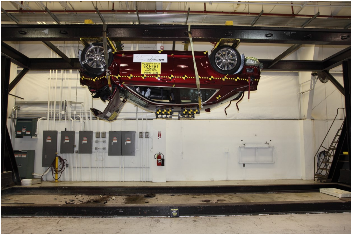
075 Vehicle at 180° on Static Rollover Device
