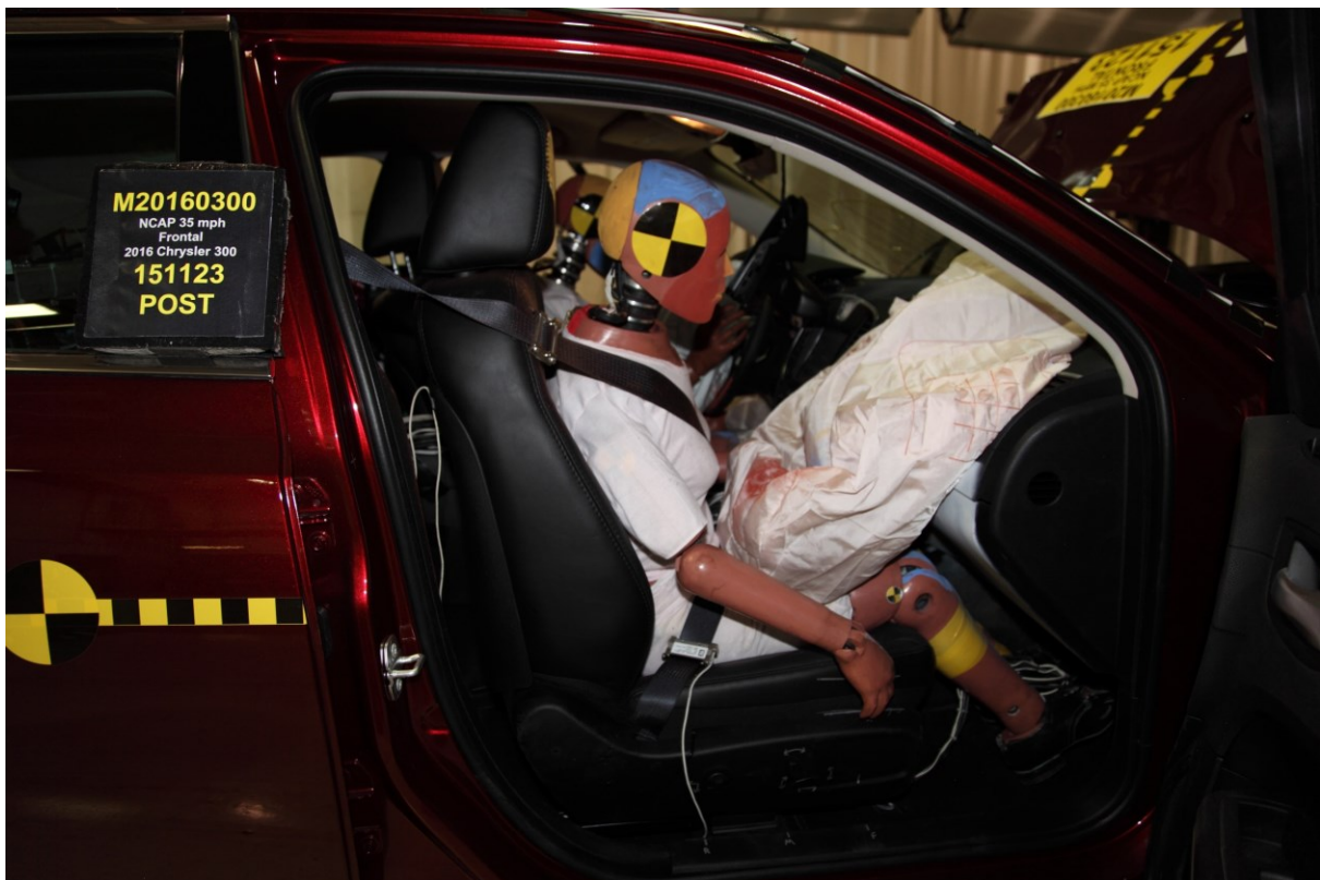
056 Post-Test Passenger Dummy and Vehicle Interior View
