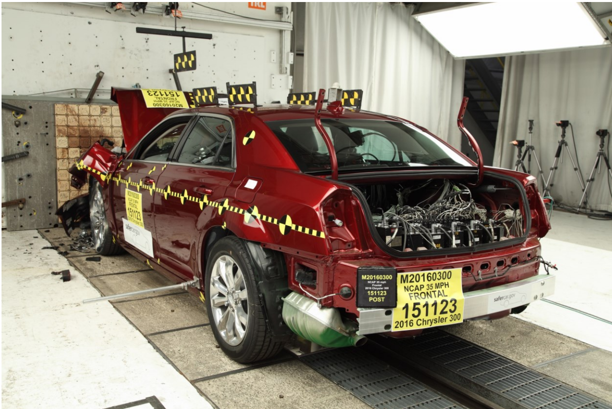
017 Post-Test Left Rear 3-4 View
