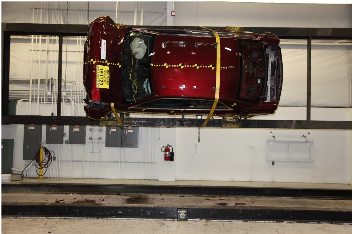
074 Vehicle at 90° on Static Rollover Device
