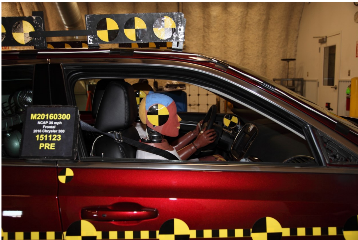
053 Pre-Test Passenger Dummy Window View
