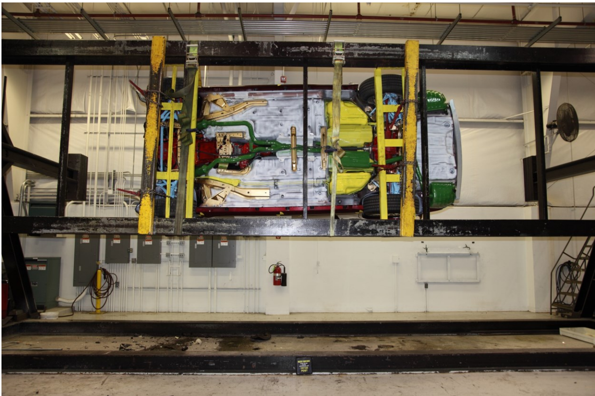
076 Vehicle at 270° on Static Rollover Device
