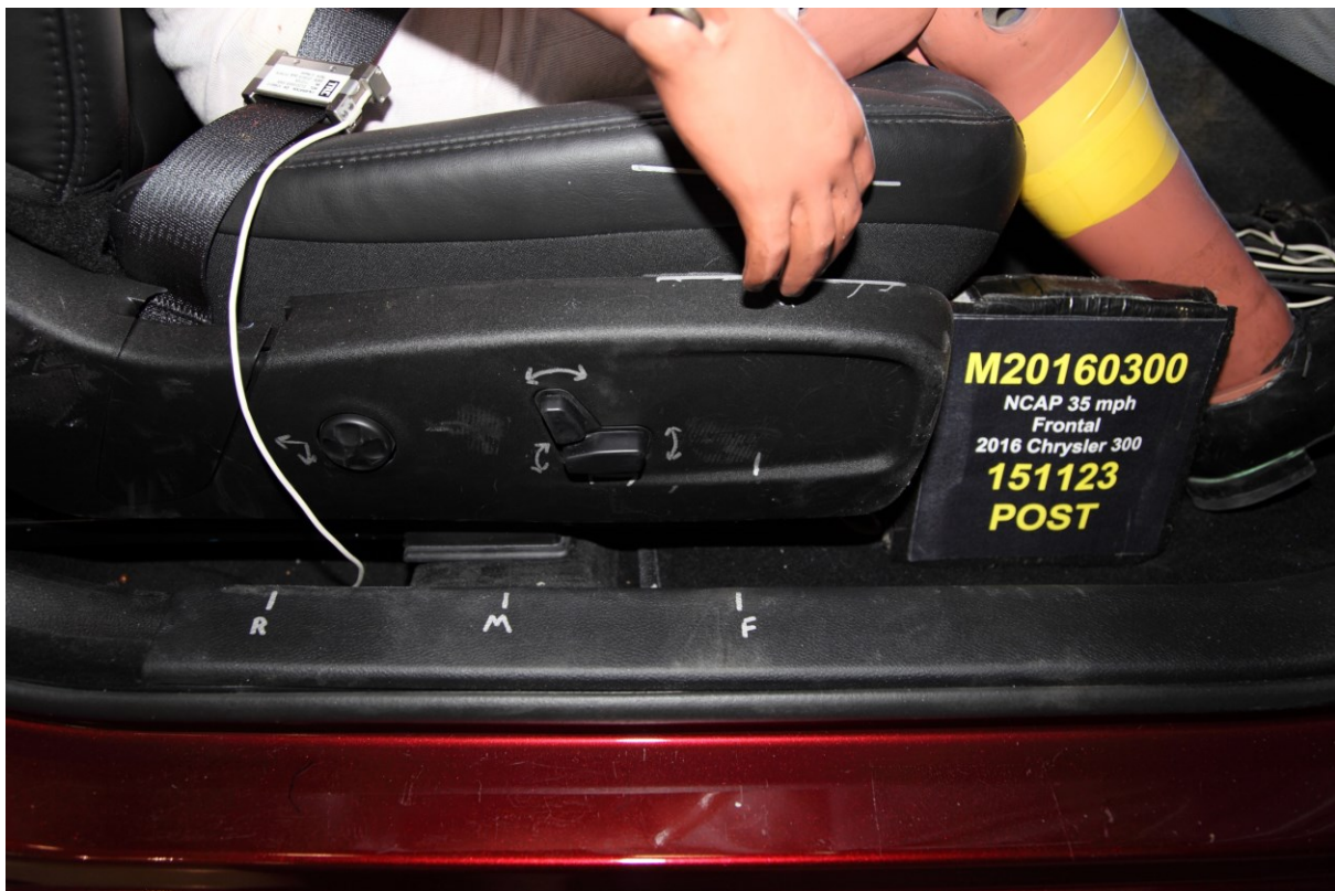
058 Post-Test Passenger's Seat Fore-Aft Markings
