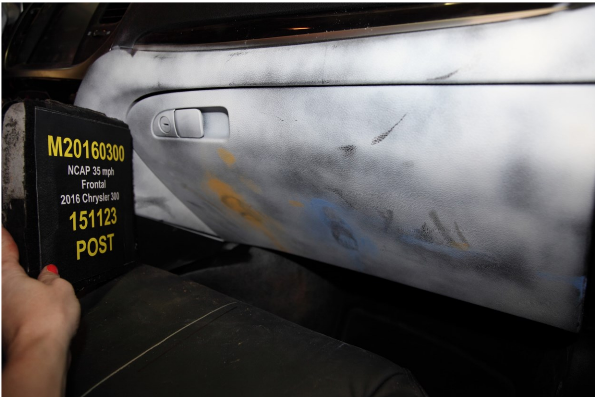
064 Post-Test Passenger's Side Knee Bolster
