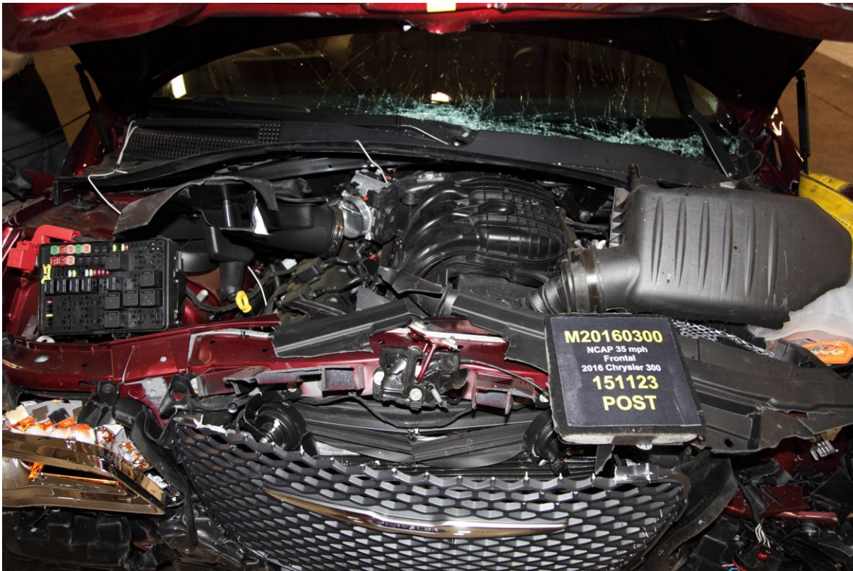
021 Post-Test Engine Compartment View
