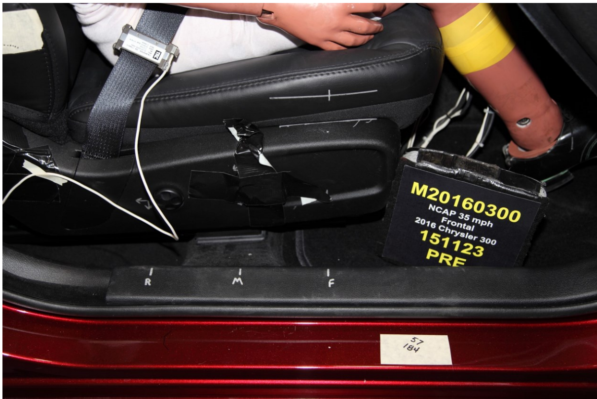
057 Pre-Test Passenger's Seat Fore-Aft Markings
