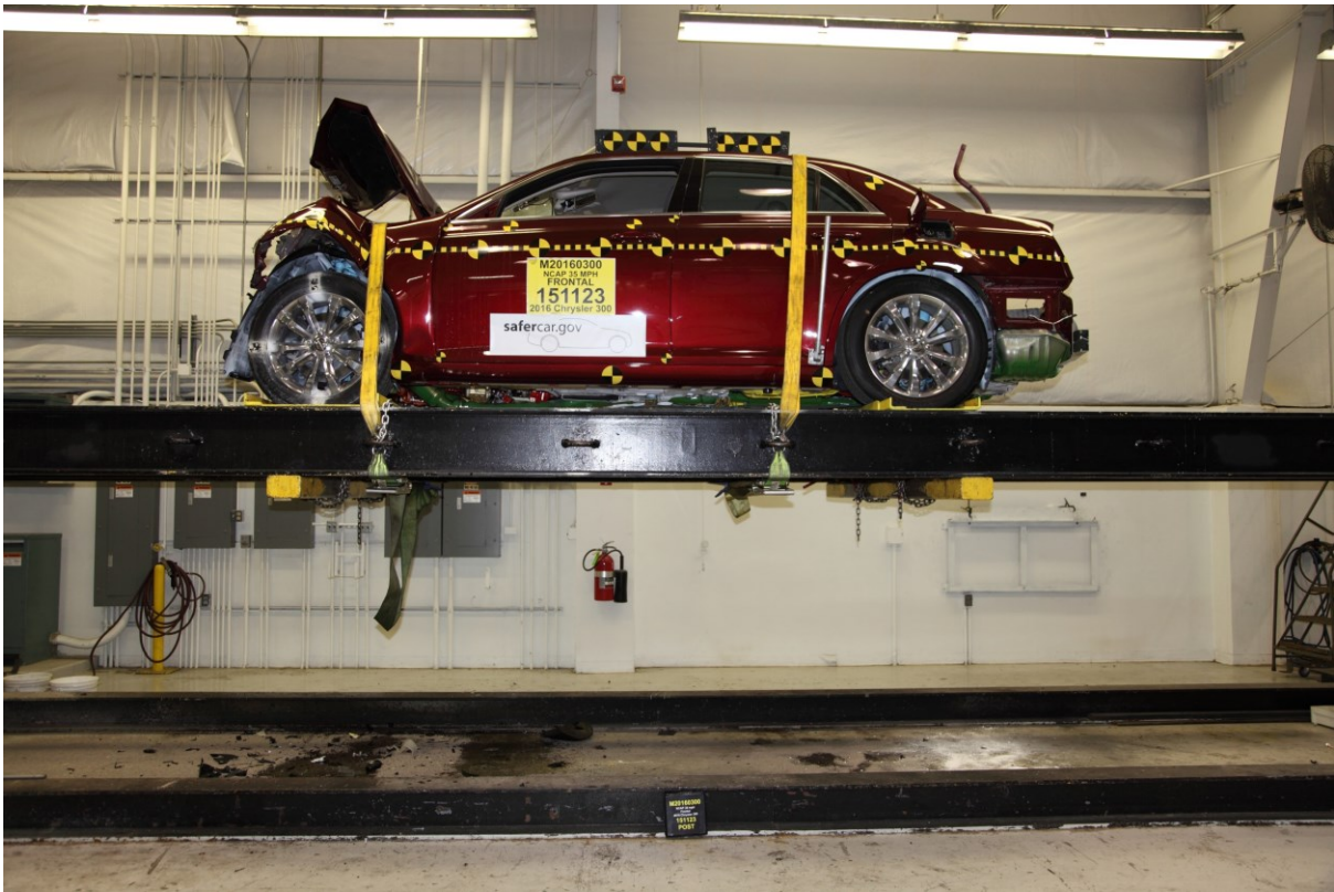
077 Vehicle at 360° on Static Rollover Device
