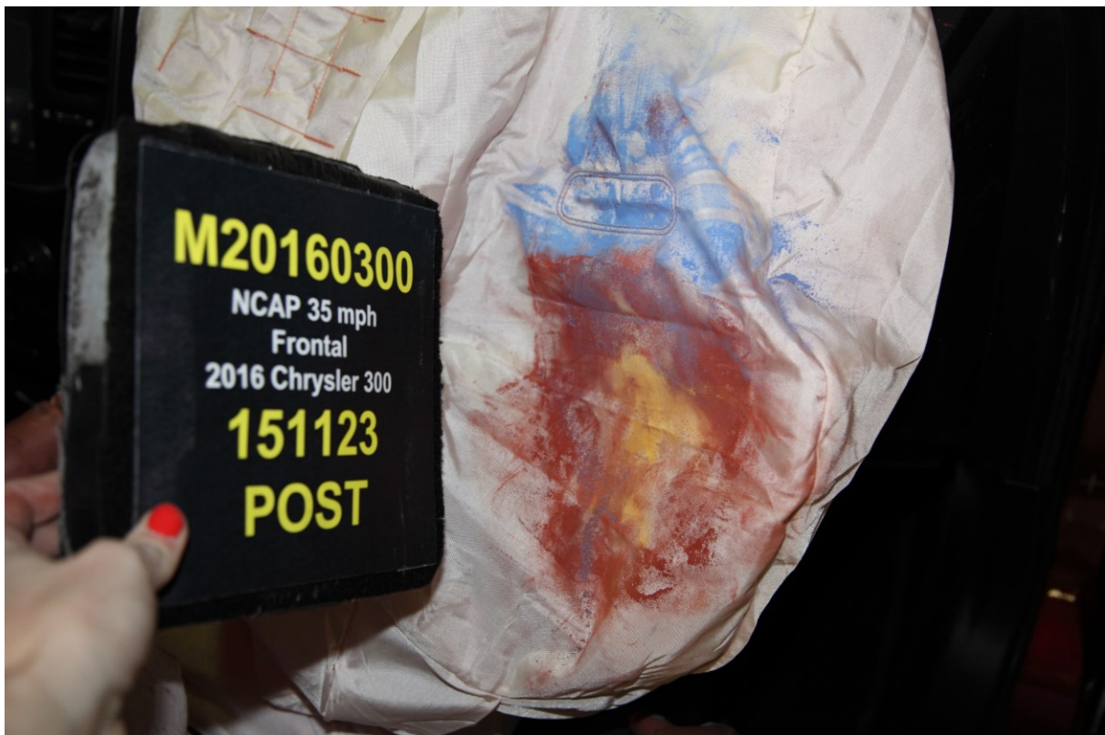
068 Post-Test Passenger Dummy Contact With Airbag
