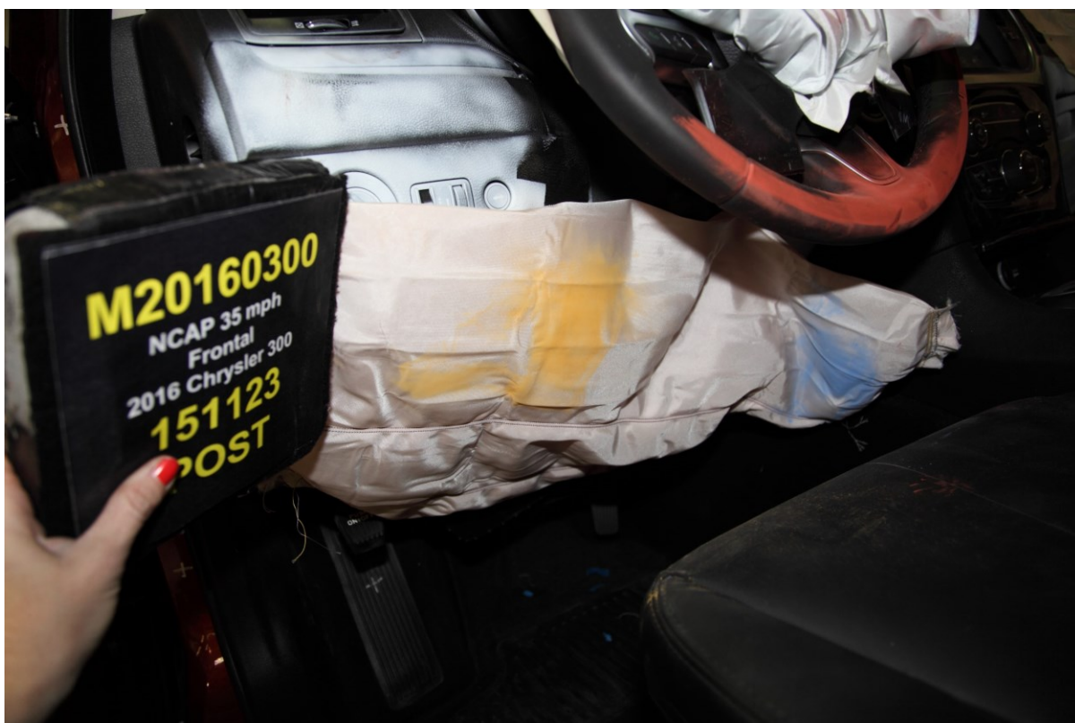
043 Post-Test Driver's Side Knee Bolster
