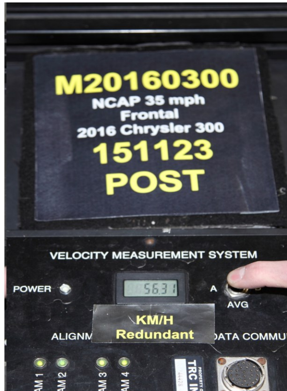
072 Post-Test Speed Trap Readout
