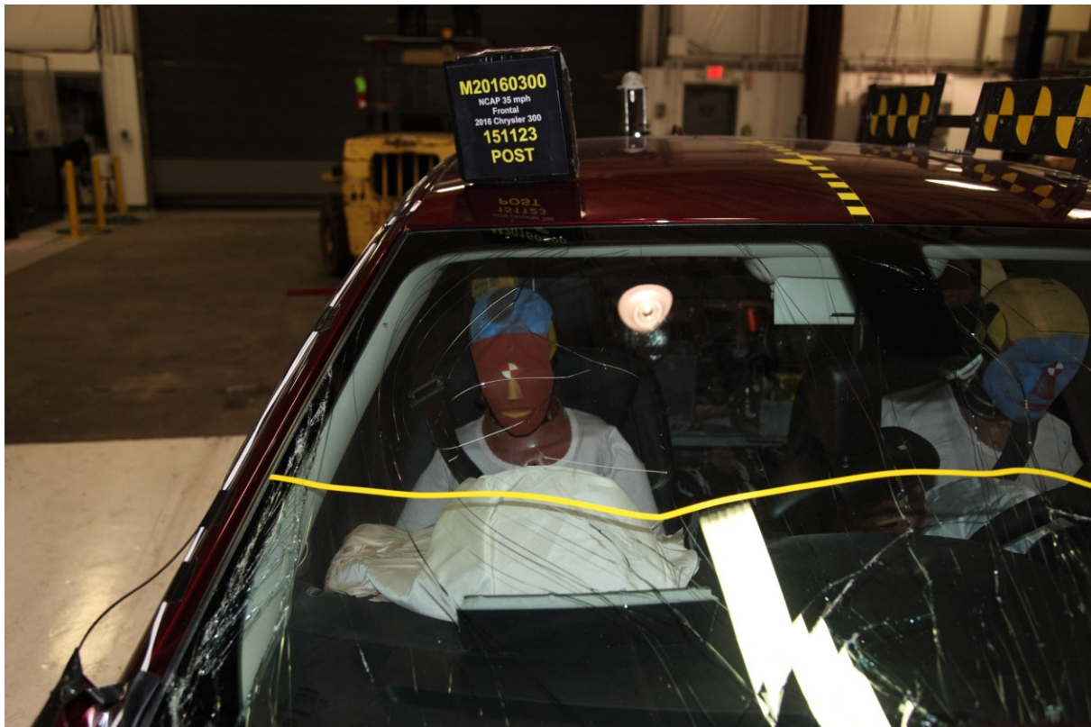
052 Post-Test Passenger Dummy Front View
