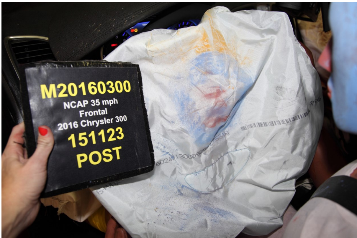
047 Post-Test Driver Dummy Contact With Airbag
