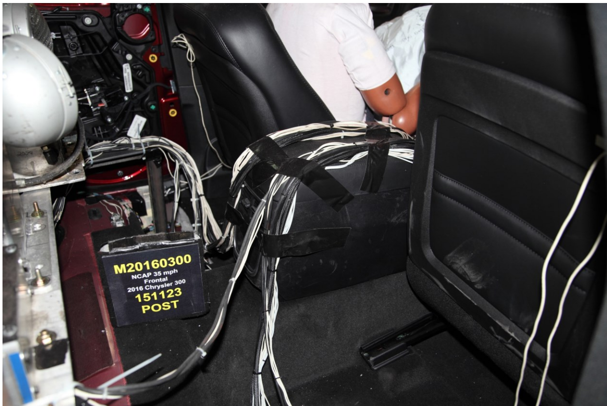
029 Post-Test Dummy Cable Routing
