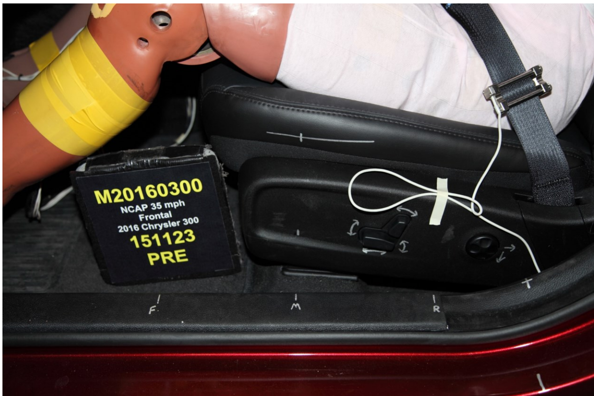
036 Pre-Test Driver's Seat Fore-Aft Markings
