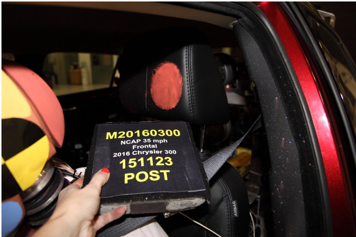
048 Post-Test Driver Dummy Contact With Headrest
