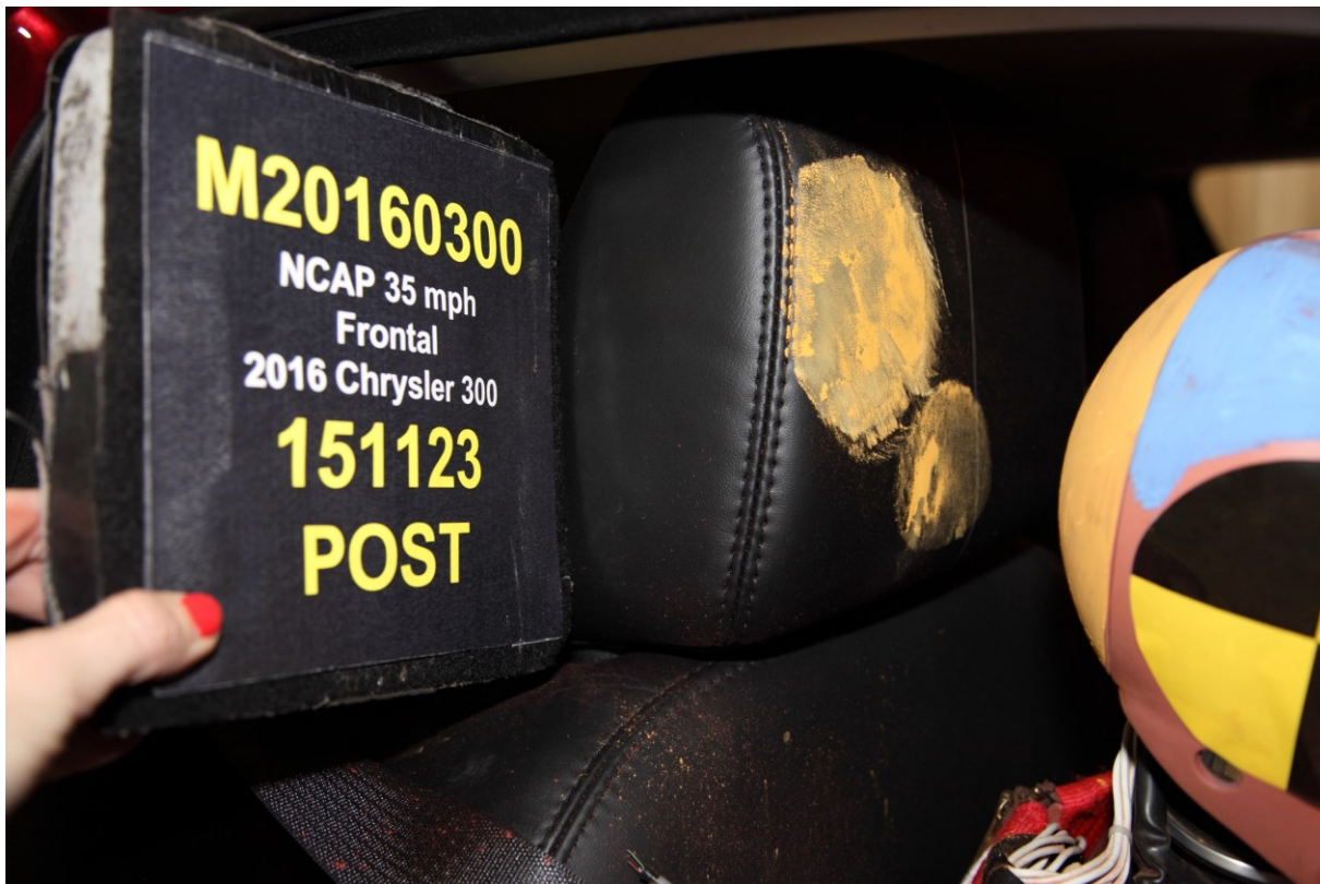
069 Post Test Passenger Dummy Contact With Headrest
