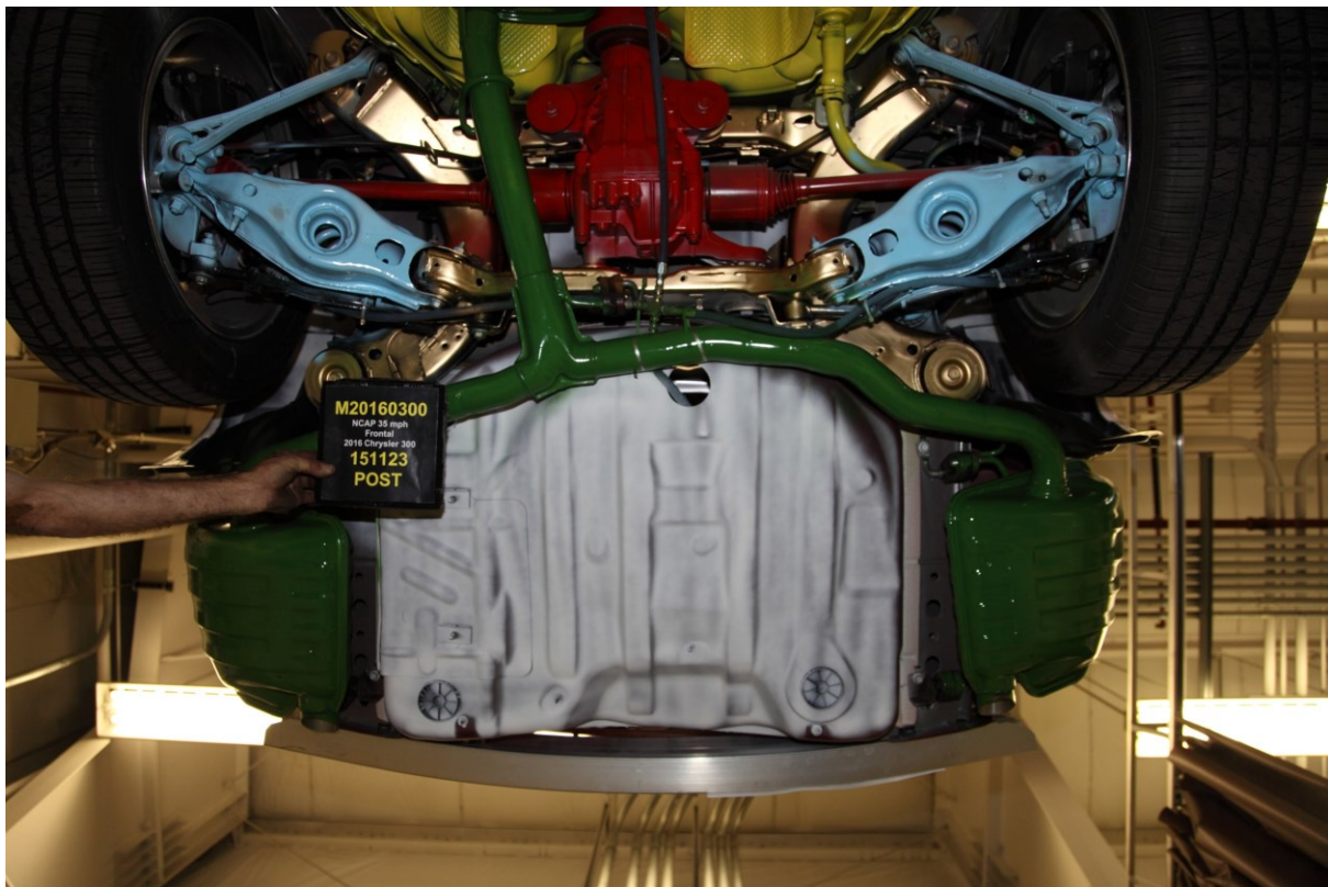
027 Post-Test Rear Underbody View
