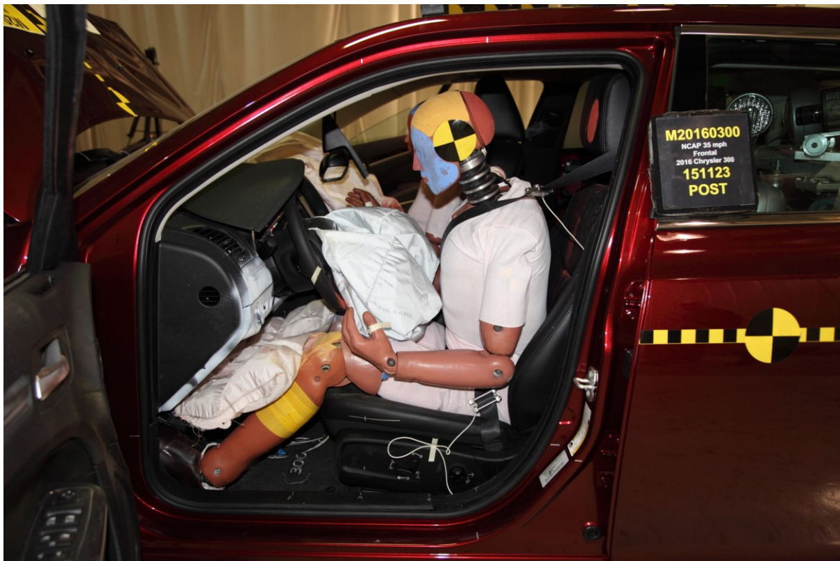
035 Post-Test Driver Dummy and Vehicle Interior View
