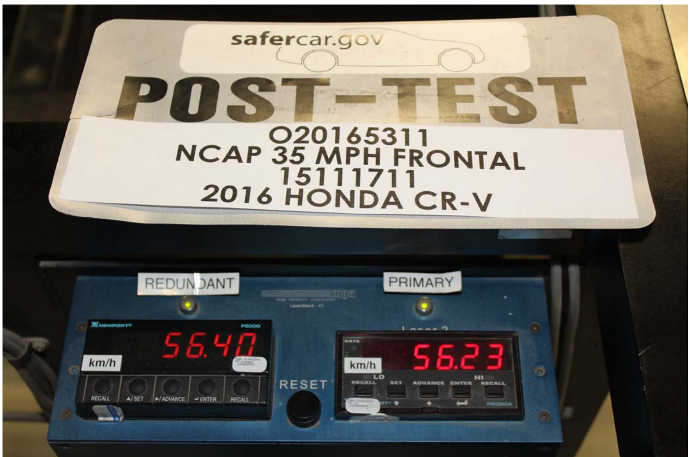
Photo No. 072 - Post-Test Speed Trap Read-Out
