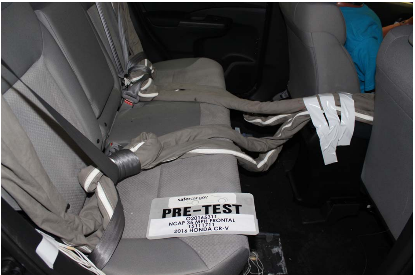
Photo No. 028 - Pre-Test Dummy Cable Routing
