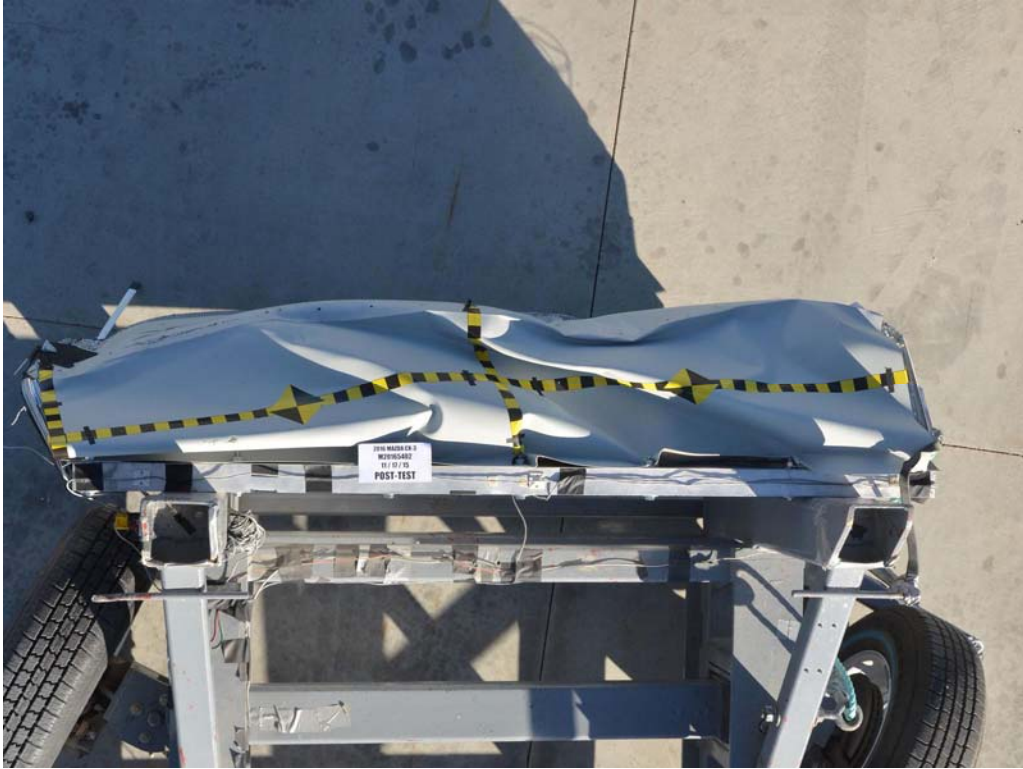
FIGURE 87. Post-Test Top View of MDB Impactor Face
