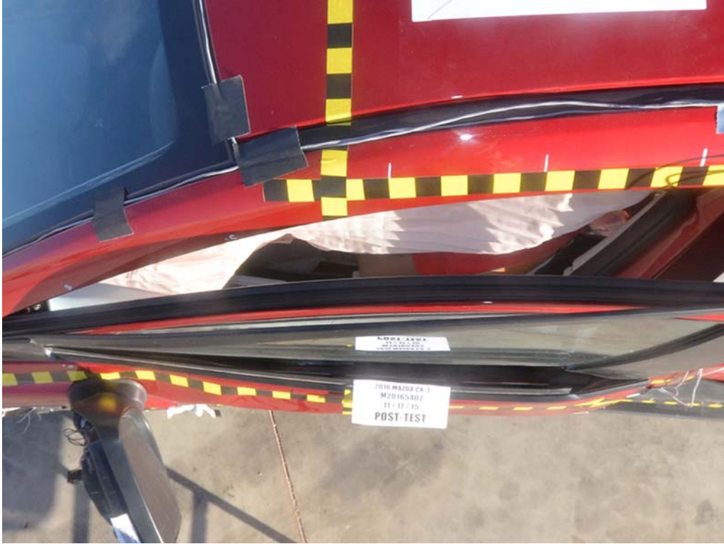
FIGURE 43. Post-Test Driver Dummy and Door Clearance View
