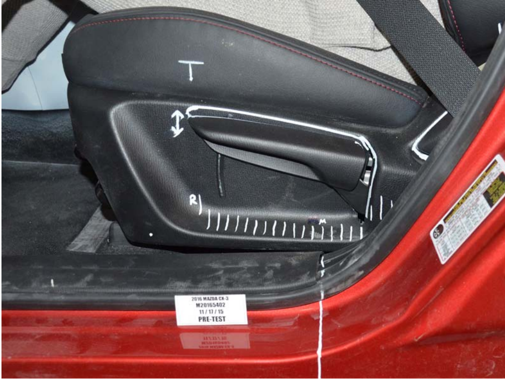
FIGURE 39. Pre-Test Close-Up Left Side View of Driver Seat Track
