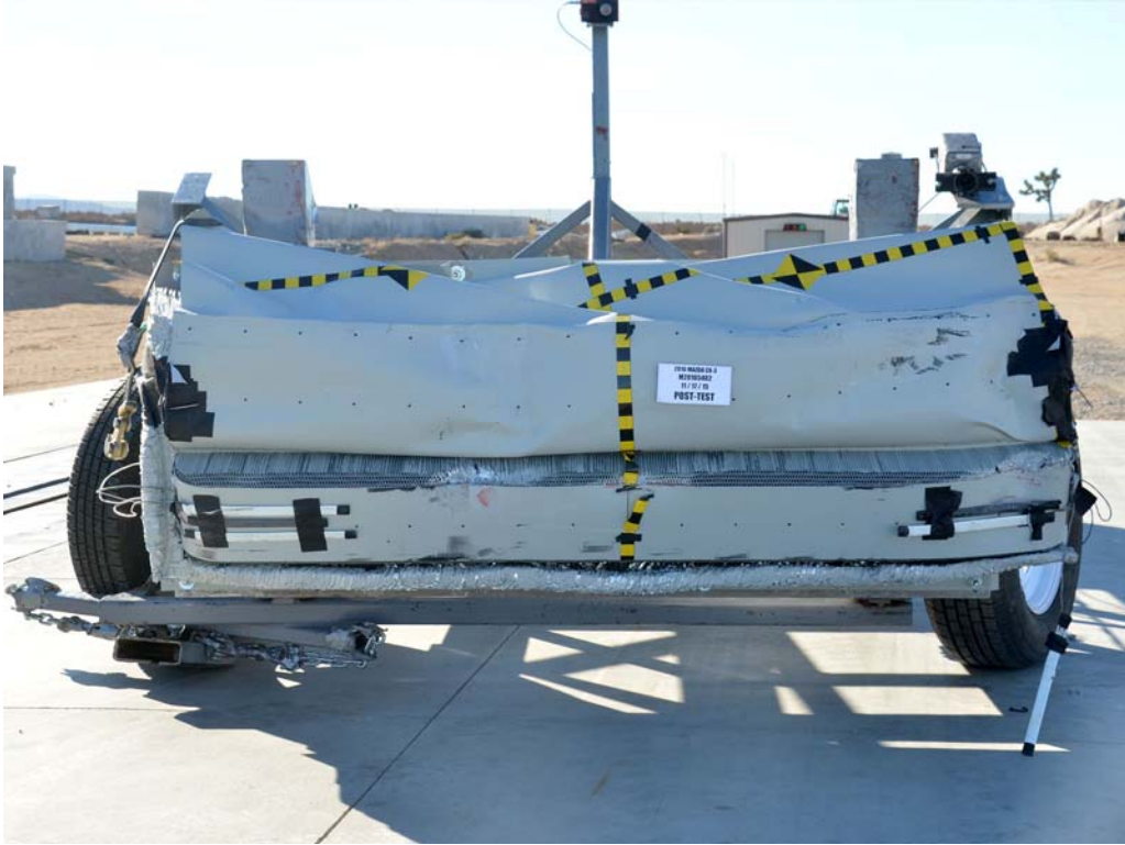
FIGURE 85. Post-Test Front View of MDB Impactor Face
