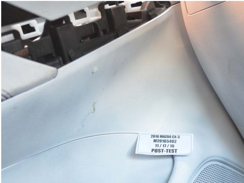
FIGURE 54. Post-Test Driver Dummy Close-Up Knee Contact View
