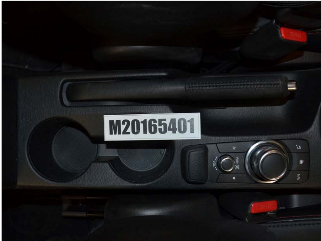
FIGURE 35. View of Disengaged Parking Brake
