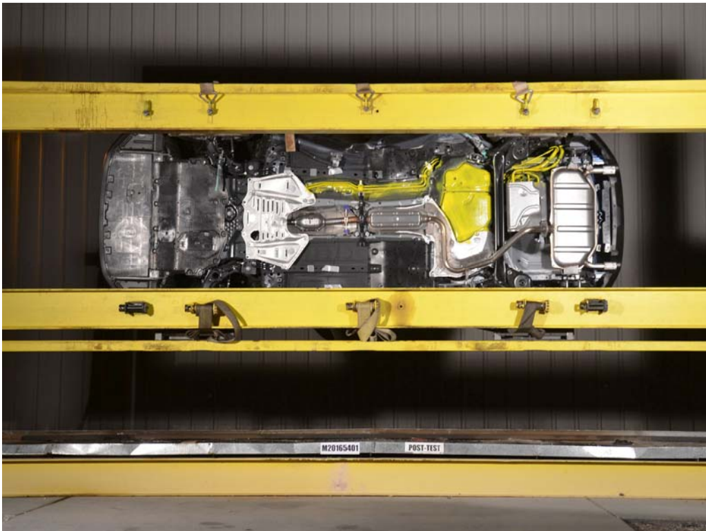
FIGURE 66. FMVSS No. 301 Static Rollover 270 Degrees
