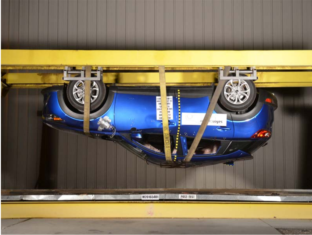
FIGURE 65. FMVSS No. 301 Static Rollover 180 Degrees
