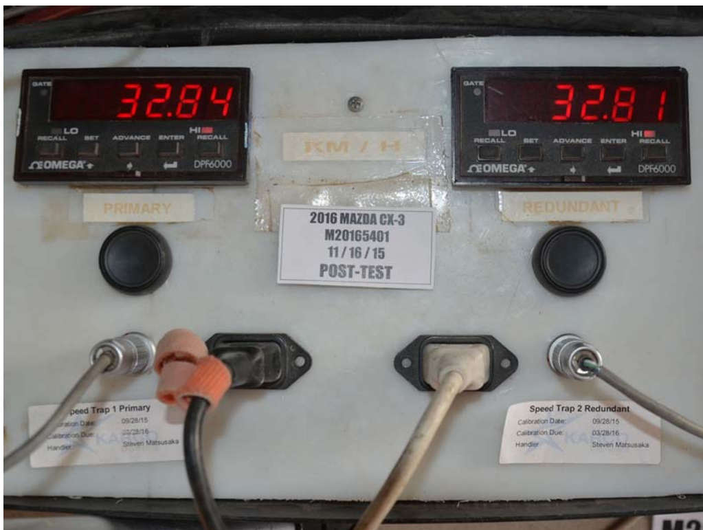
FIGURE 62. Post-Test Primary and Redundant Speed Trap Read-Out
