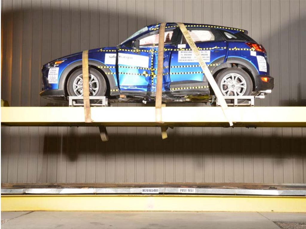
FIGURE 63. FMVSS No. 301 Static Rollover 0 Degrees
