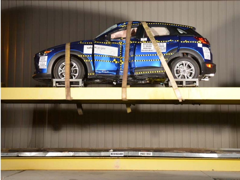
FIGURE 67. FMVSS No. 301 Static Rollover 360 Degrees
