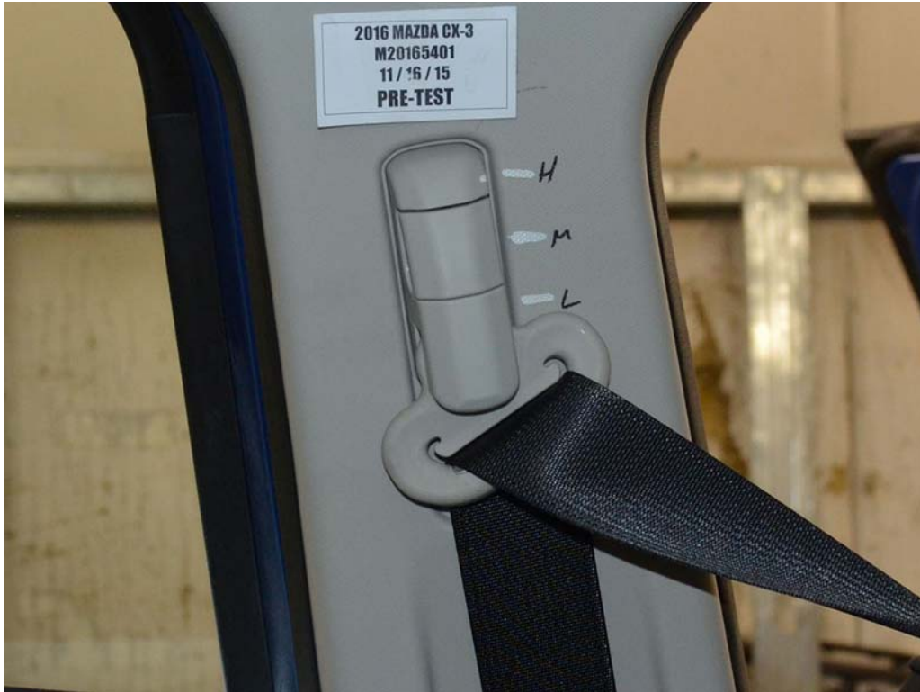
FIGURE 33. Pre-Test View of Belt Anchorage for Dummy
