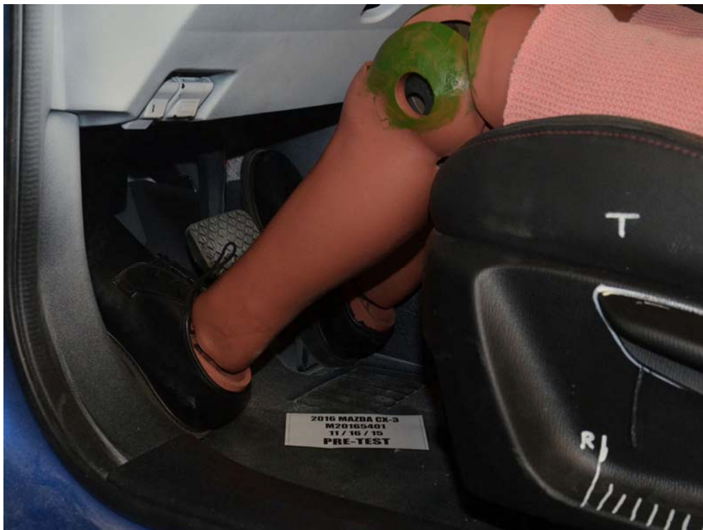
FIGURE 32. Pre-Test Placement of Dummy's Feet
