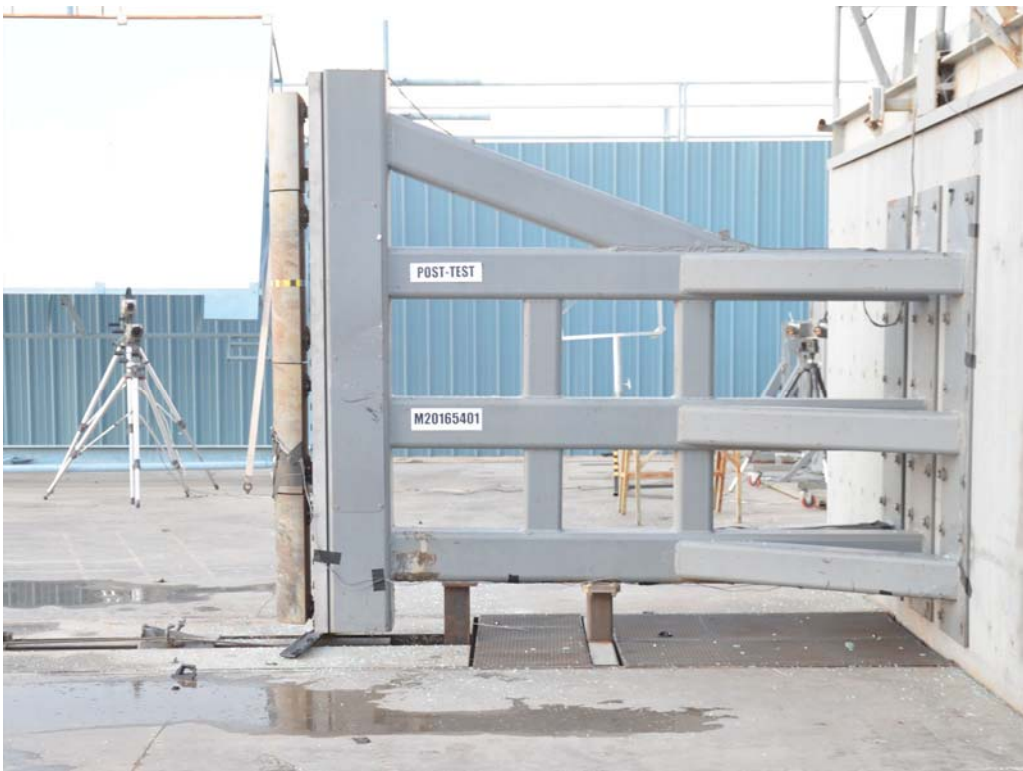
FIGURE 60. Post-Test Pole Barrier Side View
