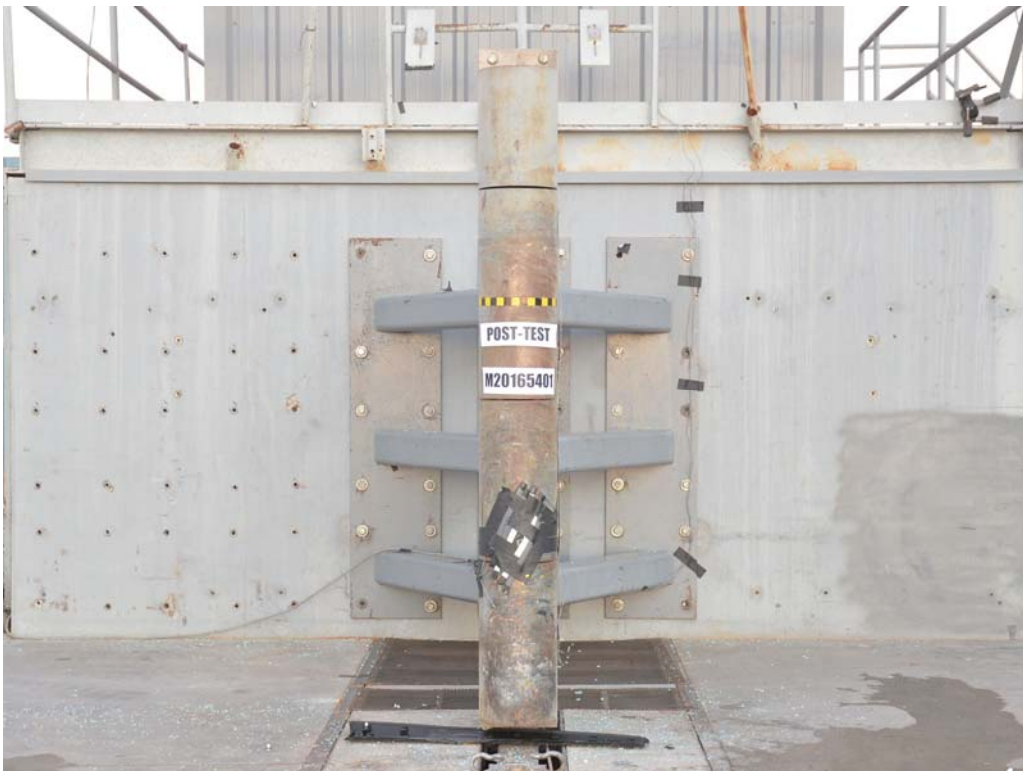
FIGURE 58. Post-Test Pole Barrier Front View
