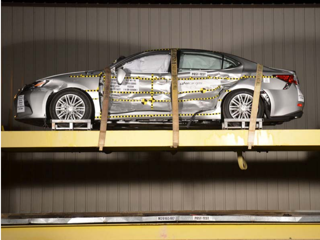
FIGURE 96. FMVSS No. 301 Static Rollover 0 Degrees
