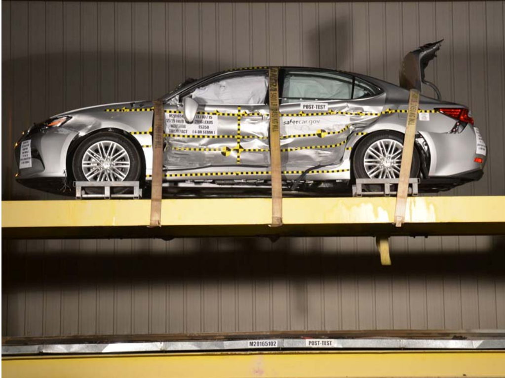
FIGURE 100. FMVSS No. 301 Static Rollover 360 Degrees
