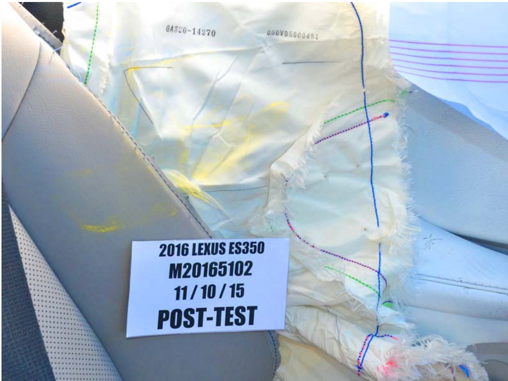
FIGURE 78. Post-Test Rear Passenger Dummy Close-Up Torso Contact with Side Airbag View
