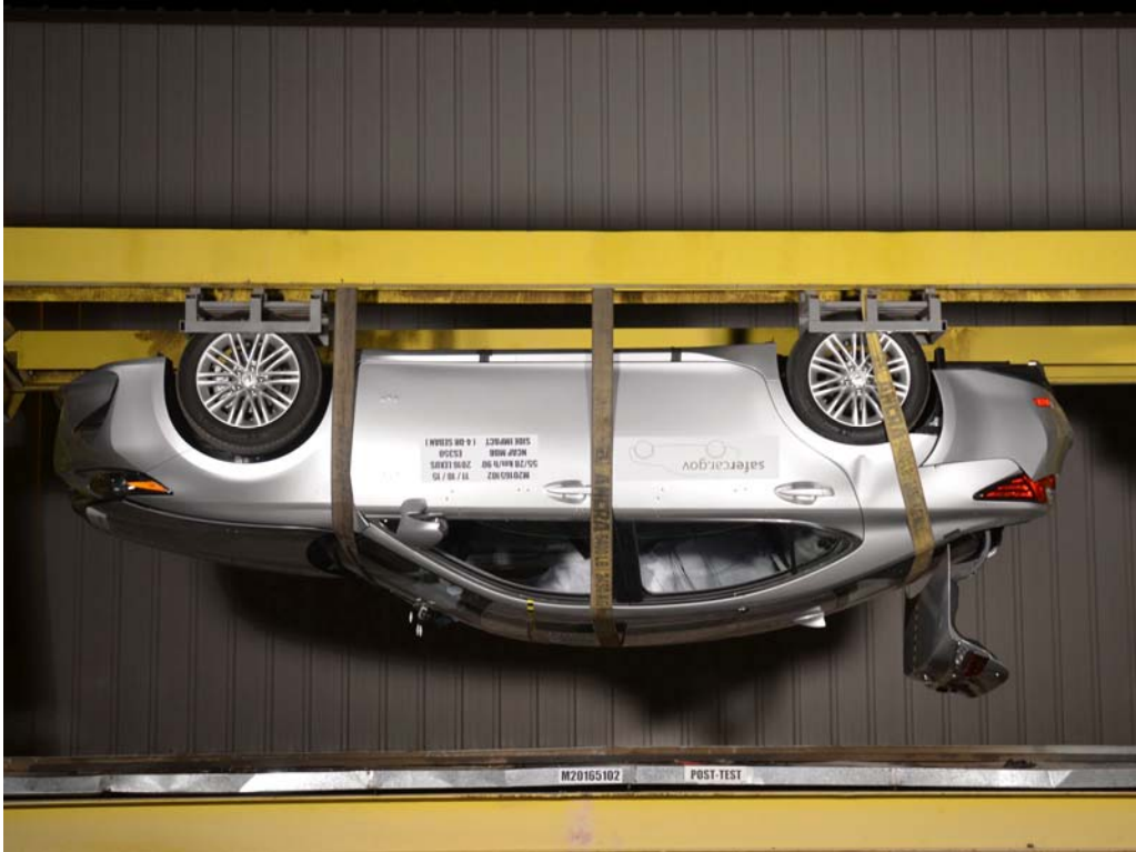
FIGURE 98. FMVSS No. 301 Static Rollover 180 Degrees
