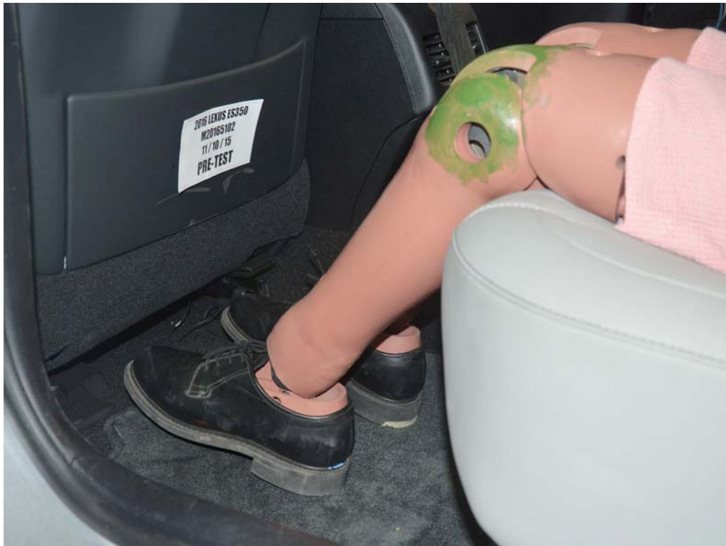
FIGURE 64. Pre-Test Placement of Rear Passenger Dummy's Feet
