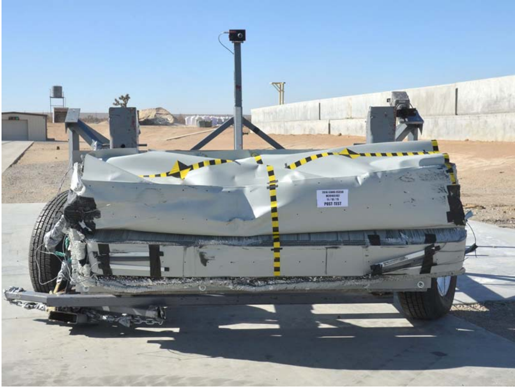
FIGURE 85. Post-Test Front View of MDB Impactor Face
